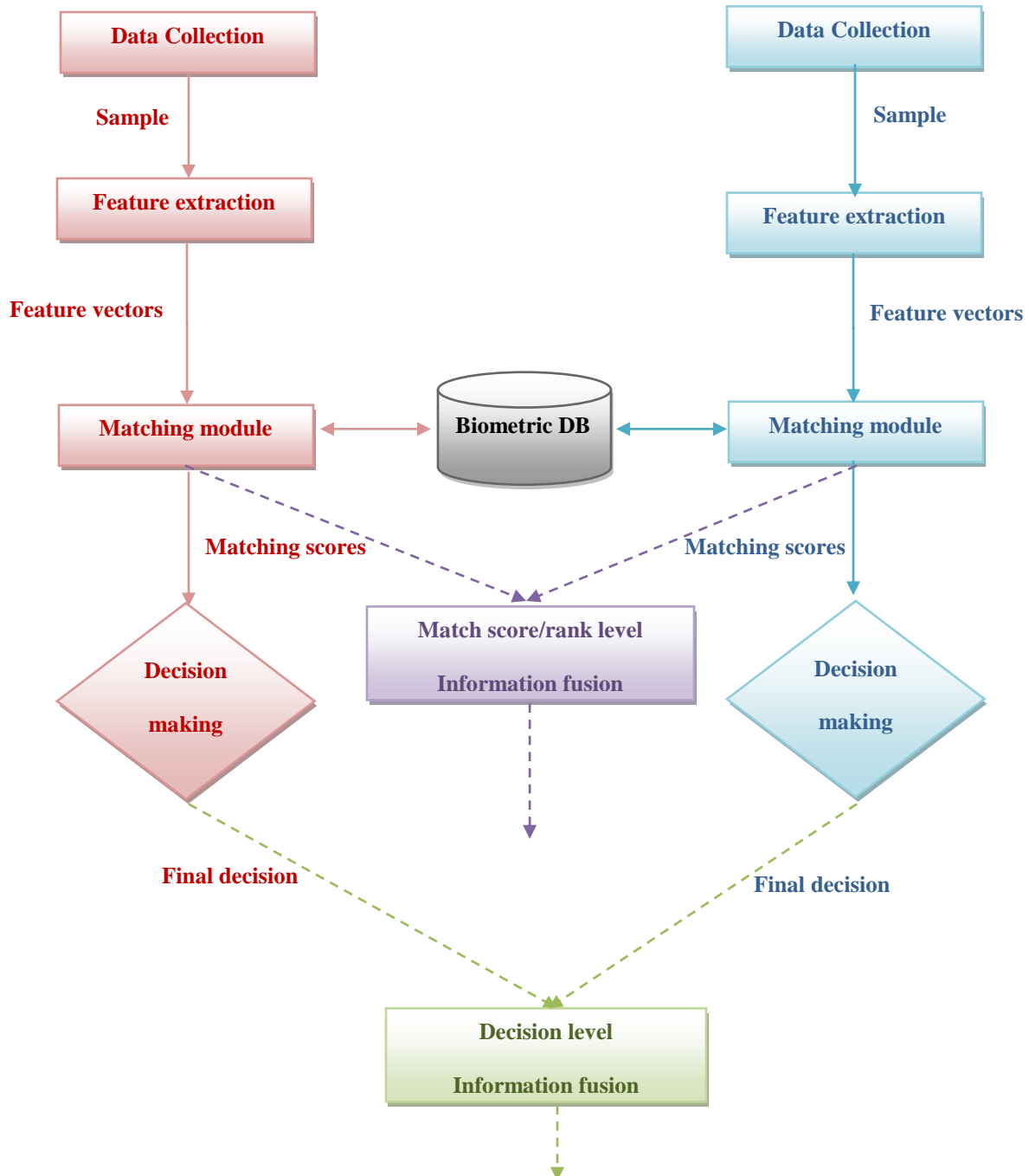
Figure 2-8: The general framework of an after matching multimodal biometric system (adapted from (11))
