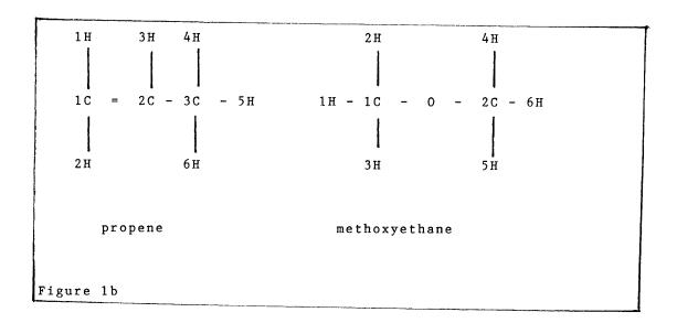
The occurrence numbers to the left of the atomic symbols in Figure 1b would likely be omitted in any display generated by a graphics system. The occurrence numbers are crucial for the storage of the structure of any molecule, no matter how large or complex. They are also used by IUPAC in chemical nomenclature. The two-path approach, which we present shortly, is to a considerable extent due to a need for synchronization of occurrence numbers with both data base and chemical methodology.
