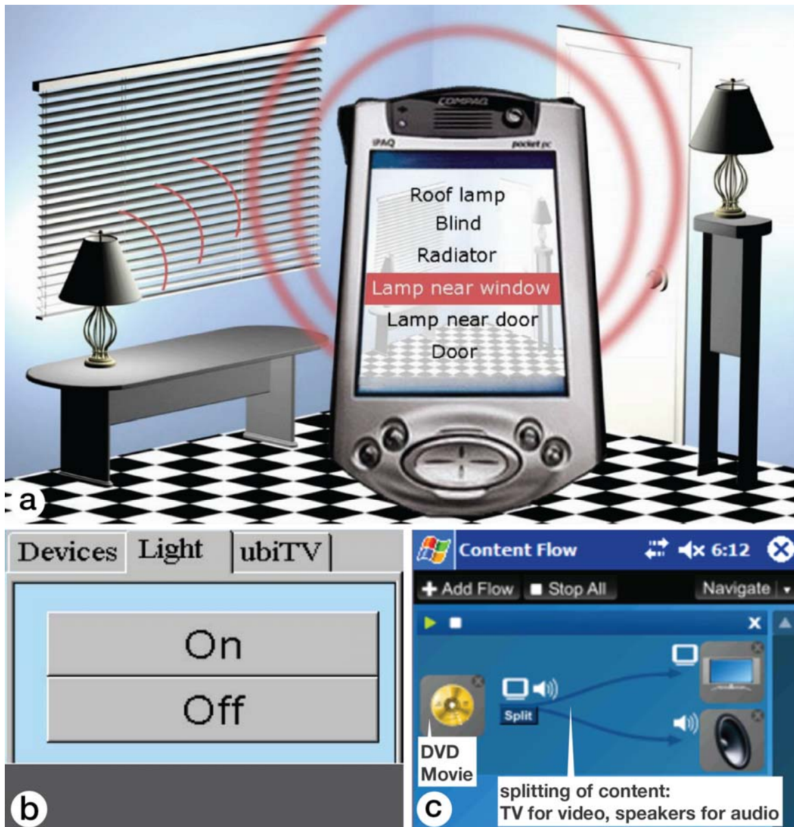
Figure 2.7. Scanning shows a list of connected devices. Here we can see (a) a list of devices from physical browsing research; (b) another interpretation by Yoon et al; and (c) Huddle, showing how users can select input and output devices for digital content. Reproduced from (Välkkynen & Tuomisto, 2005), (Yoon et al., 2007) and (Nichols et al., 2006) (annotated).
