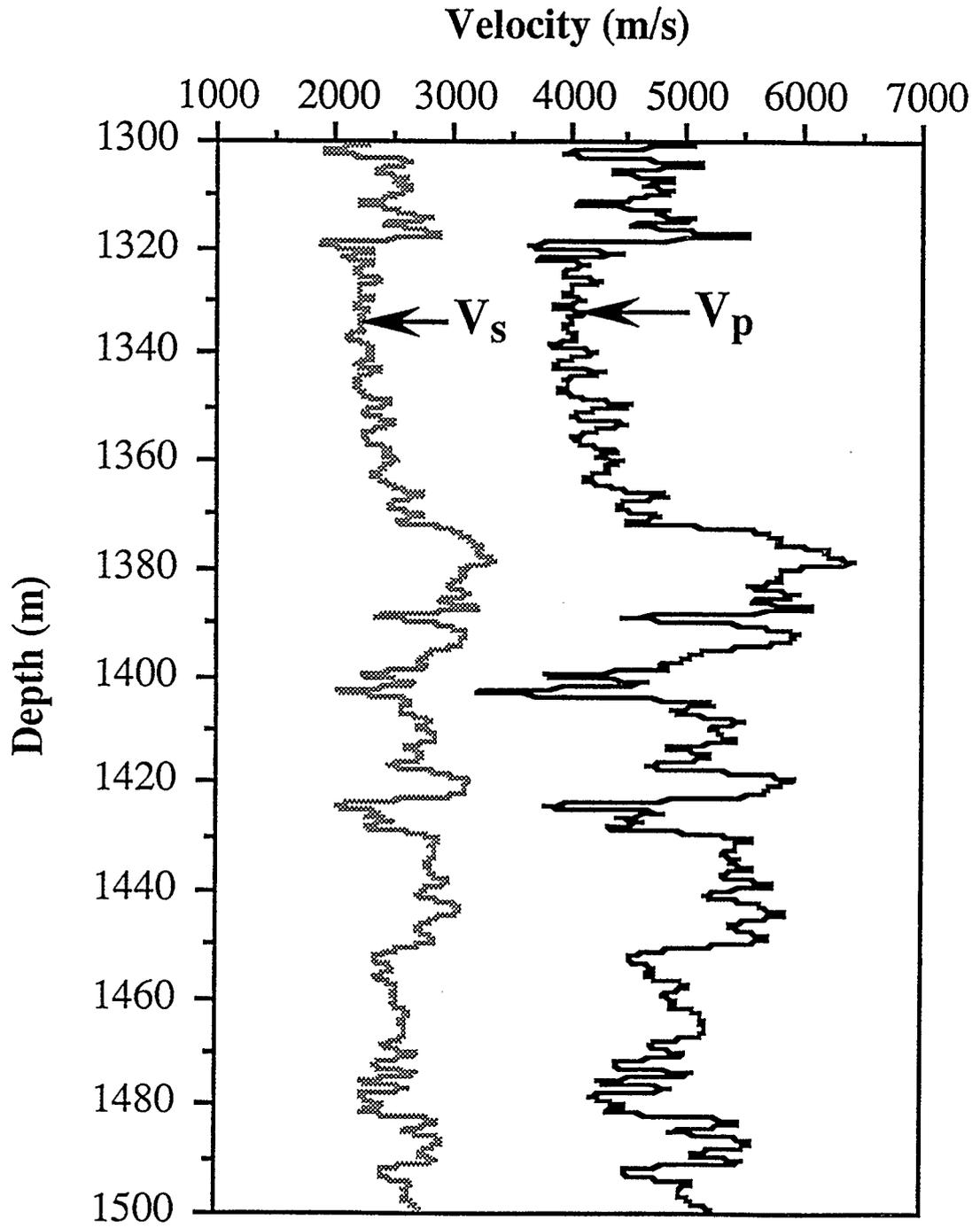
Figure 2.4: Interval velocity functions of the sonic logs.
