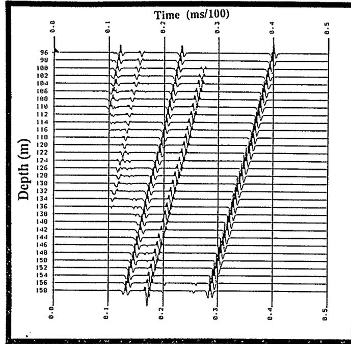
Figure 4.2: Median-filtered upgoing wavefield of synthetic shot record 2.
