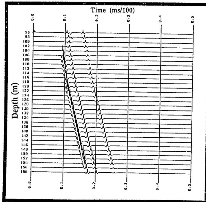
Figure 4.3: Median-filtered downgoing wavefield of synthetic shot record 2.
