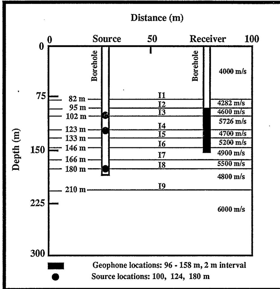
Figure 2.5: Depth model for generating synthetic data. Interface depths, P-wave layer velocities, and array geometry are displayed on the model.
