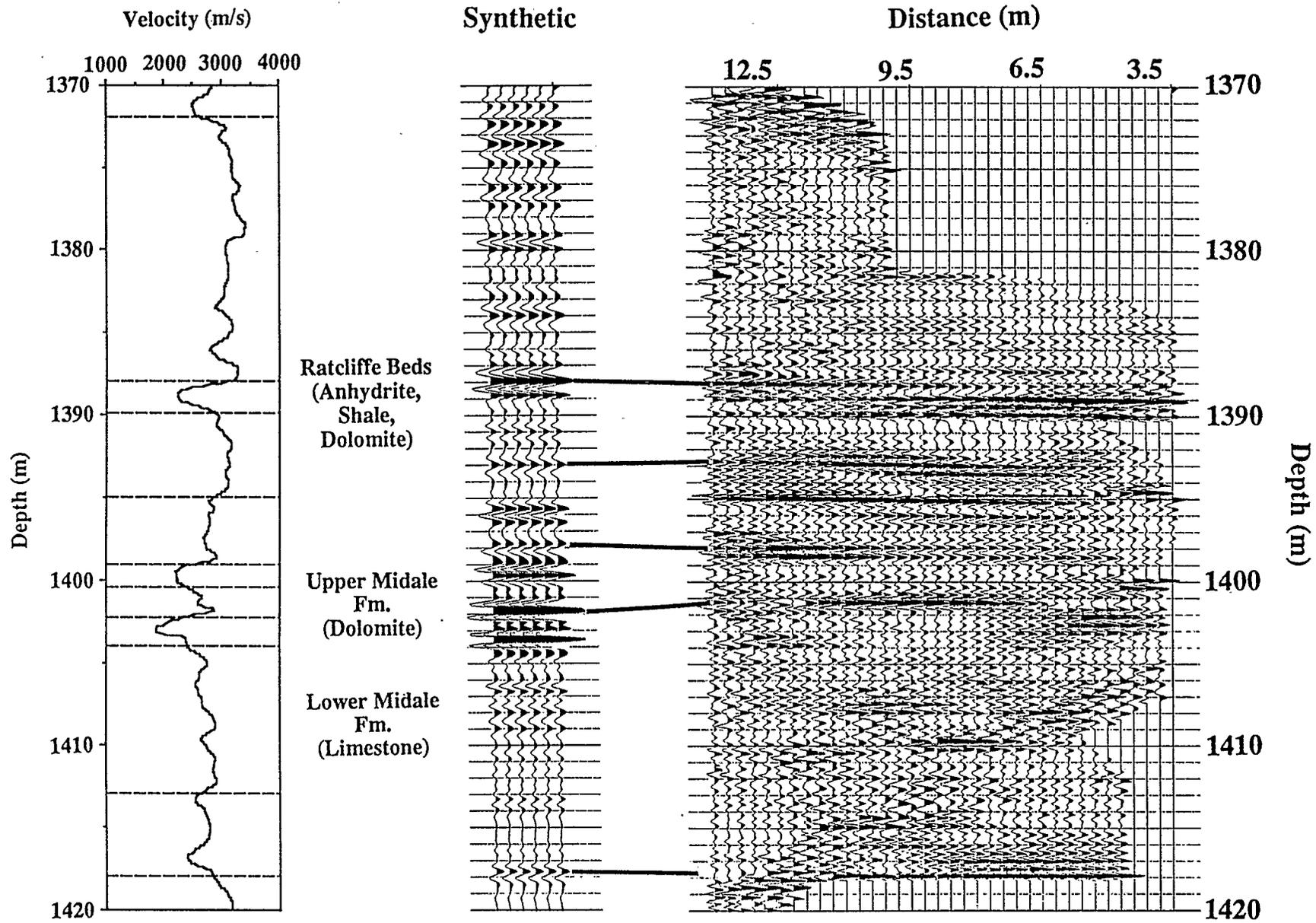
Figure 5.2: Correlation between the sum of all receiver-gather maps (right) and the synthetic seismogram in depth (middle) generated from the sonic log (left).
