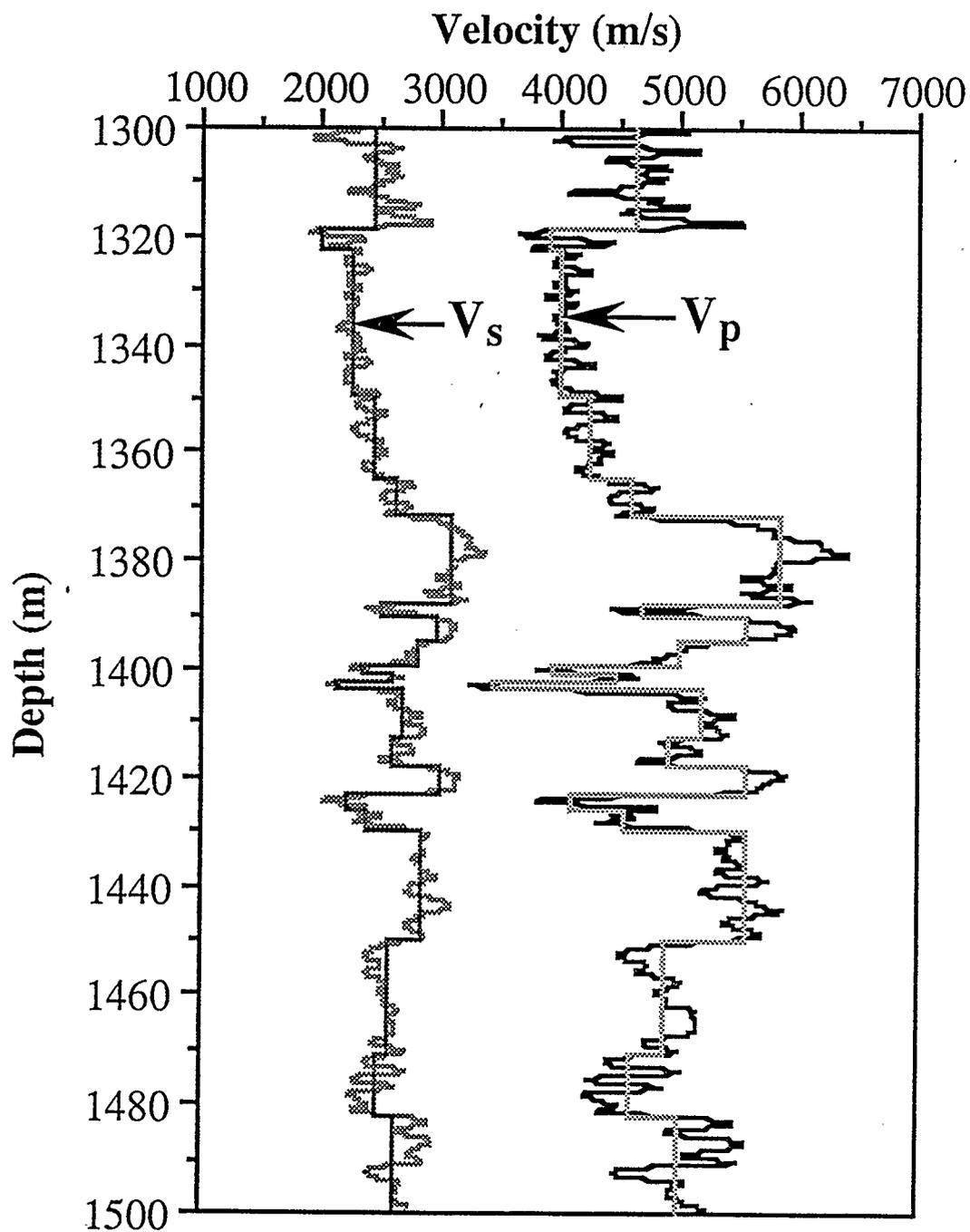
Figure 3.1: Blocked full-waveform velocity log of the Midale field data.
