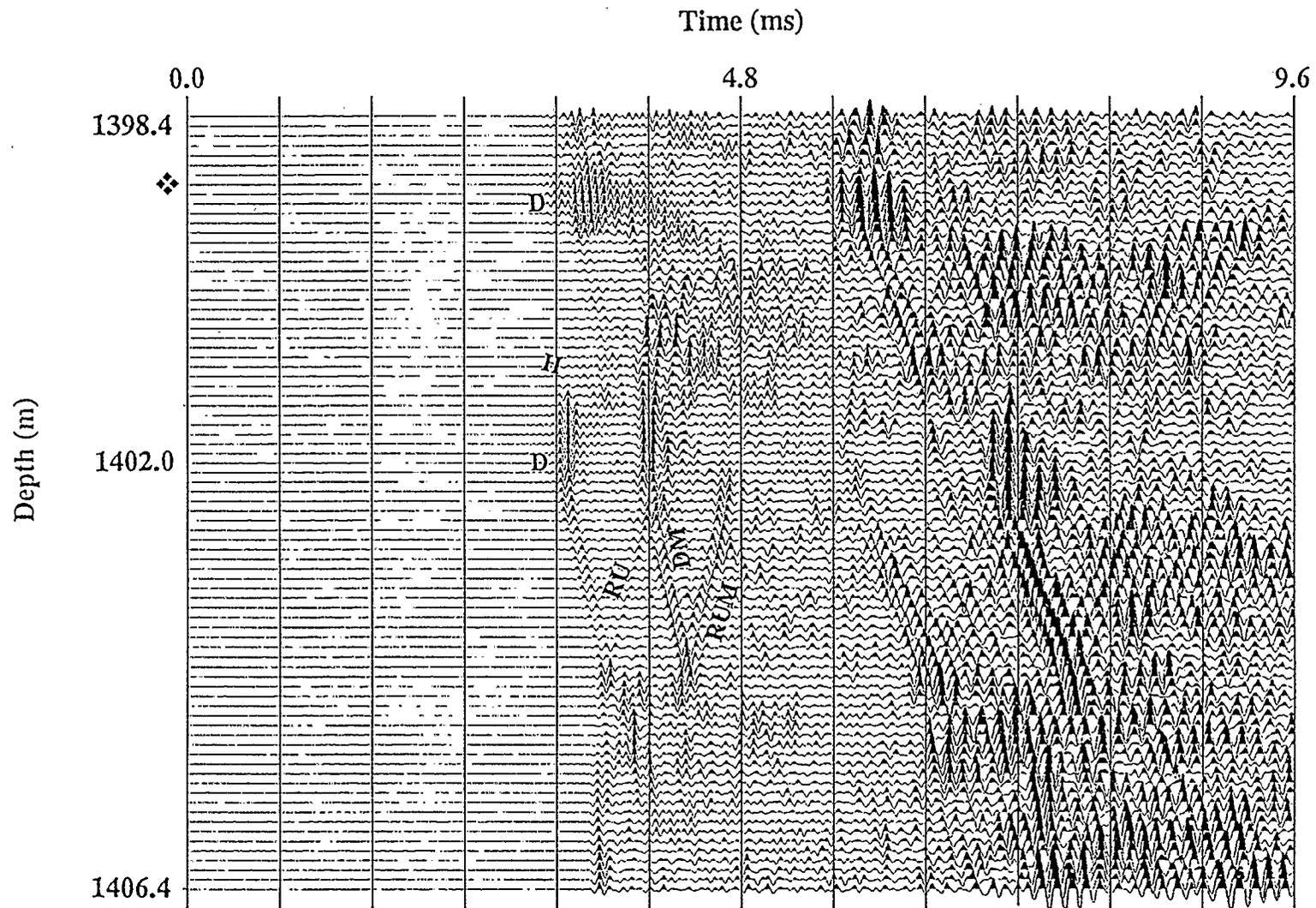
Figure 2.21: Source levels 1398.4 m to 1406.4 m of receiver 5 to show head waves, H, and peg-leg multiple events, DM and RUM. Receiver is at depth 1399 m.
