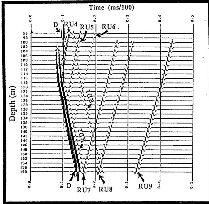
Figure 2.6: Synthetic shot record. Shot 1 at depth 100 m with geophone locations 96 to 158 m with 2 m interval (same set of geophones for every shot). Direct arrivals are labeled D, while reflected upgoing events are identified by RUI where I denotes the interface at which reflection occurred. Reflected downgoing events follow the same scheme.
