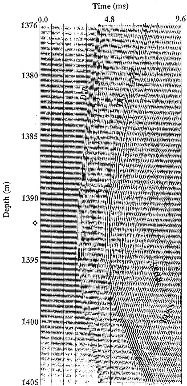
Figure 2.14: Band-pass receiver gather (no. 2) of the Midale field data. Annotated are D-P and D-S for direct P- and S-wave respectively, RUSS and RDSS for reflected upgoing and downgoing S waves.
