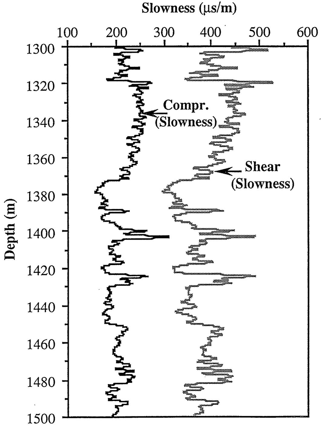
Figure 2.3: Full-waveform sonic log recorded in well FS-1.
