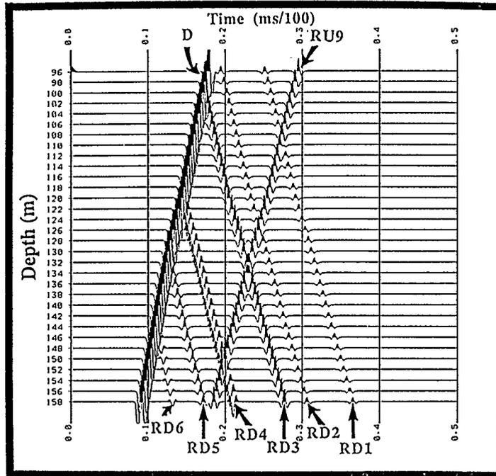
Figure 2.8: Synthetic shot record. Shot 3 at depth 180 m.
