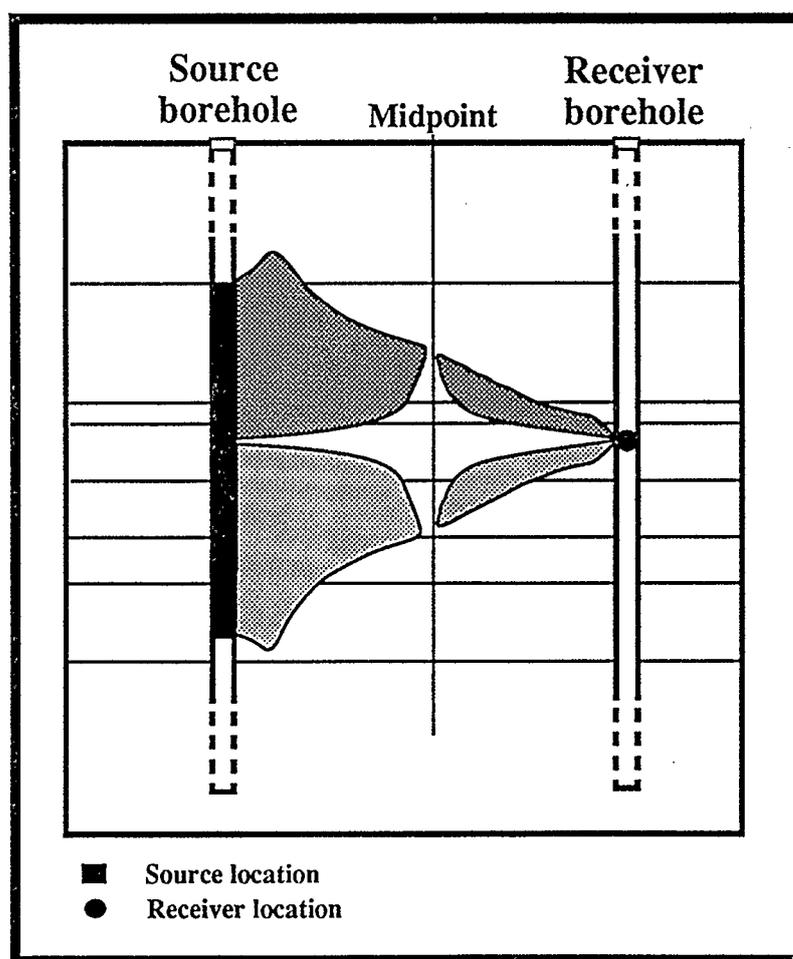
Figure 4.25: Subsurface coverage of receiver gather 2. Note the effect of limited recording time on the coverage.
