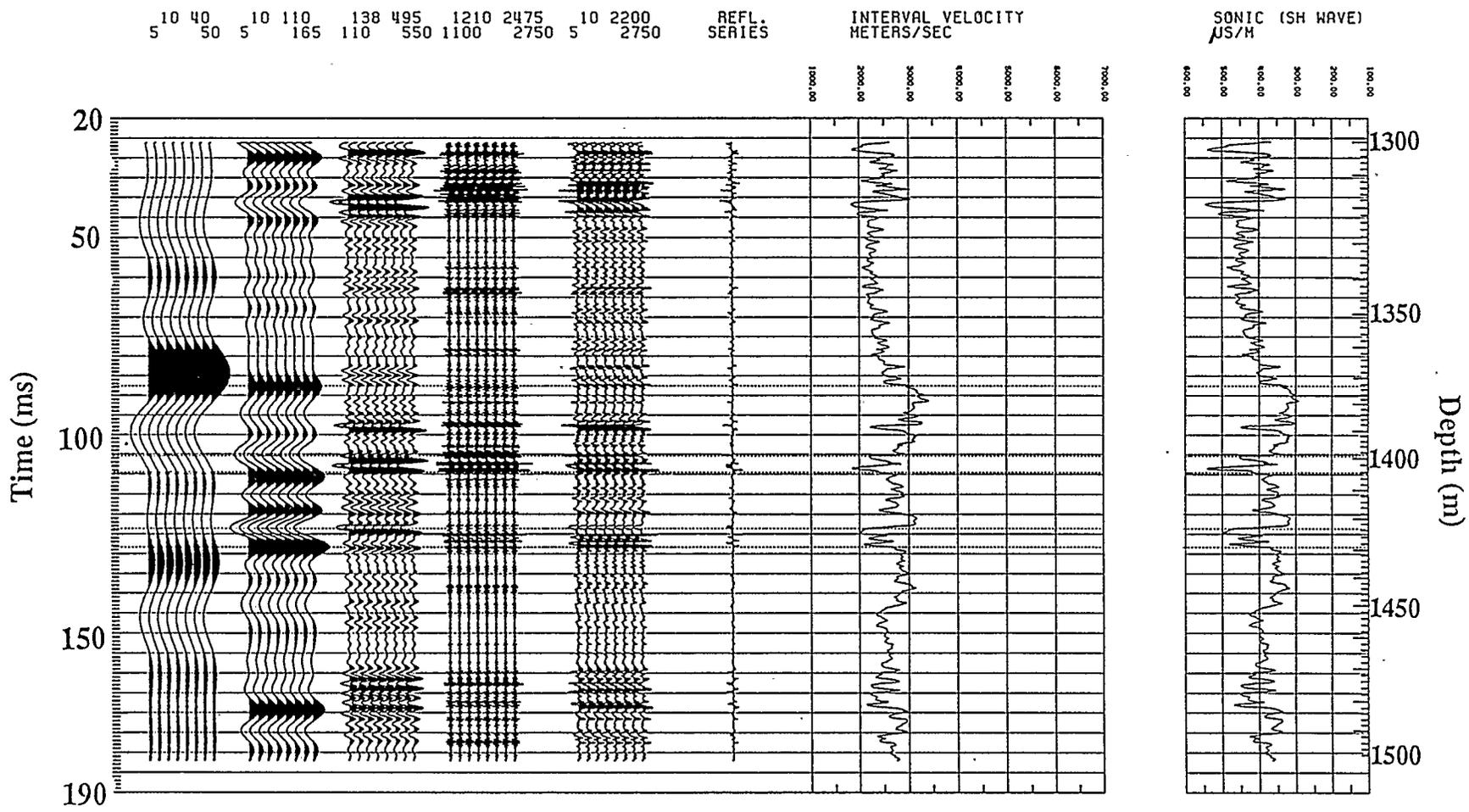
Figure 5.1: Synthetic seismograms generated from the shear sonic log from the source well (FS-1). The band limits used to generate the wavelet are annotated on the top of each group of synthetic seismograms.
