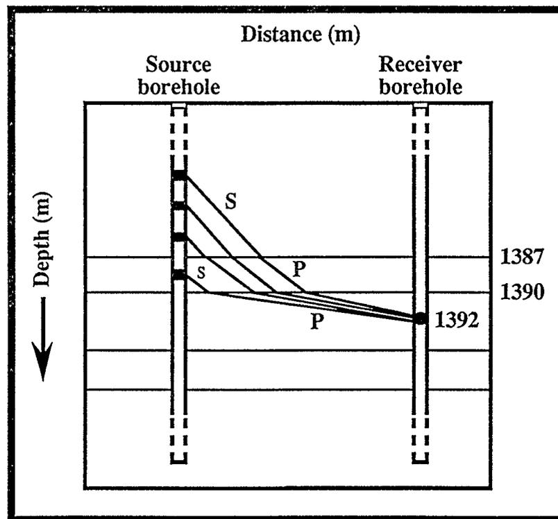
Figure 2.17: Geometry showing raypaths of transmitted-converted arrivals.
