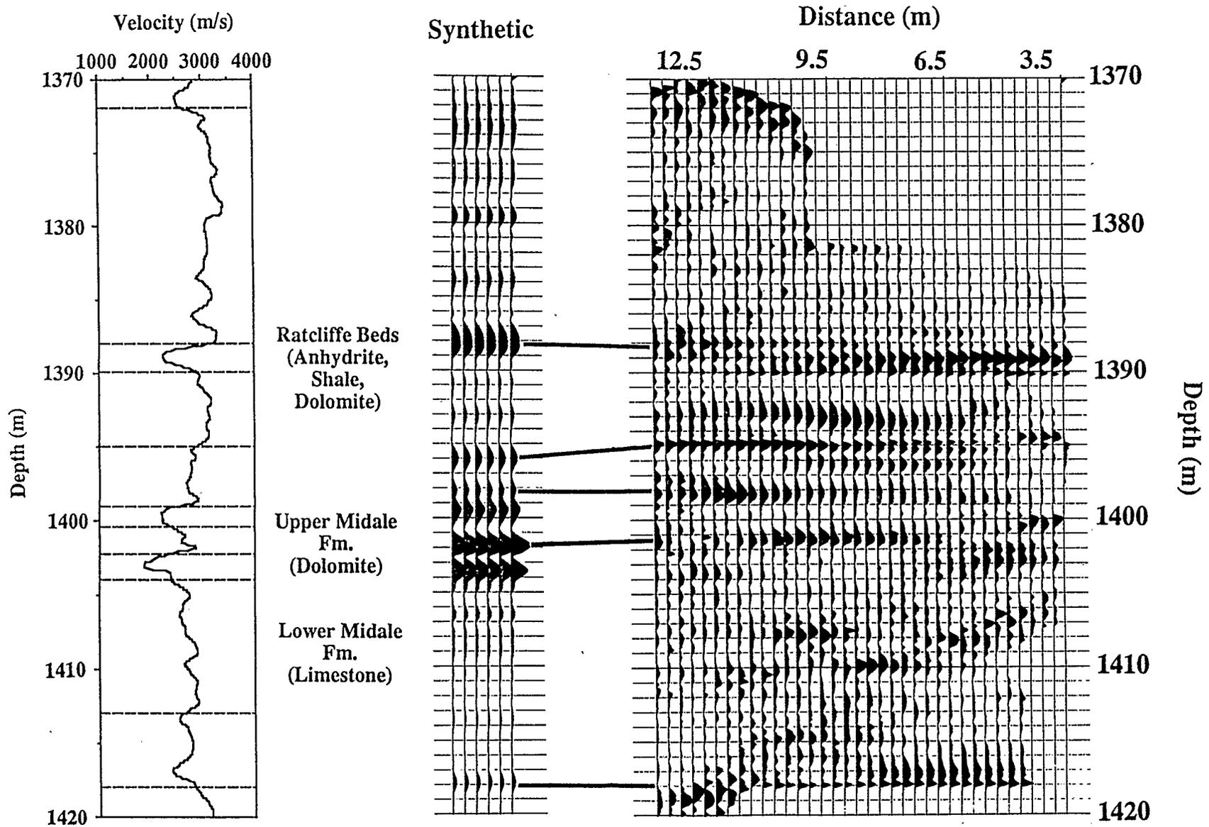
Figure 5.3: Correlation between the instantaneous amplitude of the sum (right) and the synthetic seismogram in depth (middle) generated from the sonic log (left).
