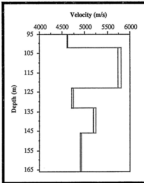
Figure 3.6: Inversion of synthetic data with a uniform error in all the picks. There is a consistent error in the estimated velocity function (dots) with respect to the true solution (solid).
