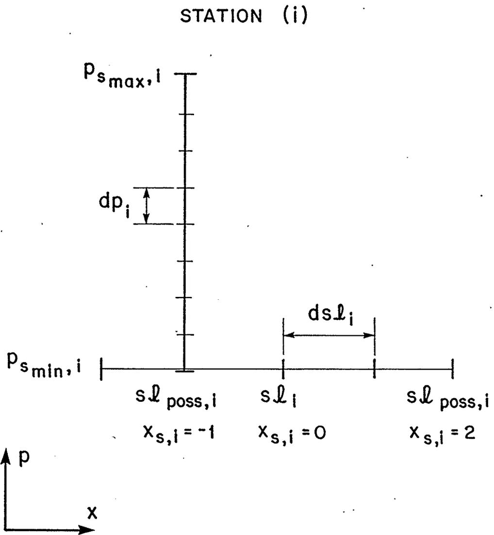
Figure 4.1 : Discretized Station Location and Pressure
