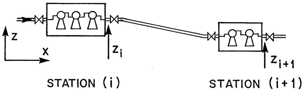
Figure 3.2 : Pressure Variation at the Booster Station (i) and in the Adjacent Pipe Segment
