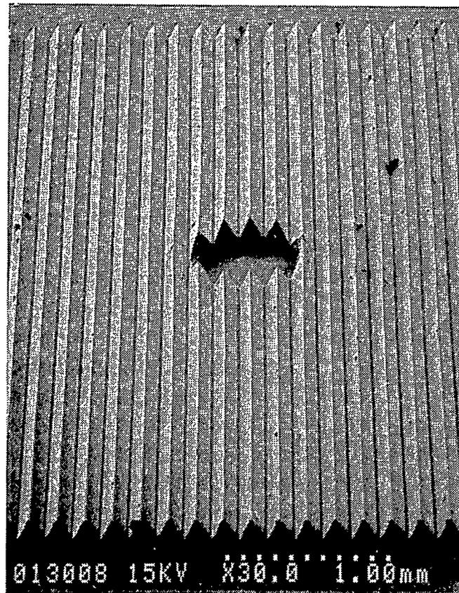
FIGURE 3.7. Typical cored pressure tap in a riblet sheet (large 3M triangular profile).
