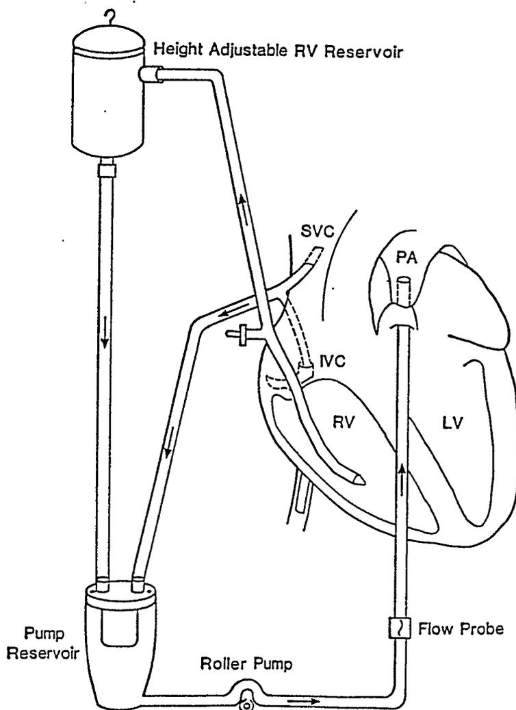
**Figure 4.1:** A Schematic Diagram Of The RV Bypass Model.
