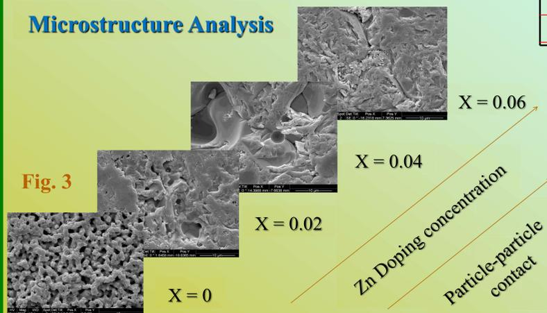
Fig. 3 shows the SEM images of as-prepared  $SrZn_{0.33+x}Nb_{0.67-x}O_{3-\delta}$  for  $x = 0, 0.02, 0.04$  and  $0.06$ .
