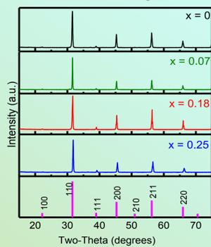
Figure 1 shows the PXRD patterns of  $SrZn_{0.33+x}Nb_{0.67-x}O_{3-\delta}$ , which could be indexed on a simple cubic ( $\sim 4 \text{ \AA}$ ) perovskite structure.
