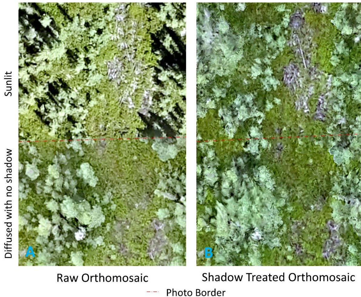
Figure 8: A comparison of performance between the raw orthomosaic and the shadow-treated orthomosaic, when data is collected under varying light conditions. The shadow-treated orthomosaic (right) displays better radiometric matching than the raw orthomosaic (left).
