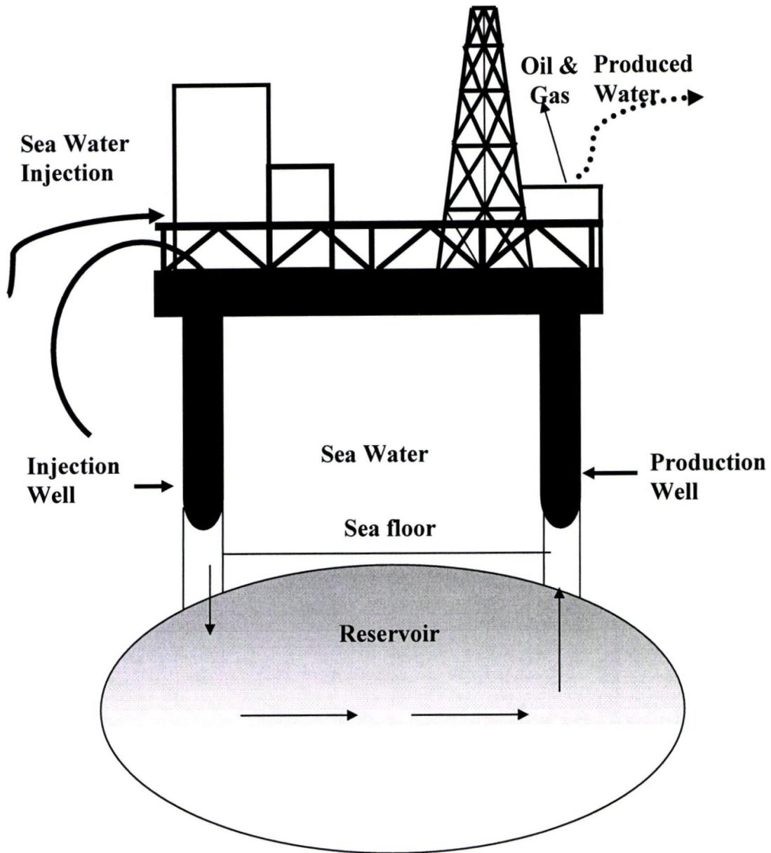
**Figure 1.1** Secondary oil production. Seawater is injected into the reservoir to maintain pressure and mixes with the oil. The oil is separated from the produced water, which is cleaned and dumped back into the sea.
