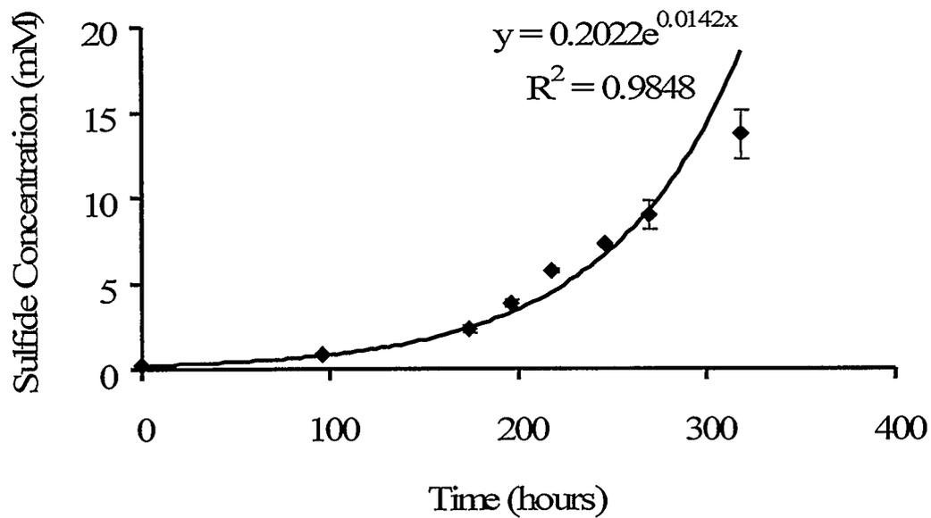
**Figure 3.5** NS-tSRB-2 during exponential growth phase in MS-20-L when incubated at 60 °C and using a 5 % inoculum. Each point is the average of two trials with the error bars representing the standard deviation between the two points. A best fit of the data (Sulfide Concentration vs Time) is shown.
