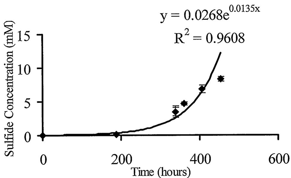
**Figure 3.1** NS-tSRB-1 during exponential growth phase in MS-2-20-OA when incubated at 60 °C and using a 5 % inoculum. Each point is the average of two trials with the error bars representing the standard deviation between the two points. A best fit of the data (Sulfide Concentration vs Time) is shown.
