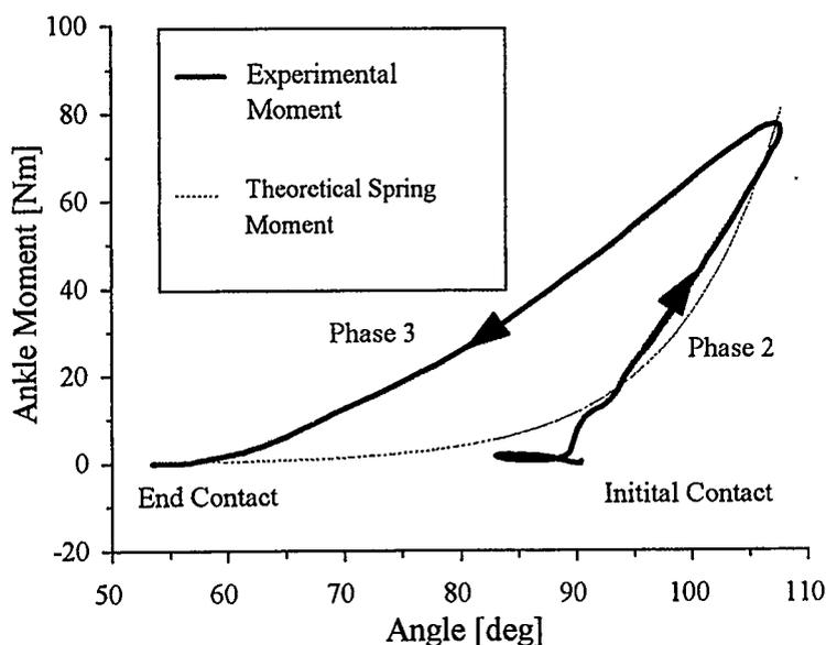
Figure 3.8: Ankle Moment Versus Angular Position of the Foot. The Experimental Moment is Shown by a Solid Line and the Theoretical Spring Moment is Shown by the Dotted Line. The Shaded Portion Represents the Energy the Spring is Unable to Provide to the System (the Quantity of the Auxiliary Moment).
