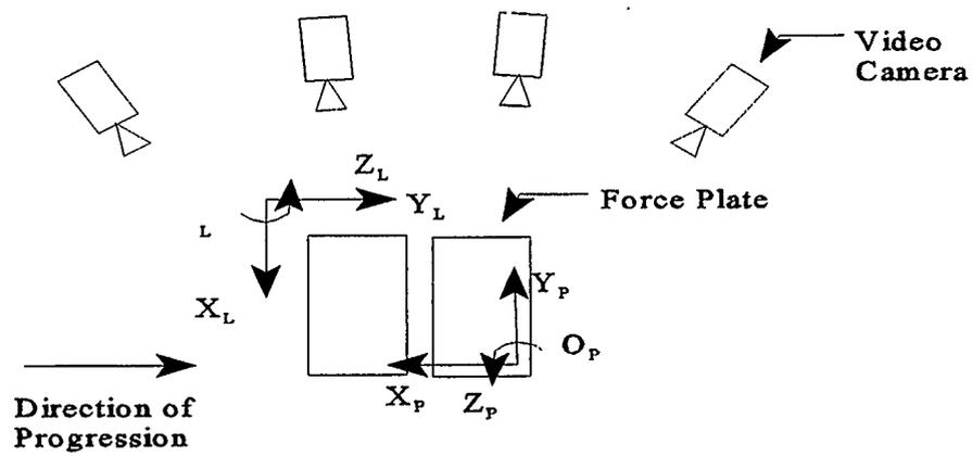
Figure 3.1: Schematic of laboratory setup,  $O_L$  is the origin of the laboratory coordinate system. The origin of the plate coordinate system was centered on the force plate with  $X_P$  running opposite  $Y_L$ , and  $Y_P$  running opposite of  $X_L$ . The axis in the laboratory coordinate system ( $Z_L$ ) points up and  $Z_P$  points down.
