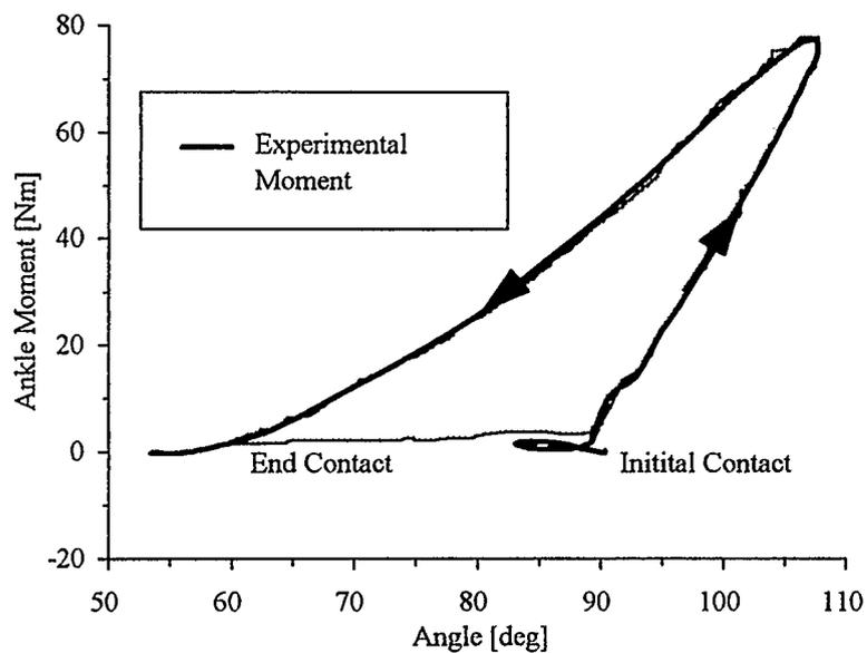
Figure 3.6: Experimental Ankle Moment Versus Angular Position of the Foot
