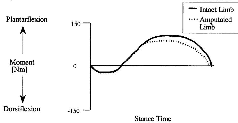
Figure 2.9: Resultant Ankle Joint Moment-Time Histories During Stance for an Individual with a BKA Running at Speed Averaging 2.6 m/s (Miller, 1987).
