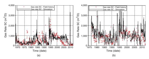
Fig. 7—History-matched gas production rates of two vertical wells. (a) Simulated gas rate of Well 1. (b) Simulated gas rate of Well 2.
