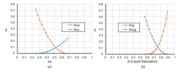
Fig. 4—Relative permeability curves. (a) Oil and water relative permeability curve and (b) liquid and gas relative permeability curve.
