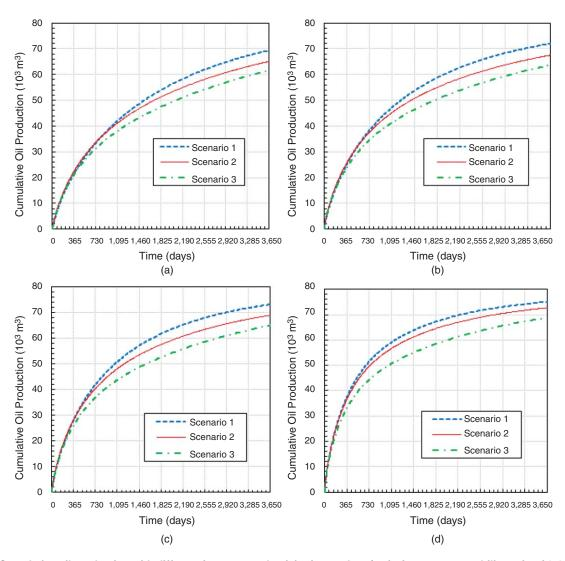
Fig. 15—Cumulative oil production with different fracture conductivity (secondary-/main-fracture permeability ratio of 1:4 and conductivity ratio of 1:8). (a) Fracture conductivity of 100 darcy mm. (b) Fracture conductivity of 150 darcy mm. (c) Fracture conductivity of 200 darcy mm. (d) Fracture conductivity of 500 darcy mm.
