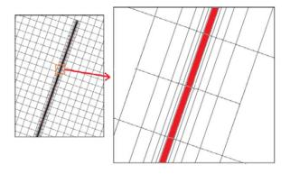
Fig. 5—Magnified picture on local refined grids at and near the hydraulic fracture.
