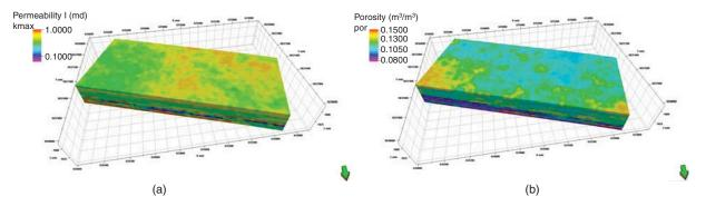
Fig. 3—Properties of geological model. (a) Matrix permeability of geological model. (b) Matrix porosity of geological model.
