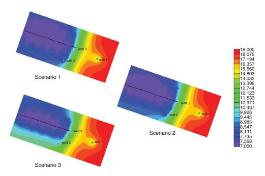
Fig. 16—Pressure distribution after 10 years (main-fracture conductivity is 500 darcy·mm; secondary-/main-fracture permeability ratio is 1:4; and conductivity ratio is 1:8).
