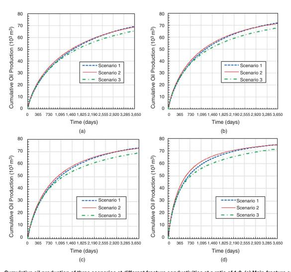
Fig. 17—Cumulative oil production of three scenarios at different fracture conductivities at a ratio of 1:2. (a) Main-fracture conductivity of 100 darcy mm. (b) Main fracture conductivity of 150 darcy mm. (c) Main-fracture conductivity of 200 darcy mm. (d) Main-fracture conductivity of 500 darcy mm.
