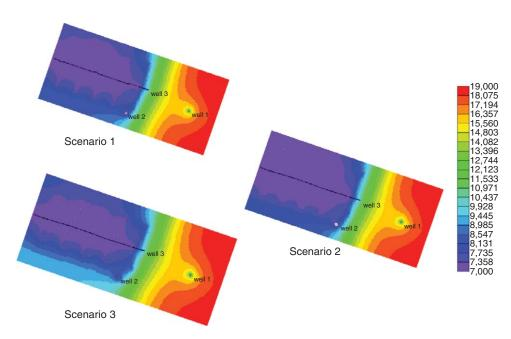
Fig. 18—Pressure distribution after 10 years at 500 darcy mm and a ratio of 1:2.
