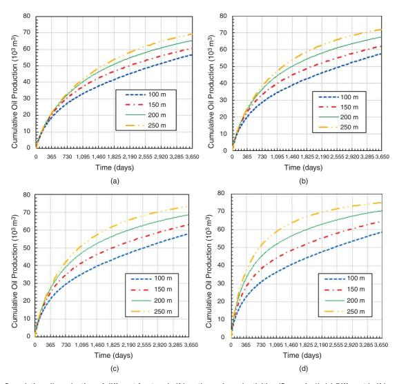
Fig. 14—Cumulative oil production of different fracture half-lengths and conductivities (Scenario 1). (a) Different half-lengths and fracture conductivity at 100 darcy·mm. (b) Different half-lengths and fracture conductivity 150 at darcy·mm. (c) Different half-lengths and fracture conductivity at 200 darcy·mm. (d) Different half-lengths and fracture conductivity at 500 darcy·mm.
