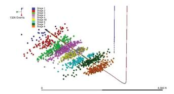
Fig. 8—Different stages of the microseismic-event view of a horizontal well.
