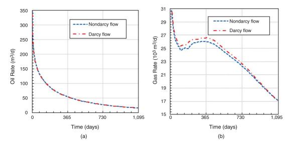
Fig. 13—Comparison of Darcy flow and non-Darcy flow in main fractures with conductivity of 500 darcy mm. (a) Comparison of Darcy flow and non-Darcy flow for oil phase. (b) Comparison of Darcy flow and non-Darcy flow for gas phase.
