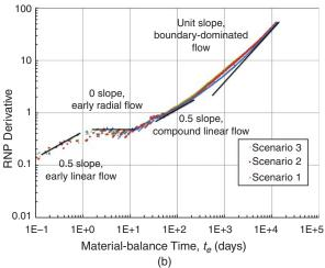
Fig. 19—Rate-normalized pressure (RNP) and its derivative signature for the horizontal well with multiple stage fractures. (a) RNP derivative signature for biwing fracture (Scenario 1). (b) RNP derivative signature for three scenarios (fracture conductivity of 500 darcy·mm).
