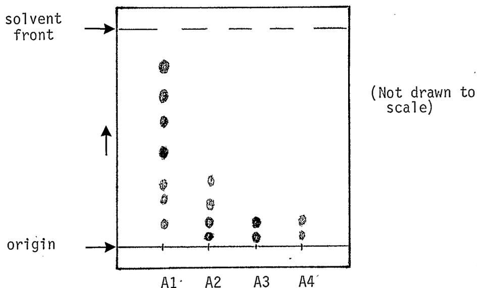
Figure 6: TLC Analysis of the pH-gradient-fractionated Alkaloids.
