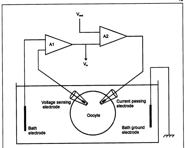
**Figure 1-3.** Conventional Two-Electrode Voltage Clamp. The difference in potential between the bath and voltage sensing electrodes  $(V_m)$  becomes the output of the A1 amplifier.  $V_m$  is compared to the command potential,  $V_{cmd}$ , by the A2 amplifier which passes current into the oocyte in order to minimize the difference between  $V_m$  and  $V_{cmd}$ .
