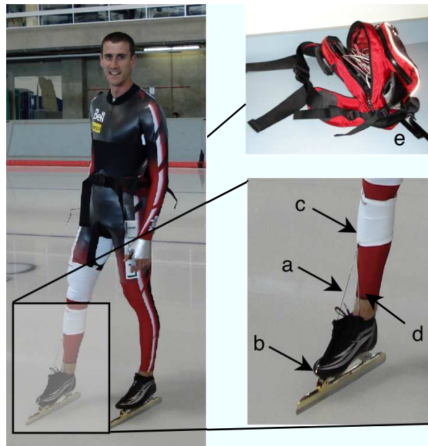
Figure 4.3: The sensor installed on the model skater: The variable-resistance elastic (a) is connected between a skate lace near the toe (b) and an elastic joint-support band (c) (used only to fasten the sensor). In this configuration, R_s (and therefore the voltage measured by the interface kit) increases with plantar flexion. Leads (d) connect the sensor to the phidget interface kit ( http://www.phidgets.com ) and netbook computer worn by the skater in a waist pack (e). Sound is broadcast using headphones (not shown).
