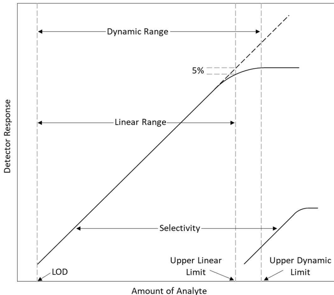
Figure 1-2: A depiction of a generic calibration curve of a detector illustrating selectivity, linear and dynamic ranges, and limit of detection (LOD).
