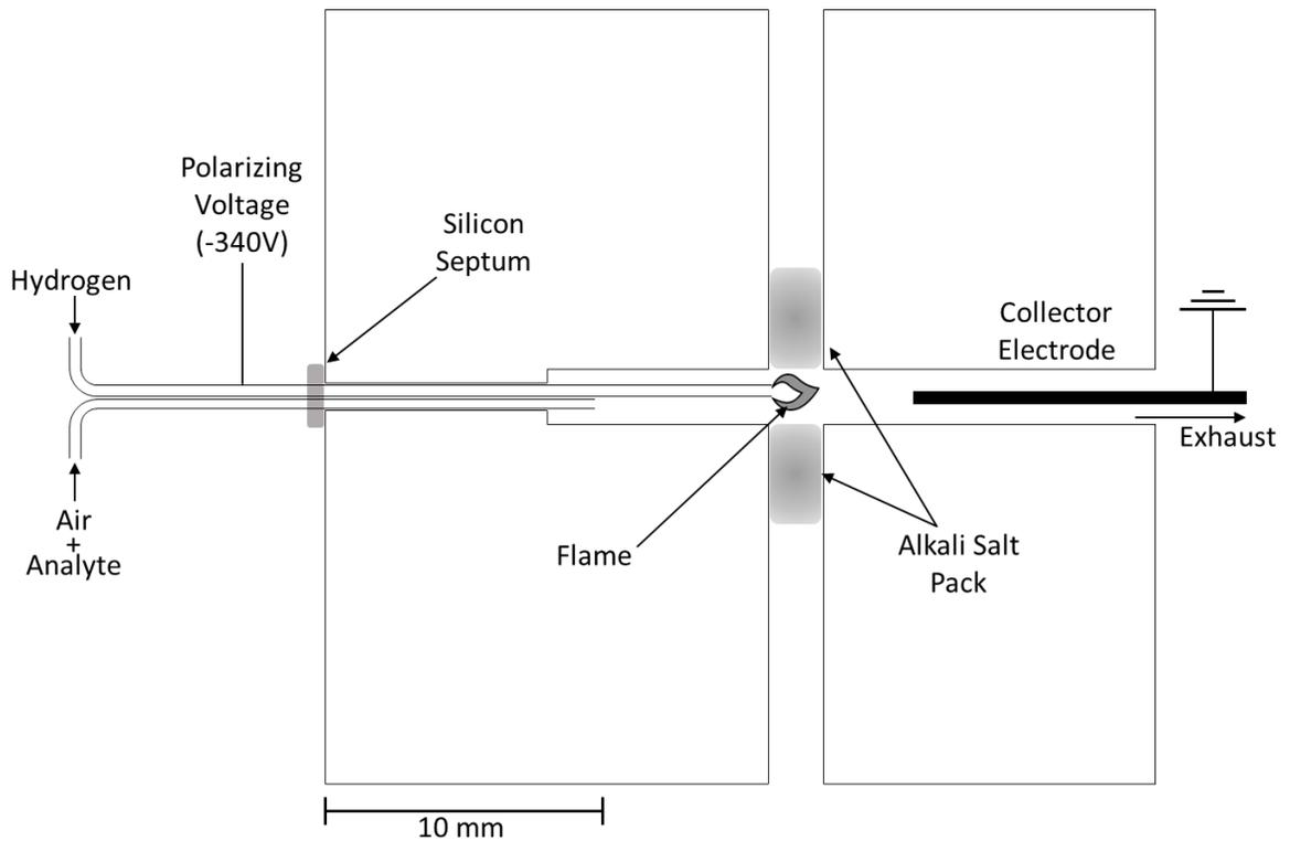
*Figure 2-1: Schematic diagram of the current AFID sensor design. The primary channel (horizontal) includes introduction of flame gases and analytes, collector electrode, and exhaust. Secondary salt channel (vertical) contains packed alkali salt*
