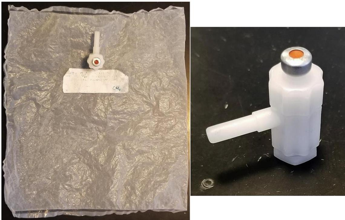
*Figure 2-4: Images of sampling bag used for testing (left) and on/off valve (right).*
