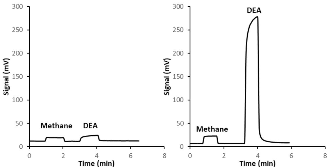
Figure 3-2: Sensor signal towards methane and diethylamine (DEA) sample bags without (FID mode, left) and with (AFID mode, right) RbCl salt present in channel.
