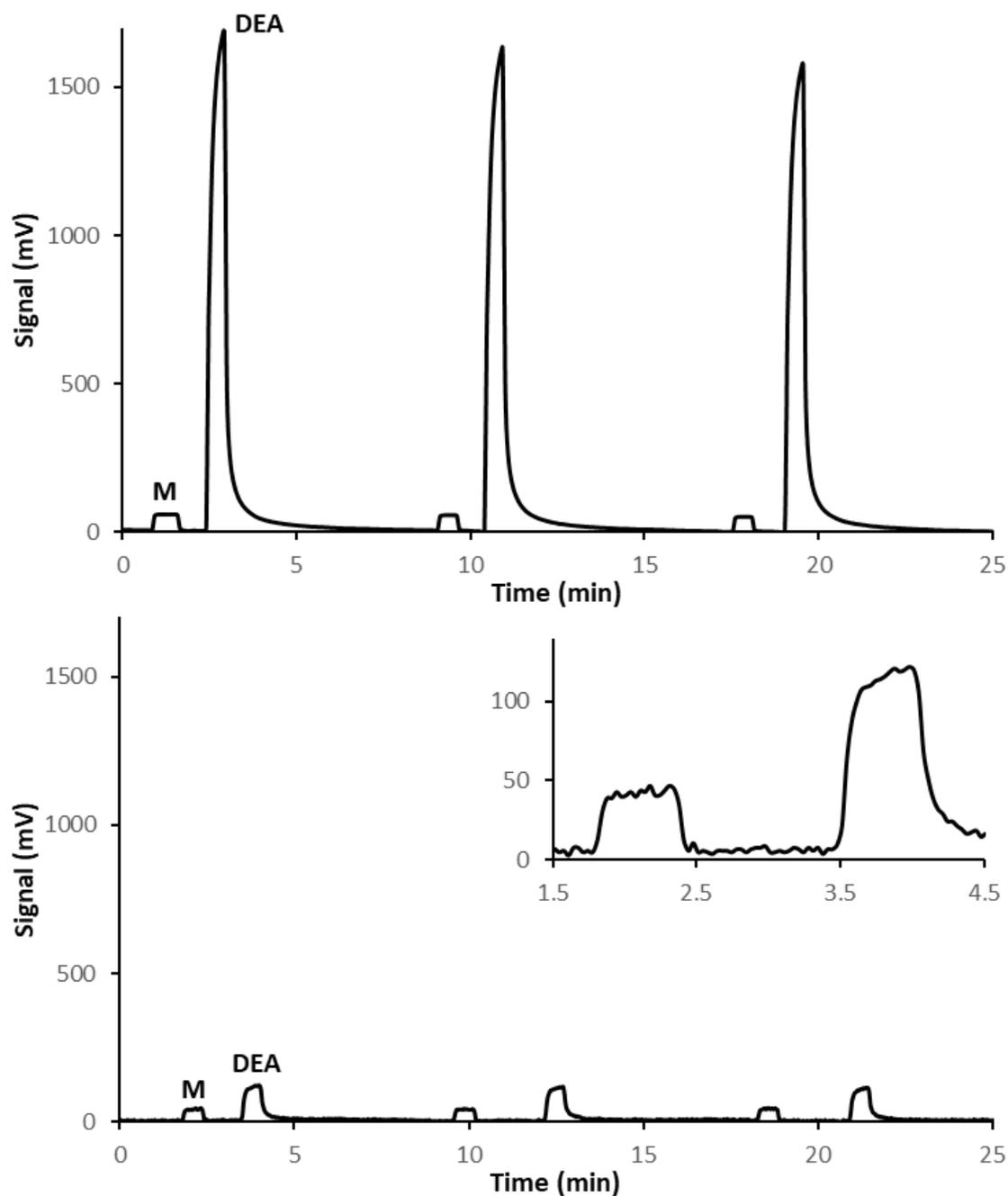
Figure 4-1: Comparison of identical methane (M) and diethylamine (DEA) sample signals in both the AFID (top) and FPD sensors (bottom). A magnified image of the first set of peaks in the FPD is also shown. Analyte concentrations are ~800 ng/mL each.
