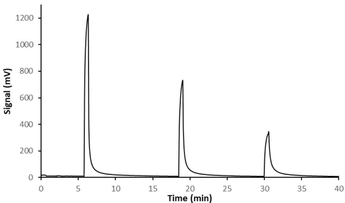
Figure 4-3: AFID sensor response to 5, 13, 26 %v/v of car exhaust to air sample bags (left to right) spiked with 800 ng/mL of DEA.
