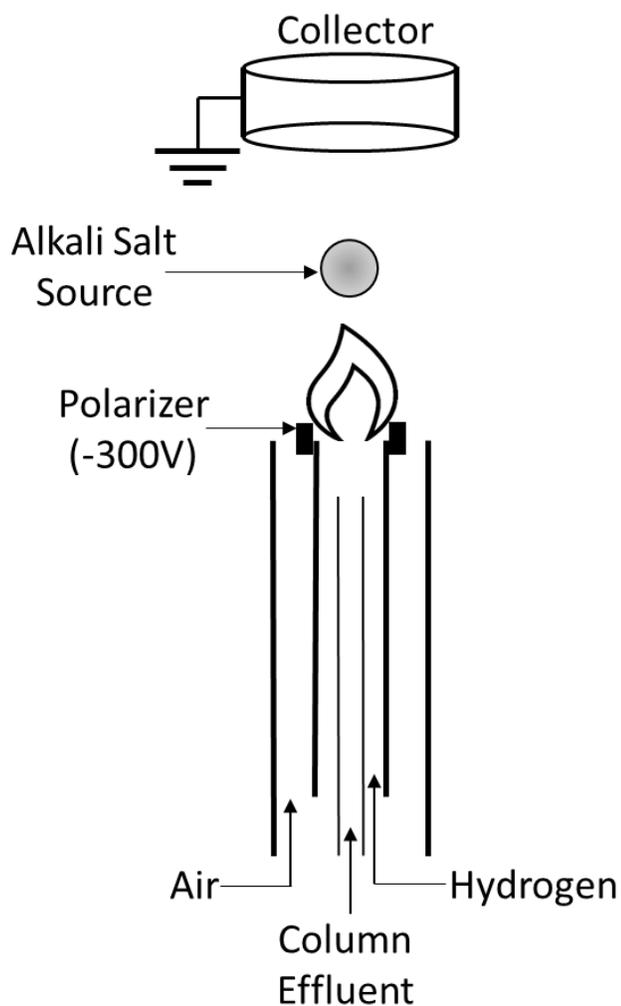
*Figure 1-5: A general schematic diagram of an AFID.*
