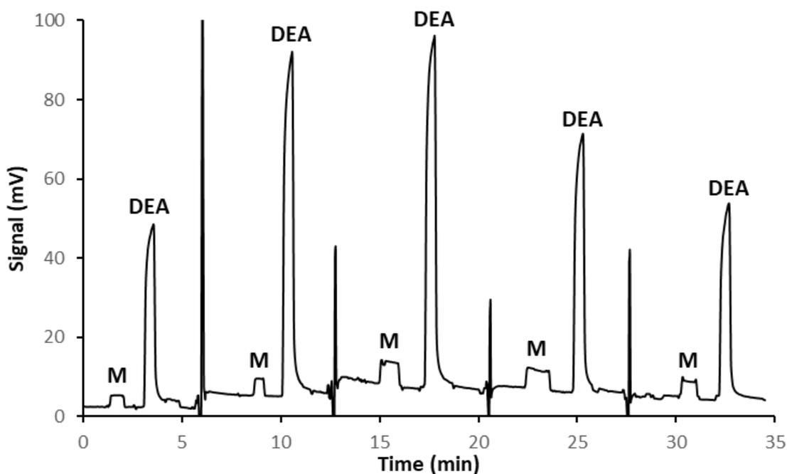
Figure 3-4: AFID response to methane (M) and diethylamine (DEA) as a function of hydrogen flow. Flows from left to right: 11, 13, 15, 17, and 19 mL/min. Intermittent spikes indicate a change in flow.
