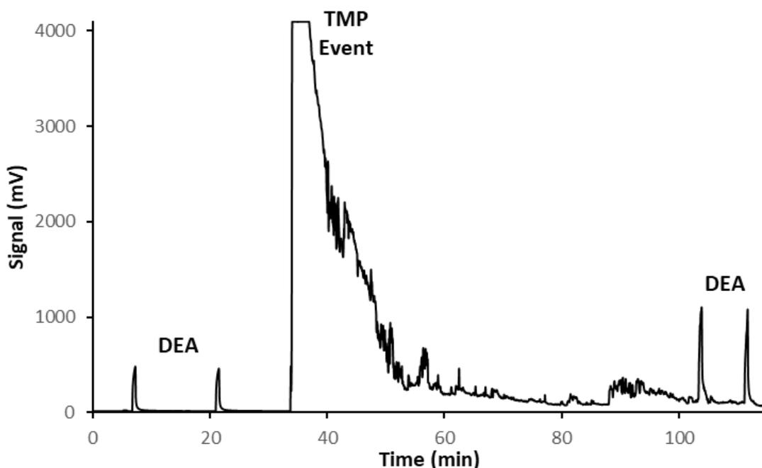
Figure 3-9: AFID sensor response to diethylamine sample bags (800 ng/mL) before (leftmost peaks) and after (rightmost peaks) sensor was subjected to concentrated levels of trimethyl phosphite (>1100 ng/mL) for ~30 seconds.
