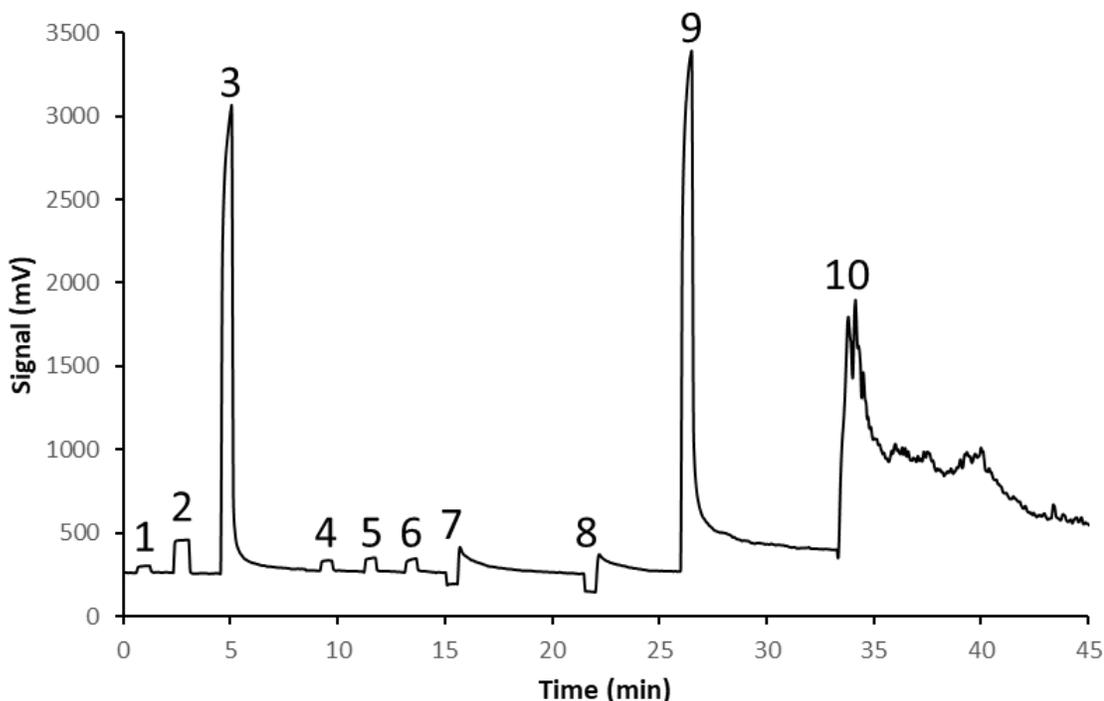
Figure 3-8: AFID sensor response toward various analytes under the optimum conditions. Analytes are: 1. air, 2. methane, 3. diethylamine, 4. methanol, 5. acetone, 6. tetrahydrofuran, 7. dichloromethane, 8. chloroform, 9. trimethyl phosphite, and 10. carbon disulfide. Concentrations are about 900 ng compound/mL each, except analytes 9 and 10 which were 12 and 140 ng/mL respectively.
