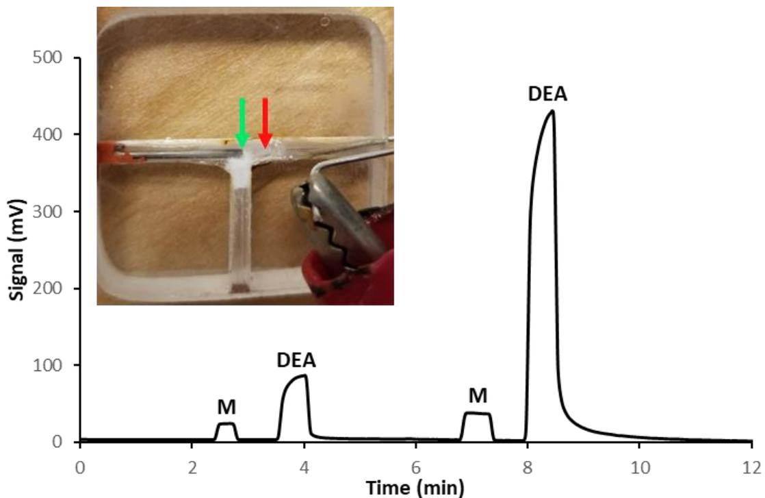
Figure 3-3: Methane (M) and diethylamine (DEA) response in the AFID sensor as flame position is altered. Left most peaks were produced when flame was in the position indicated in the image by the red arrow. Left most peaks were produced when flame was positioned at green arrow.
