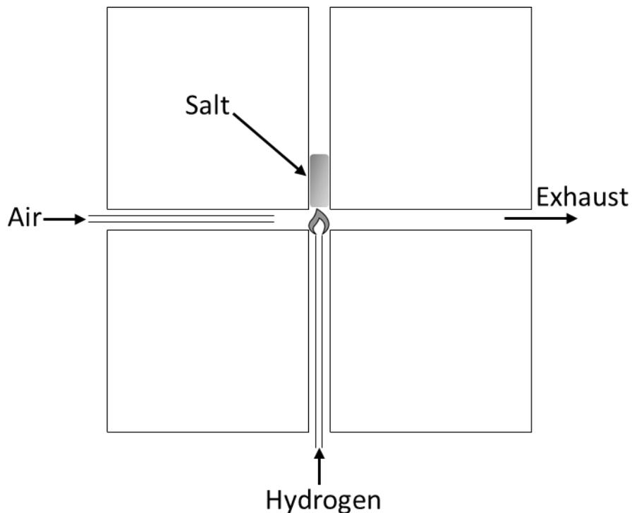
*Figure 3-1: Initial design of the planar-channelled AFID.*
