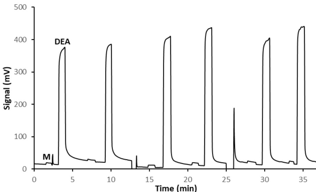
Figure 3-5: AFID response to methane (M) and diethylamine (DEA) as a function of air flow. From left to right (as doublets): 40 mL/min (pump), 60 mL/min (40 mL/min pump + 20 mL/min auxiliary), and 80 mL/min (40 mL/min pump + 40 mL/min auxiliary). Intermittent spikes indicate a change in flow.
