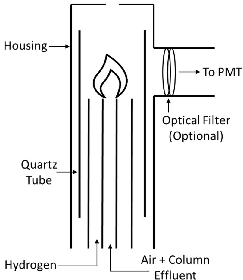
Figure 1-4: A general schematic diagram of an FPD.
