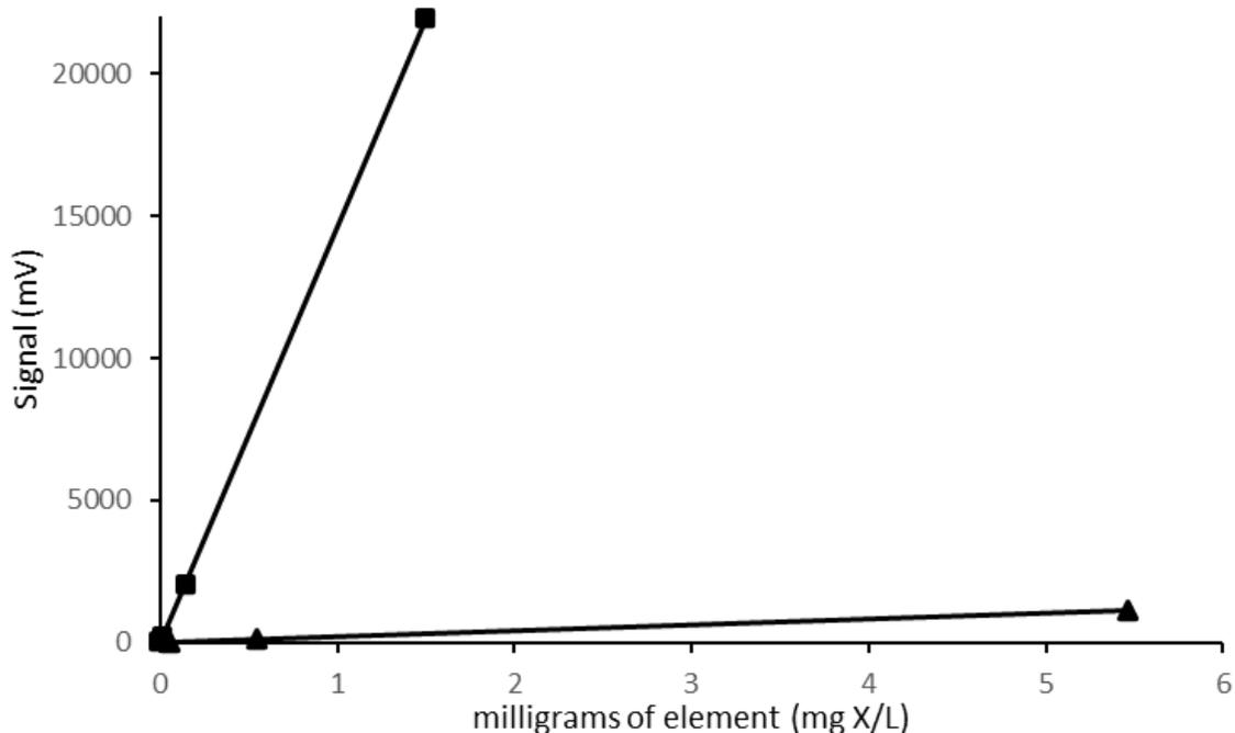
Figure 3-7: Calibration plot of the AFID sensor over three orders of concentration for both methane (▲) and diethylamine (■). Gas flows were 40 mL/min air, 14.5 mL/min hydrogen.
