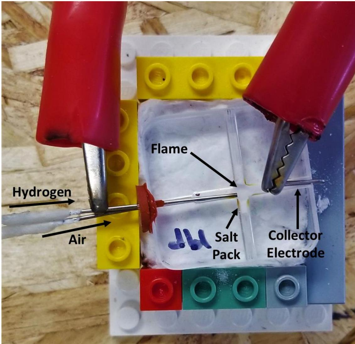
*Figure 2-3: An image of the AFID sensor operating under normal conditions.*
