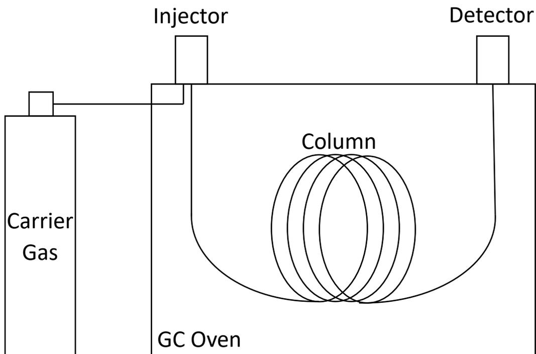
*Figure 1-1: A general schematic diagram of a conventional GC system.*
