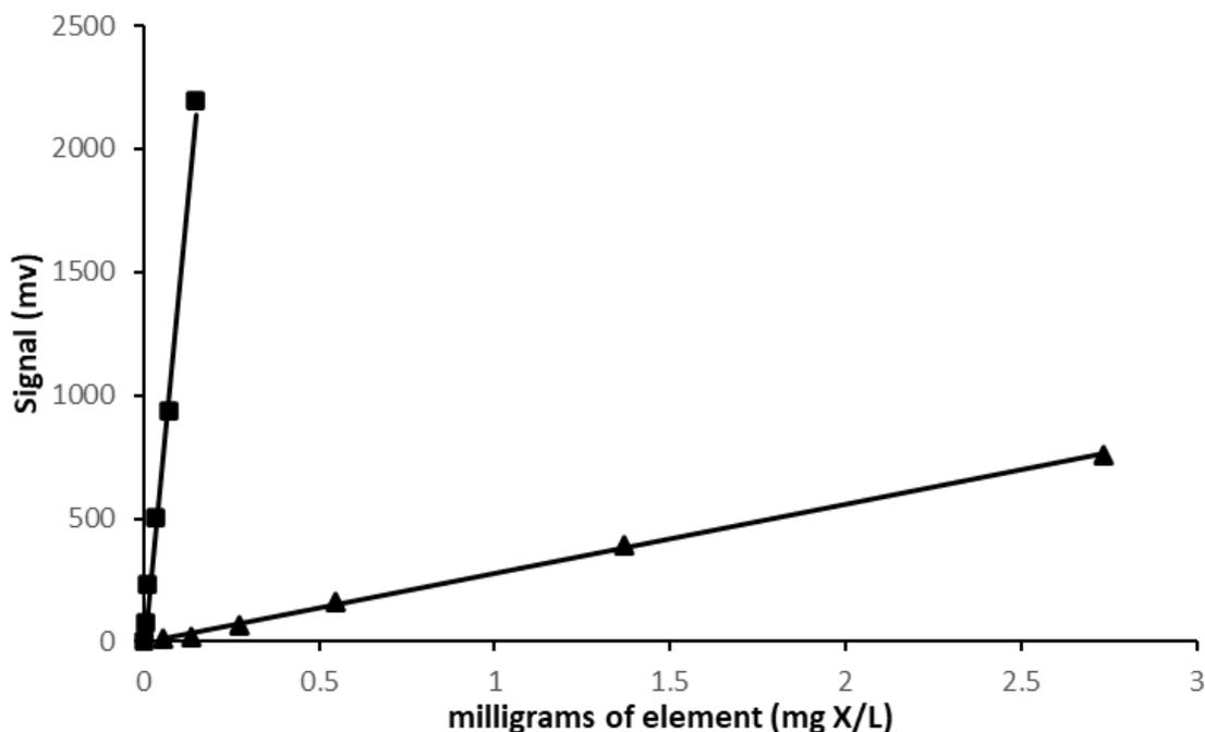
Figure 3-6: 6-point calibration plot of methane (▲) and diethylamine (■) in the AFID sensor. Gas flows were 40 mL/min air, 14.5 mL/min hydrogen.
