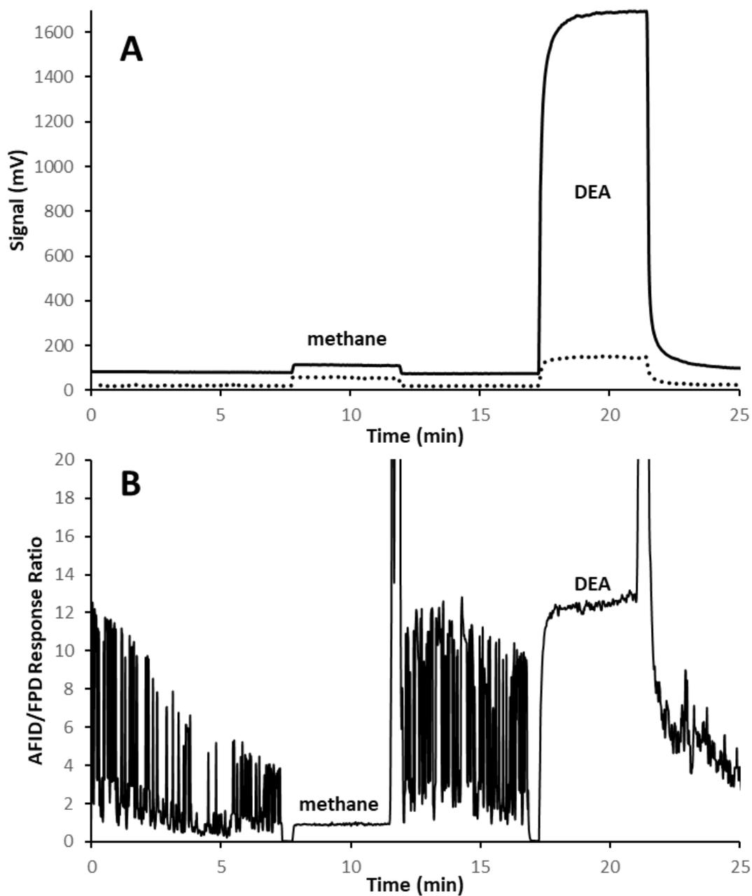
Figure 4-2: Simultaneous sensor response toward a methane and diethylamine (DEA) sample in both the AFID (solid line) and FPD (dashed line) devices under optimum conditions. Concentrations are about 800 ng/mL each. B) The ratio of the response traces shown in A after baseline subtraction.
