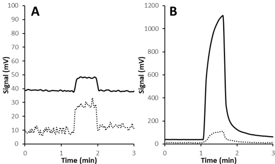
Figure 4-4: Simultaneous sensor response in both the AFID (solid line) and FPD (dashed line) devices to pure gasoline (A) and gasoline spiked with DEA (B). Concentrations are ~800 ppm of gasoline in either sample bag and 800 ng/mL of DEA in spiked bag.
