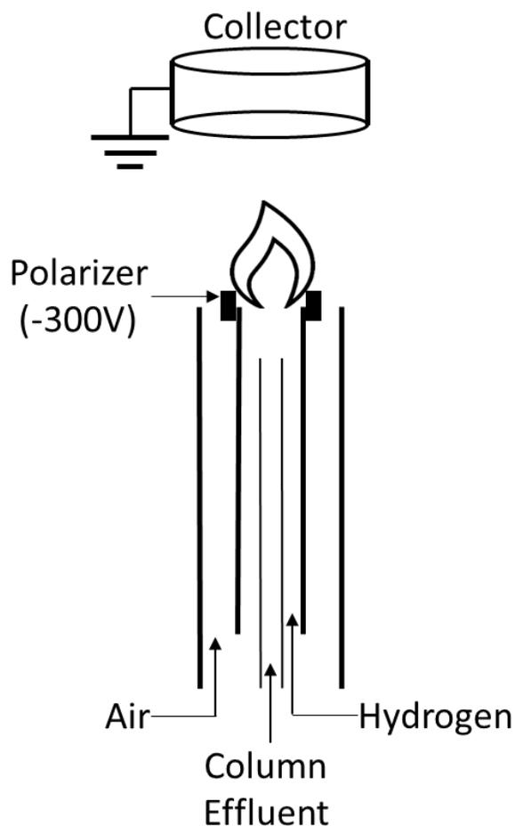
Figure 1-3: A general schematic diagram of an FID.
