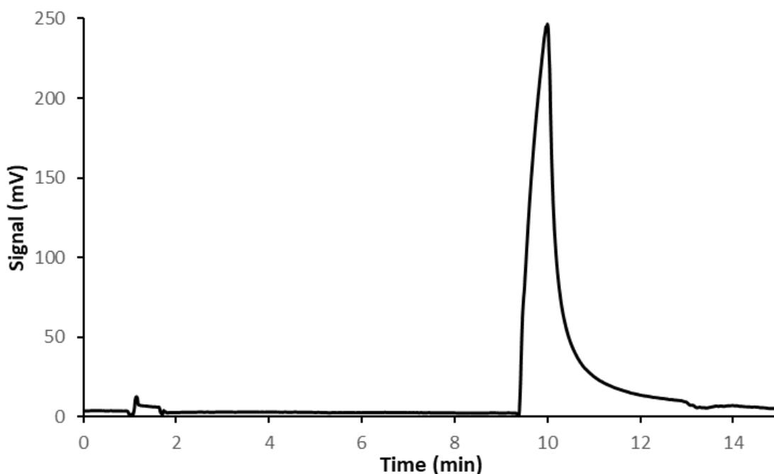
Figure 4-5: AFID response to the headspace over a 10 g piece of dried fish meat without (left peak) and with (right peak) 800 ng/mL of DEA. Time from spiking to testing was ~10 min.
