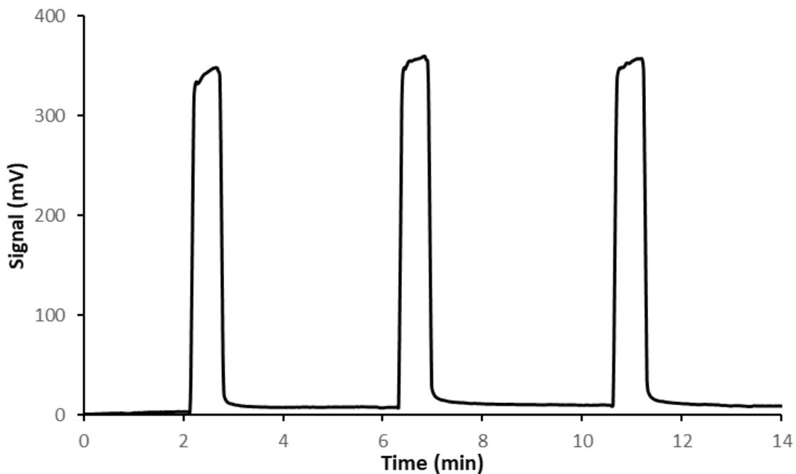
Figure 4-6: AFID sensor response to acetonitrile in air at a concentration equivalent to sub IDLH levels of CK/AC (44 ng/mL). Three replicate runs shown.
