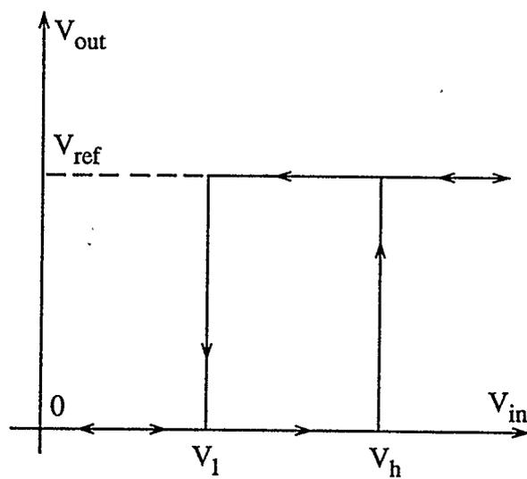
Fig.2.3 Schmitt trigger and its transfer characteristic
