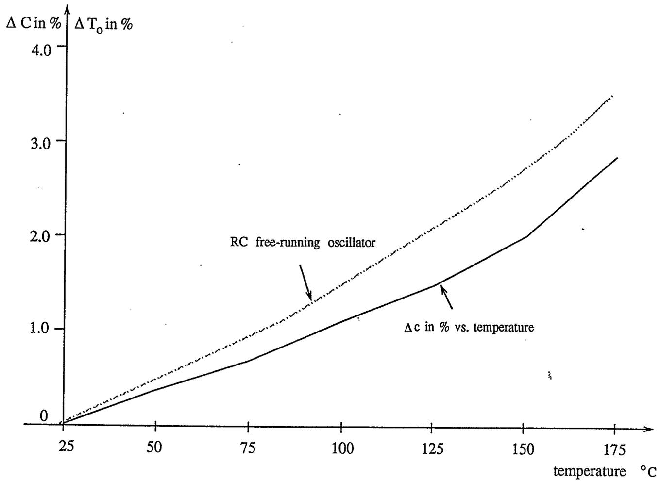
Fig. 2.10 % capacitance change and % period change vs. temperature
