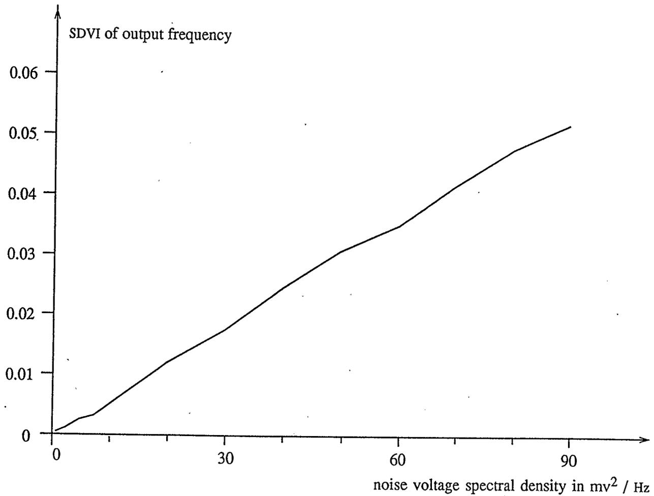
Fig. 6.6 Simulated noise characteristic for RC free-running oscillator
