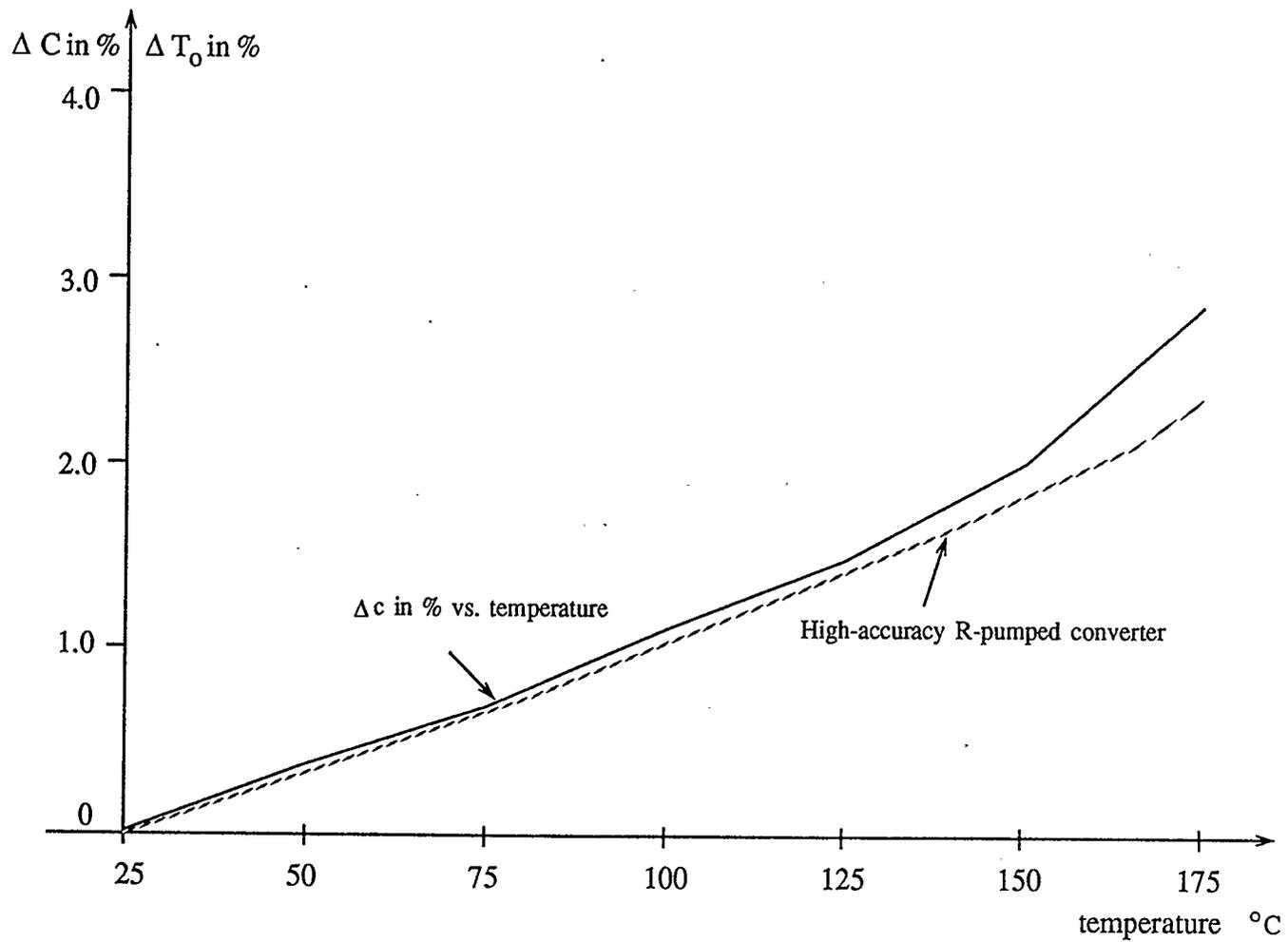
Fig. 4.6 % capacitance change and % period change vs. temperature
