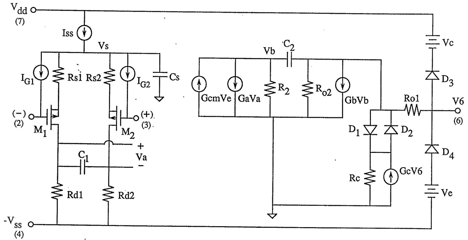
Fig. 6.3 Macromodel with MOSFET input stage for TSC913.
