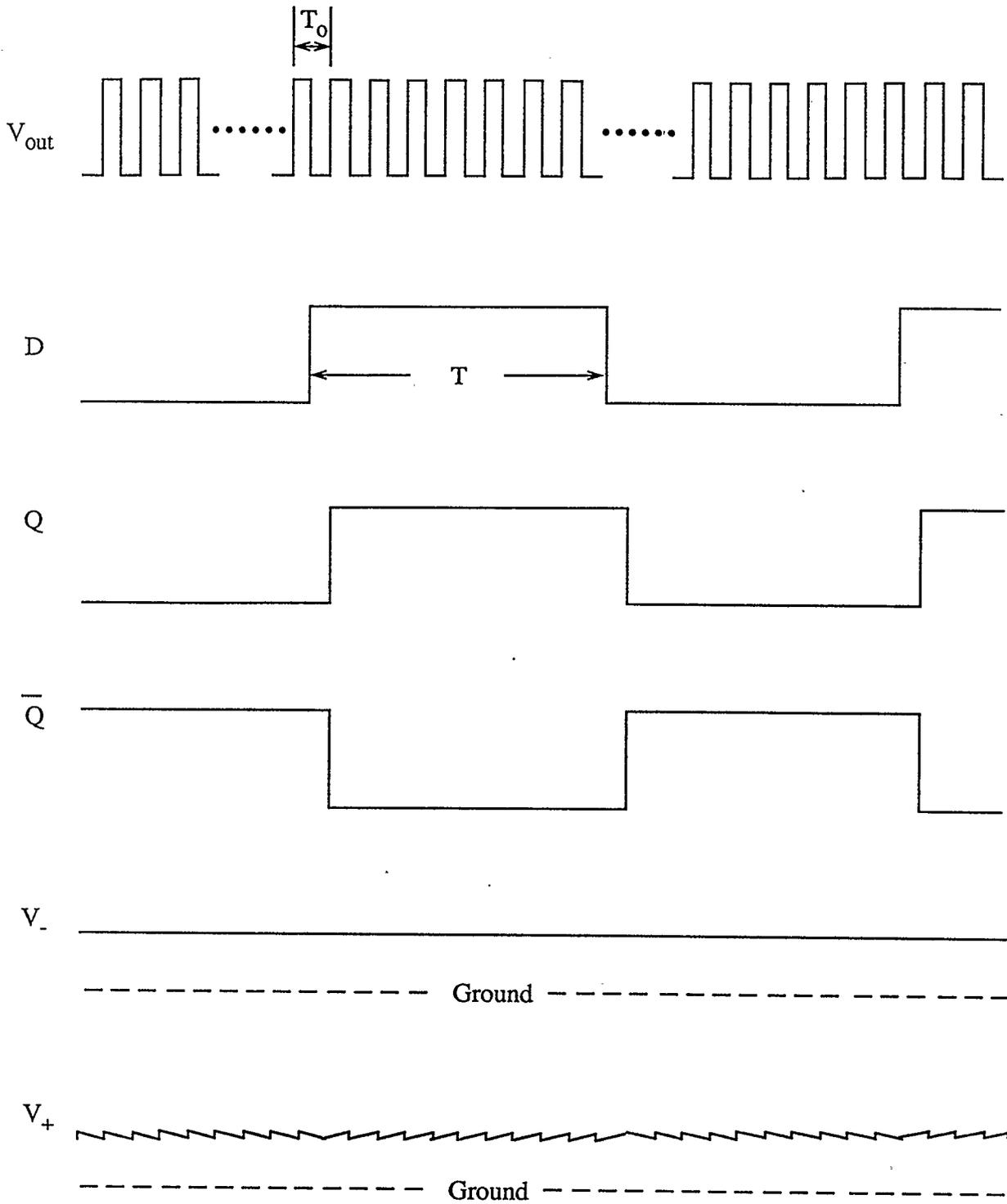
Fig. 4.2 Timing diagram for the modified capacitance-to-frequency conversion circuit
