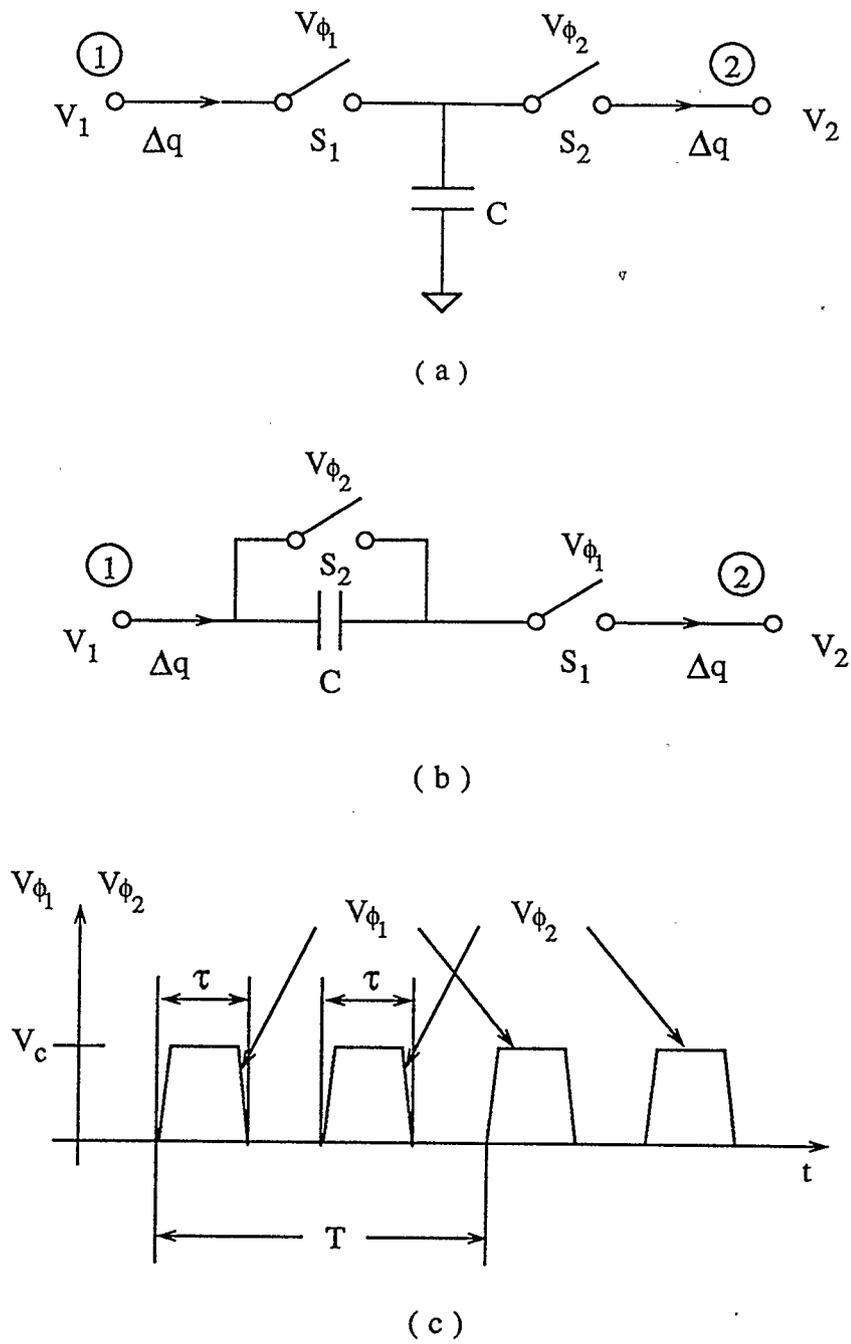
Fig. 3.1 Switched capacitor simulated resistors : (a) shunt circuit; (b) series circuit; (c) clock waveforms
