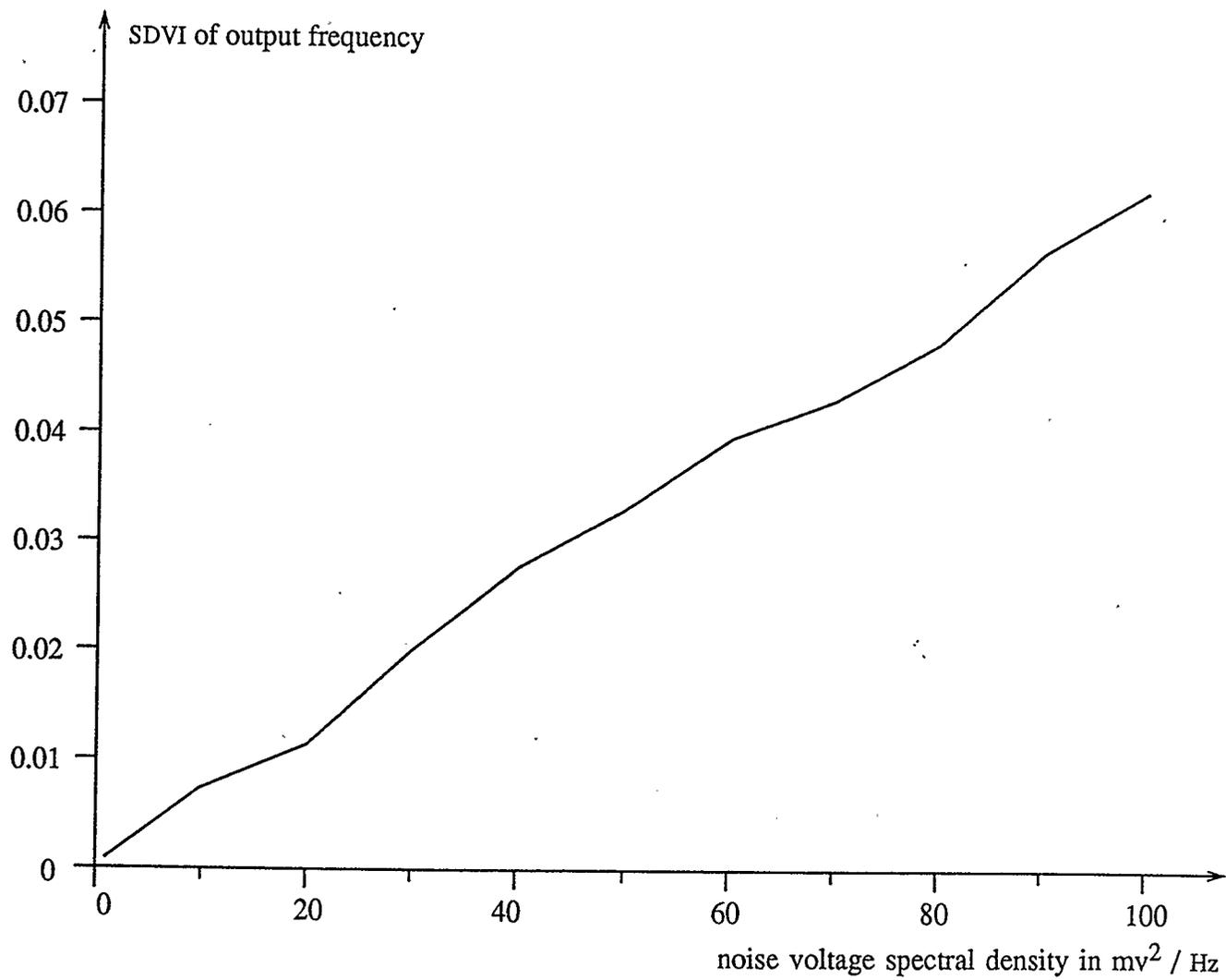
Fig. 6.7 Simulated noise characteristic for R-pumped converter
