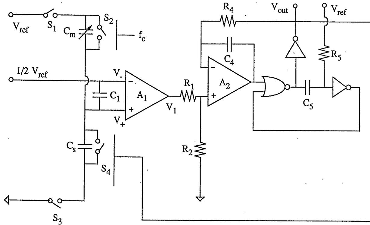
Fig. 5.1 Schematic diagram of the two-capacitor pumped capacitance-to-frequency conversion circuit
