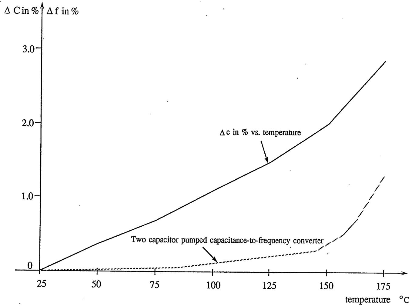
Fig.5.7 % capacitance change and % frequency change vs. temperature
