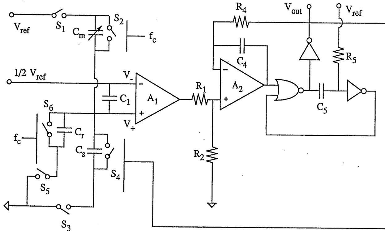
Fig. 5.5 Schematic diagram of the modified two-capacitor pumped capacitance-to-frequency conversion circuit
