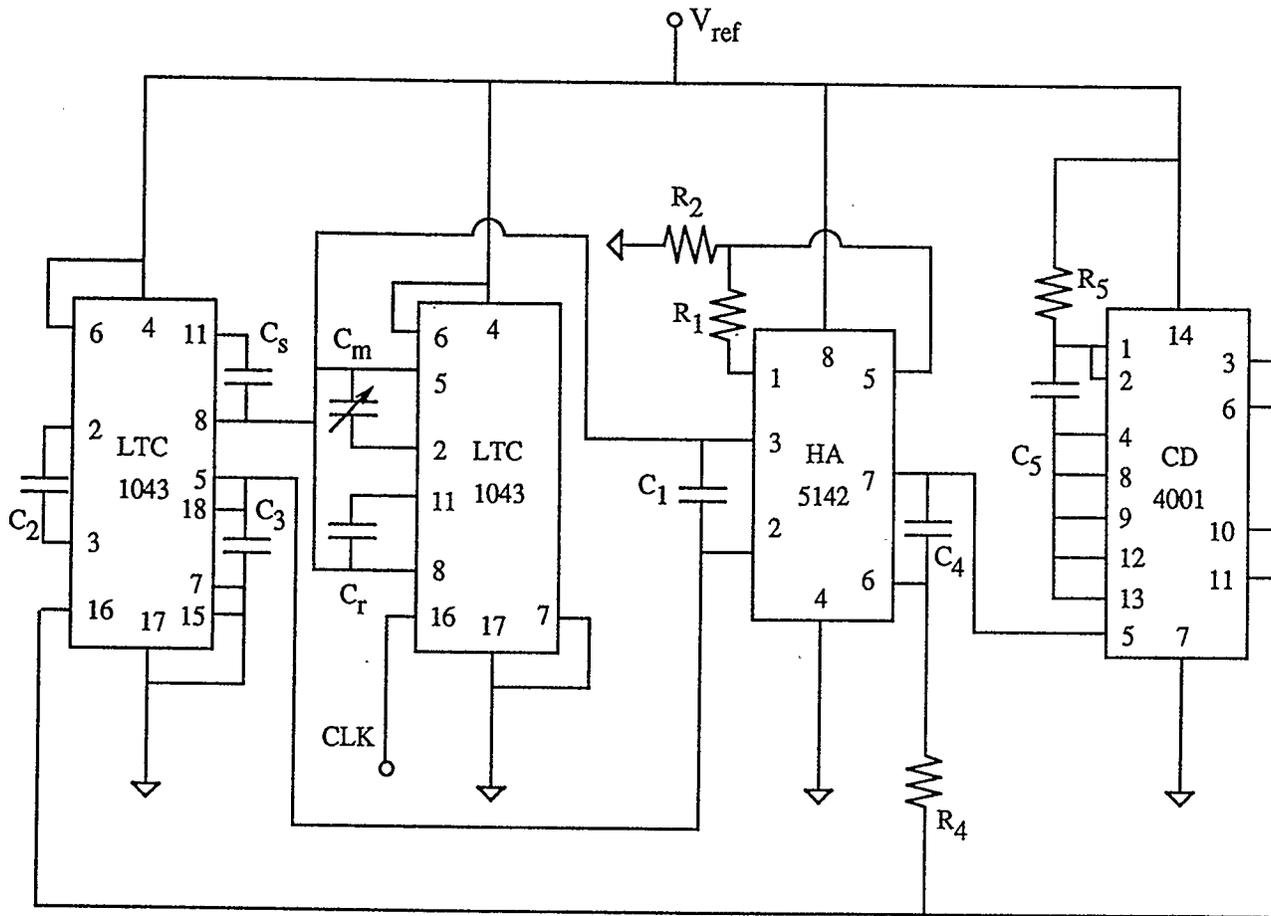
Fig. 5.6 Practical implementation for the modified two-capacitor pumped capacitance-to-frequency converter
