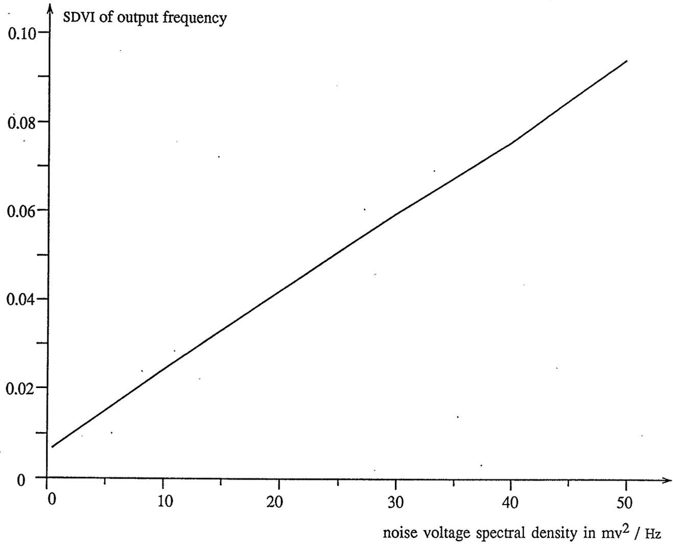
Fig. 6.8 Simulated noise characteristic for two-capacitor pumped converter
