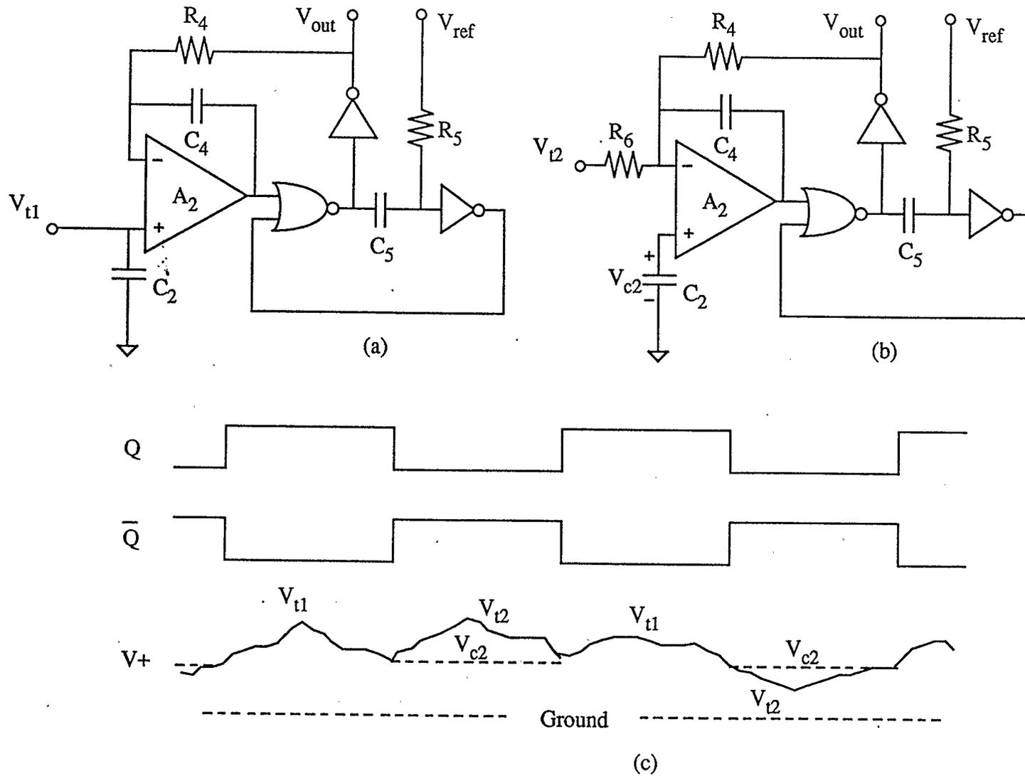
Fig.4.4 (a) The VFC circuit when  $Q$  is high (b) The VFC circuit when  $Q$  is low
