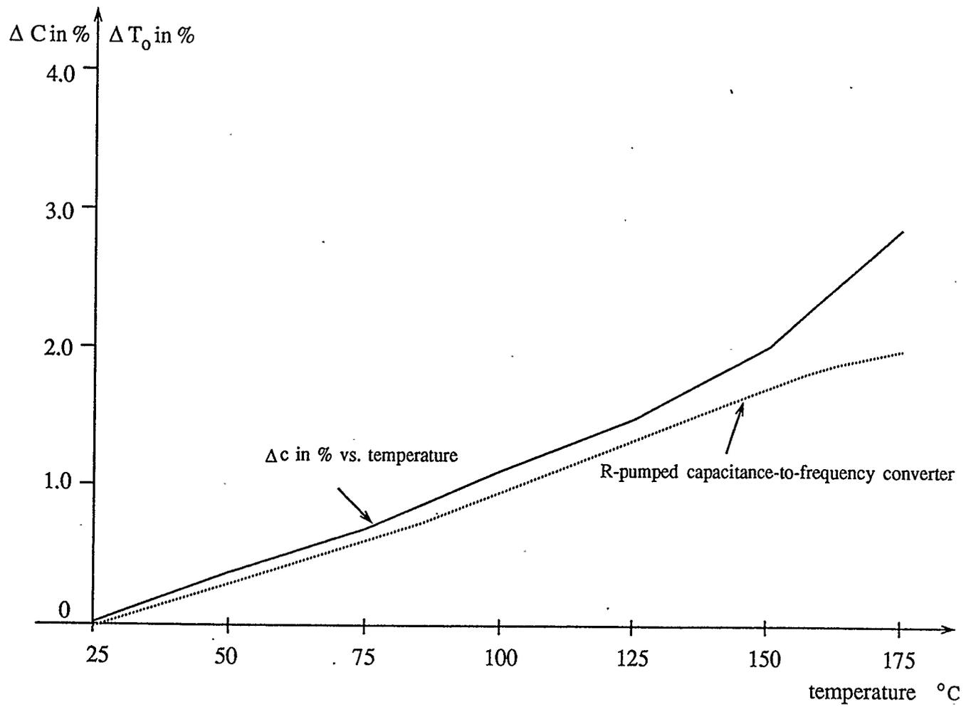
Fig. 3.9 % capacitance change and % period change vs. temperature
