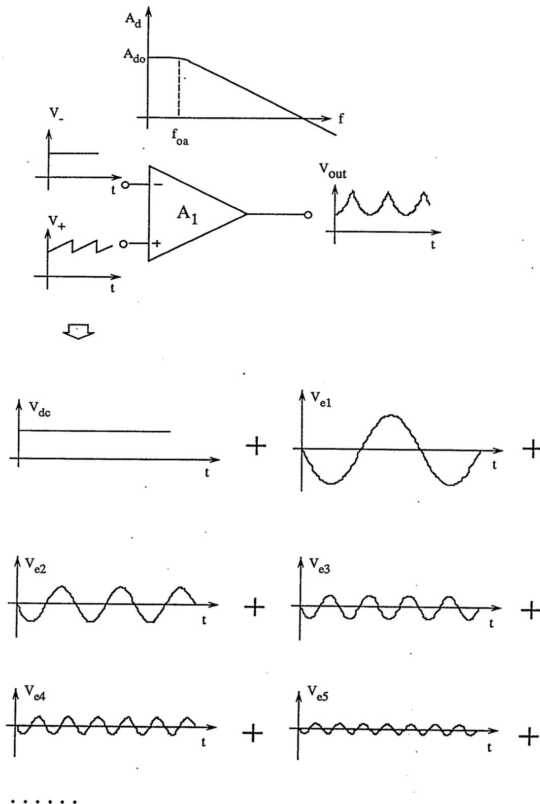
Fig. 3.4 A diagram illustrating the effects of input ripple voltage and frequency response characteristics of op-amp  $A_1$
