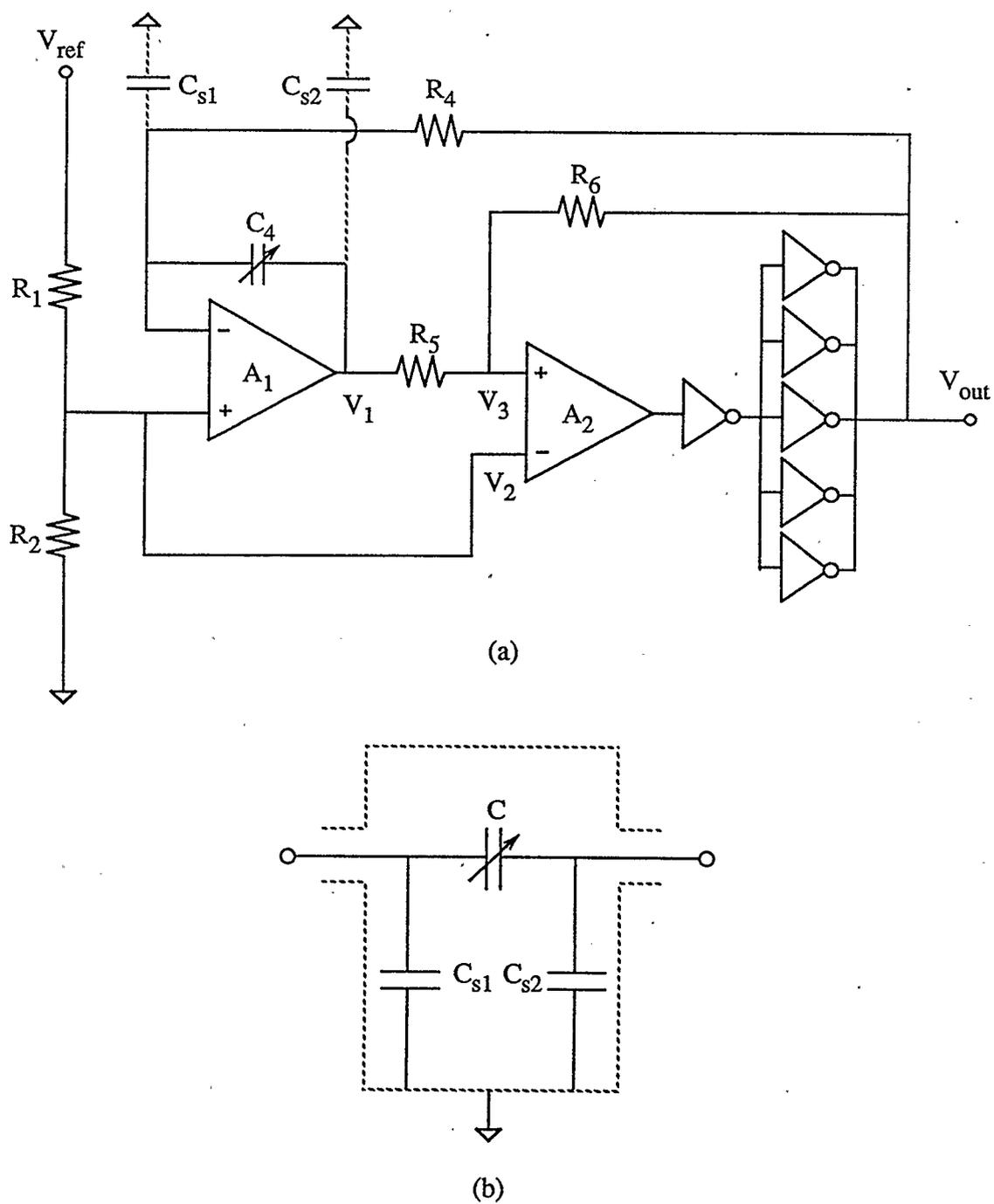
Fig. 2.1 (a) Schematic of the basic RC oscillator with three-terminal capacitor
