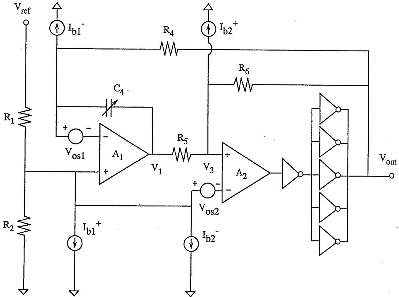
Fig.2.7 Basic RC oscillator showing effects of input offset voltage and input bias currents
