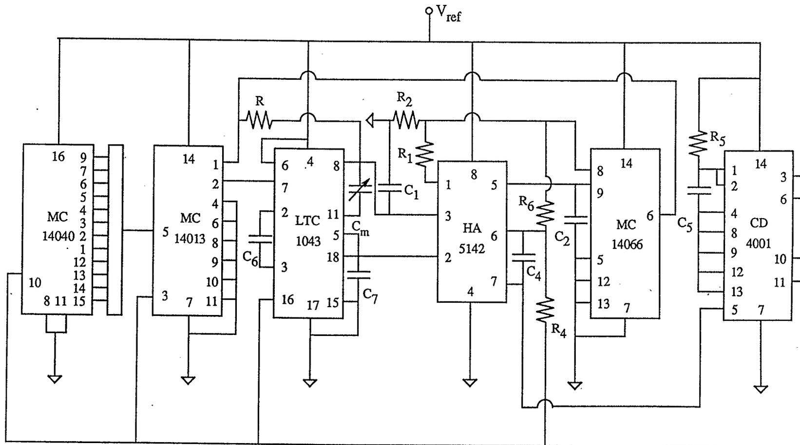
Fig. 4.5 Practical implementation for the modified R-pumped capacitance-to-frequency converter
