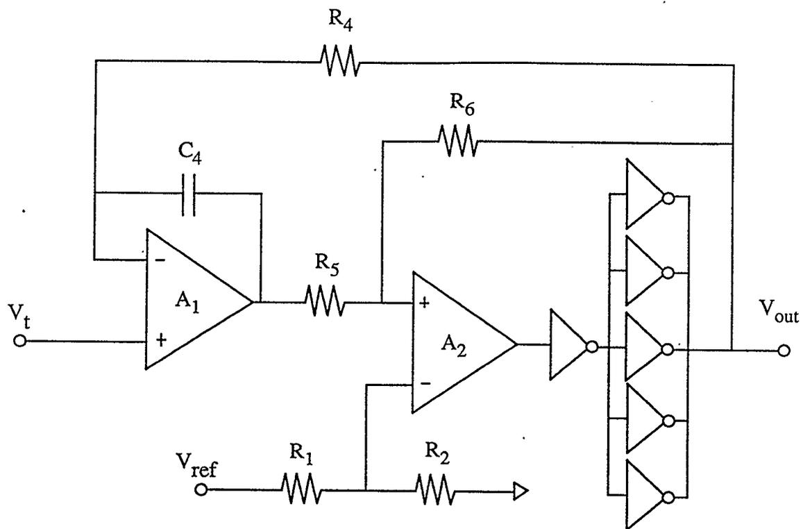
Fig. 2.5 Schematic of VFC
