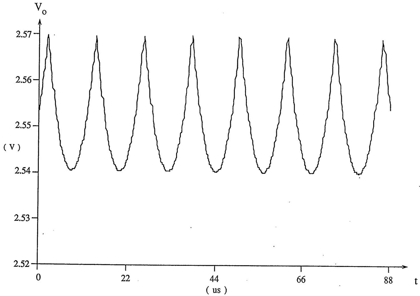
Fig. 3.5 Output waveform of open-loop amplifier  $A_1$
