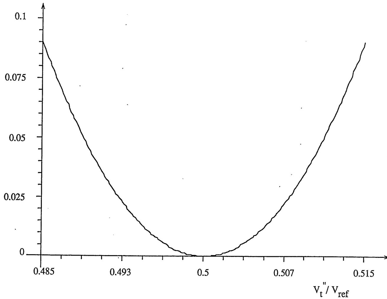
Fig. 2.8 Variation in  $f_0$  due to variations in  $V_t''/V_{ref}$  about an operating point  $V_t''/V_{ref} = 0.5$
