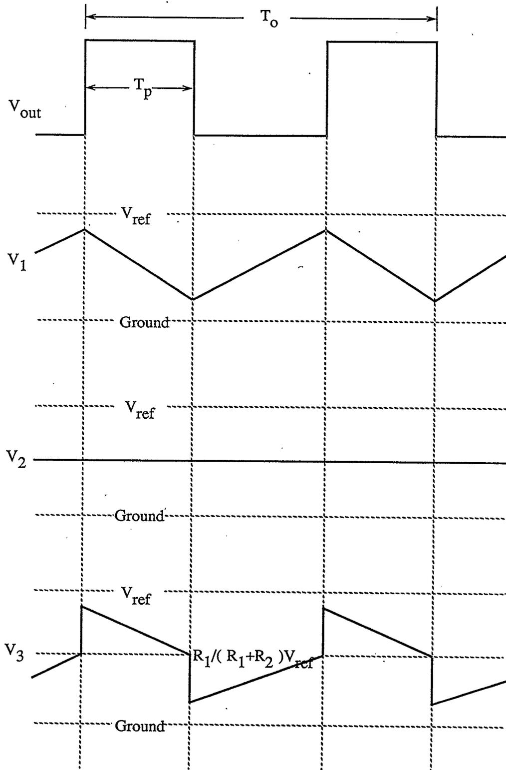
Fig.2.2 Voltage waveforms of the RC oscillator
