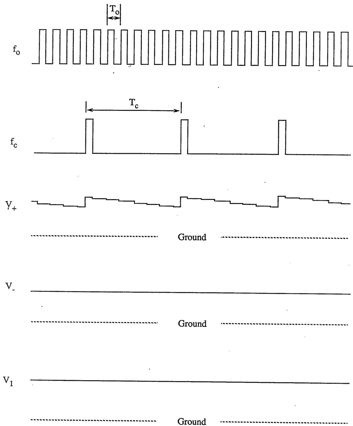
Fig. 5.2 Timing diagram of the two-capacitor pumped capacitance-to-frequency conversion circuit
