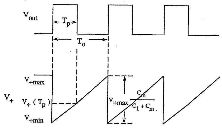
Fig. 3.3 The basic capacitance-to-frequency converter and the voltage waveform at the non-inverting input of  $A_1$
