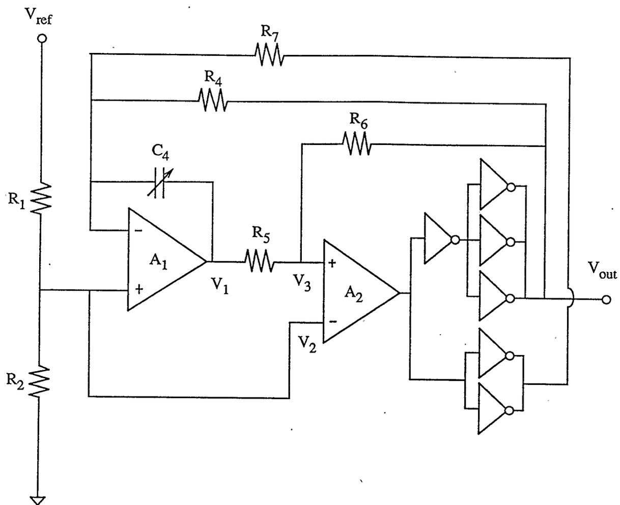
Fig.2.4 Schematic of RC oscillator with two ratioed charging-discharging resistors
