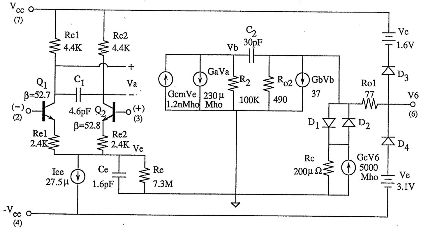
Fig. 6.2 A 741 operational amplifier macromodel
