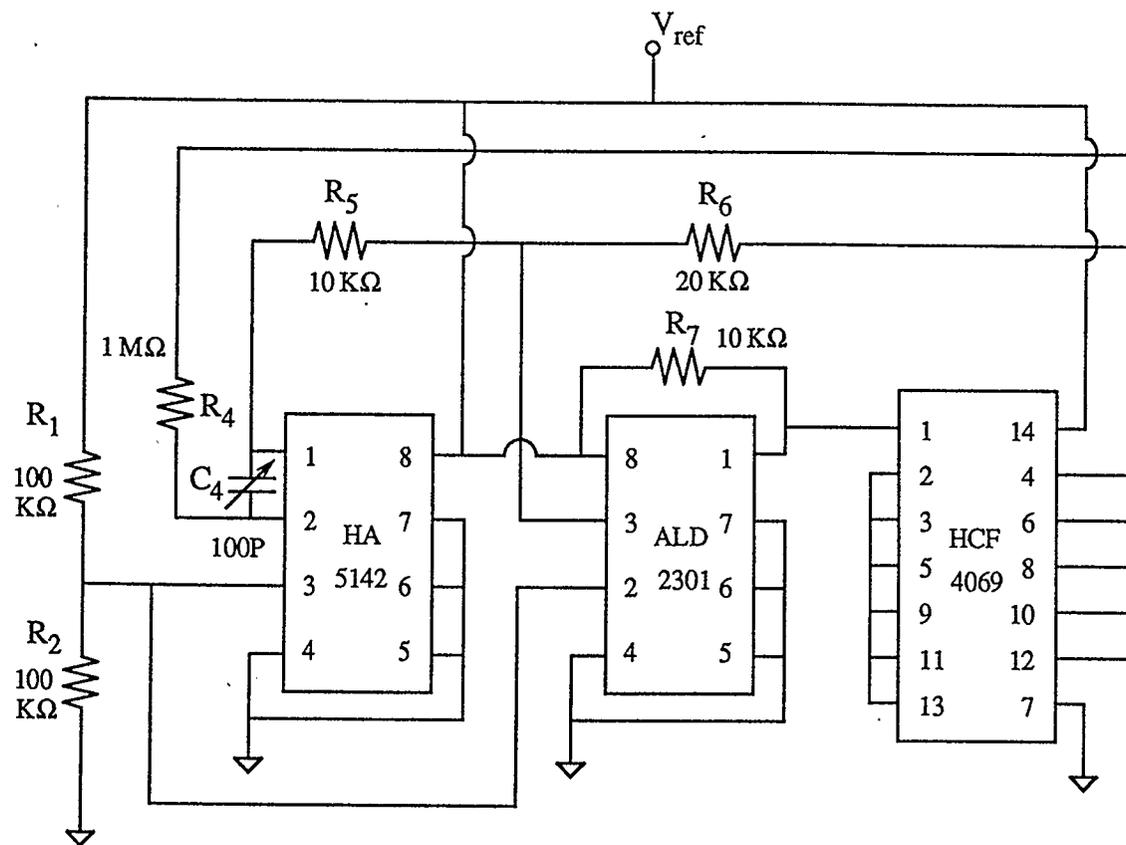
Fig. 2.9 Practical implementation for the RC free-running relaxation oscillator
