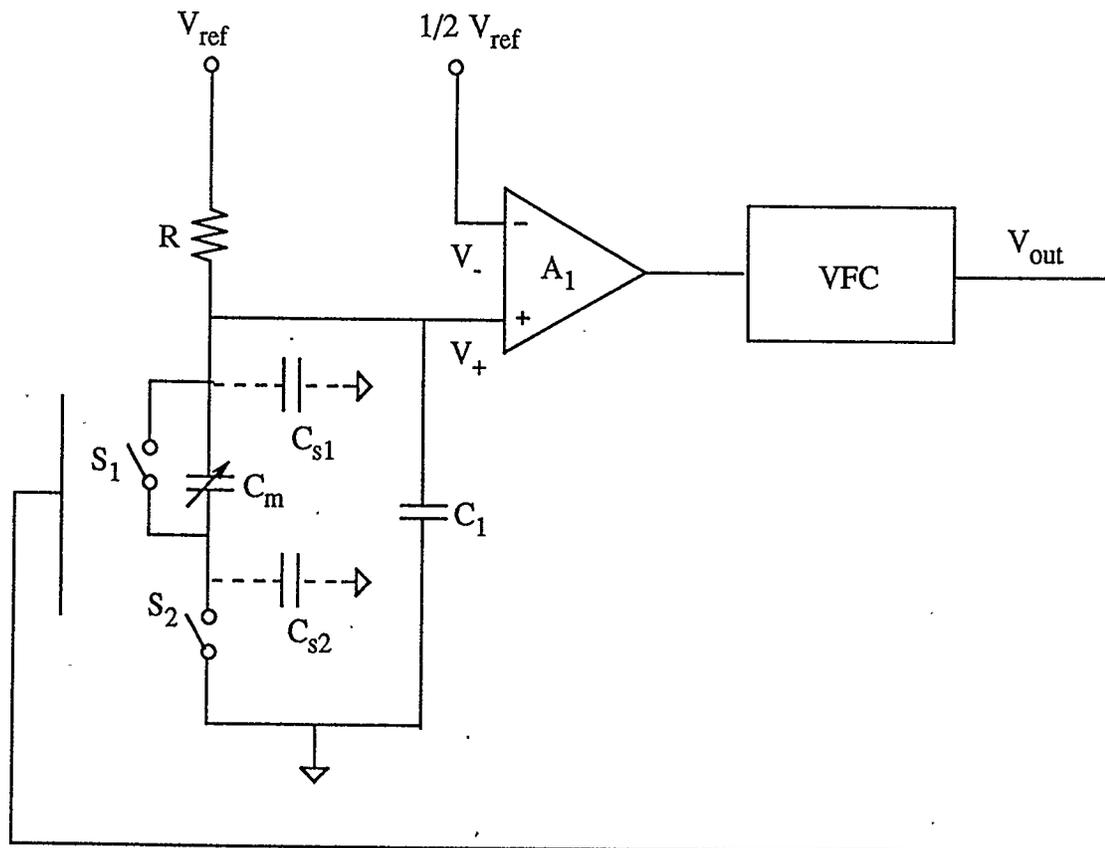
Fig. 3.6 The switched capacitor capacitance-to-frequency conversion circuit with a typical three-terminal capacitor
