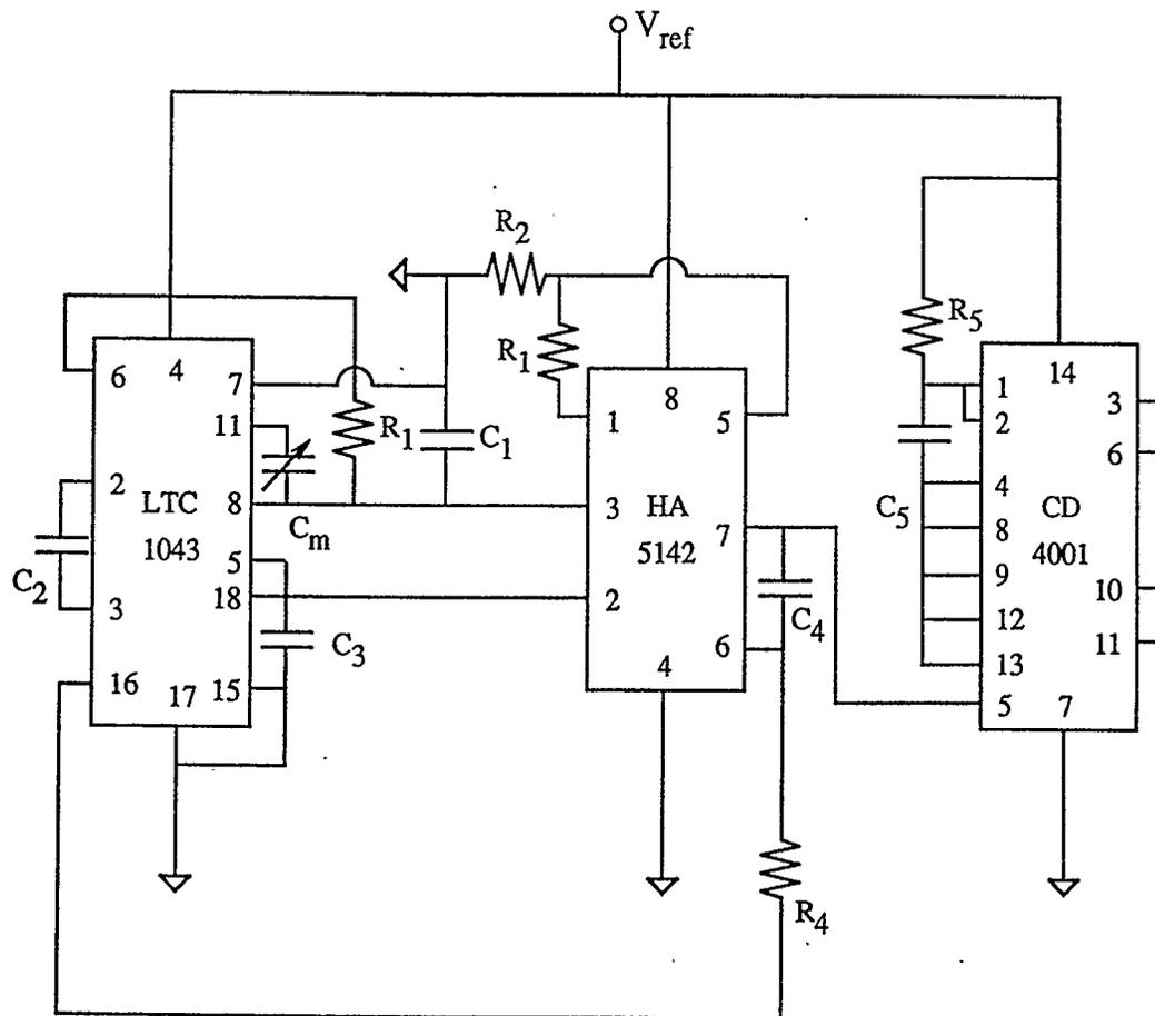
Fig. 3.8 Practical implementation for the R-pumped capacitance-to-frequency converter
