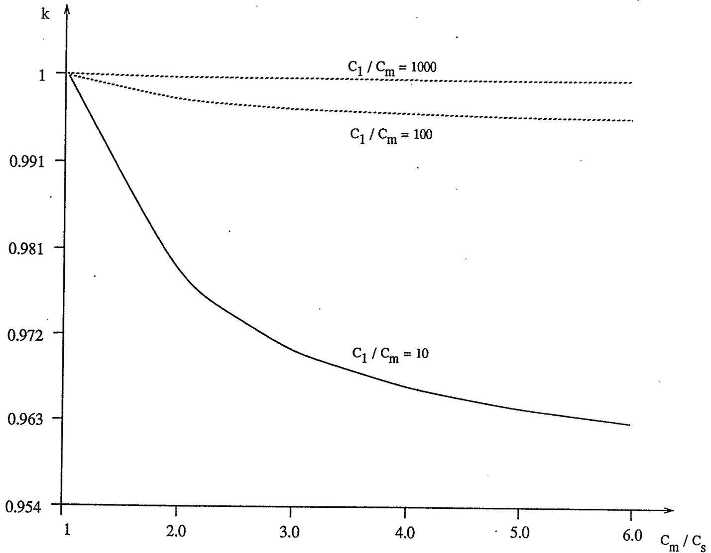
Fig. 5.4 The relationship between factor  $k$  and the capacitance ratio  $C_m / C_s$  for different capacitance ratios  $C_1 / C_m$
