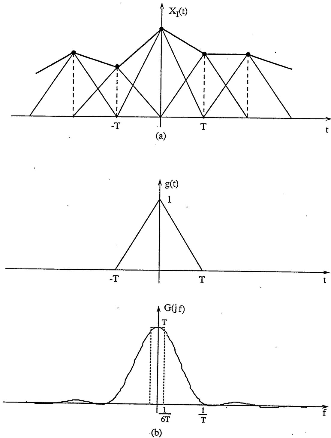
Fig. 6.5 (a) Straight line linear interpolation
