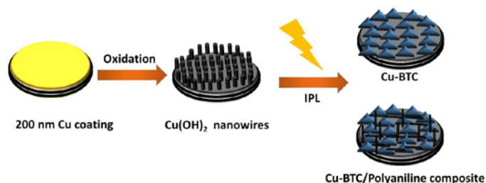
Fig. 2. Schematic illustration of the two-step method for the fabrication of sensing films (Cu-BTC or Cu-BTC/PANI nanocomposite).
