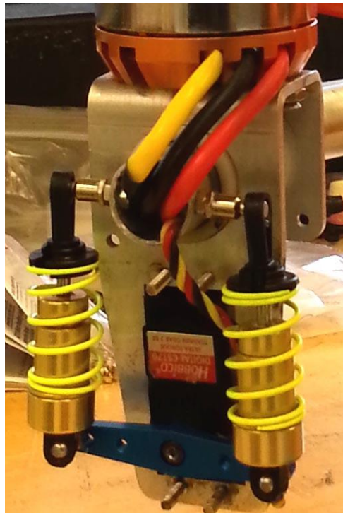
Figure 4-18. Dampers and centering springs on Nymbus bicopter.
