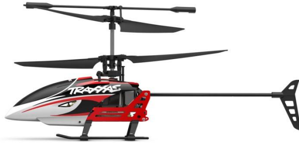
Figure 5-3. Coaxial R/C helicopter, with electronic yaw stabilization consisting of yaw gyro connected to differential speed control of the two rotors. (Source: www.traxxas.com , 2014)
