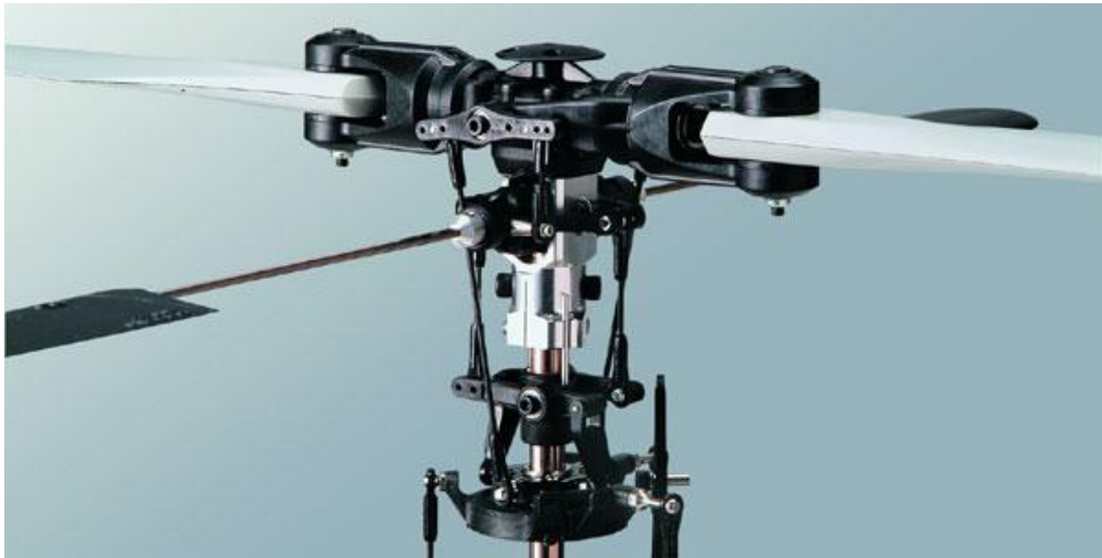
Figure 1-1. Bell-Hiller helicopter rotor head showing flybar. (Hirobo)
