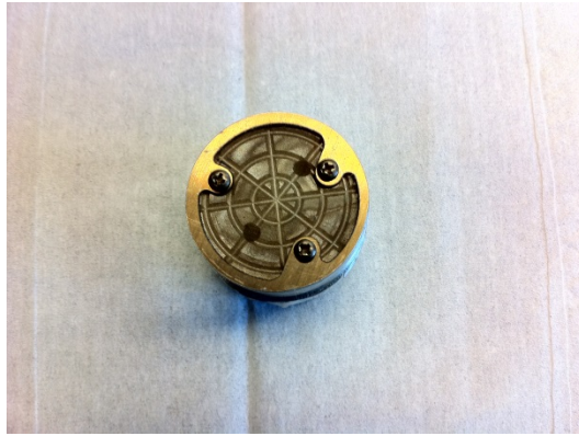
Figure 3.2 Inner-face view of sand pack head showing the installed screen and distribution channels
