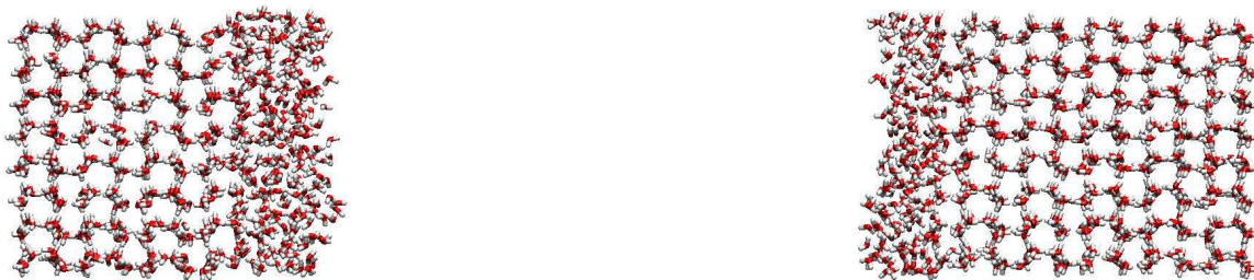
Figure 2.1: Snapshot from the configuration of the equilibrated system taken from the basal simulation at 245 K. Hydrogen and oxygen atoms are represented in white and red colors, respectively.
