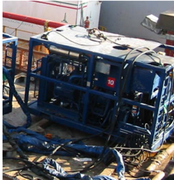
Figure 3-2: Power pack skid unit
