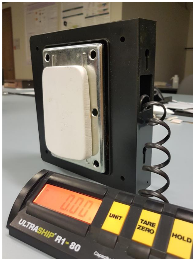
Figure A-5 - Moulding of the template used to produce the pad of the PCO attached to the scale. The mould allowed full surface area contact of the pad when tightening the PCO.
