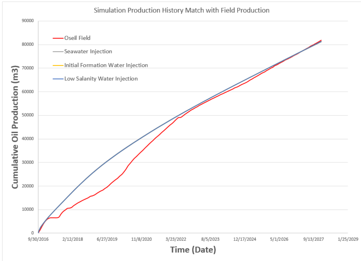
Figure 5.2.2.1 History Match of Field Production Data vs. Simulation Production Data
