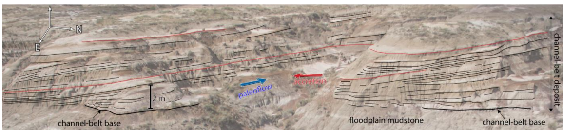
Figure 5.1. Geologic interpretations (line drawing on 2D field photograph), a common conventional method to highlight stratigraphic architecture and distribution of related units. Mudstones are grey to light brown, sandstones are light grey to white. This process is often performed on photos or a photomosaic acquired in the field.
