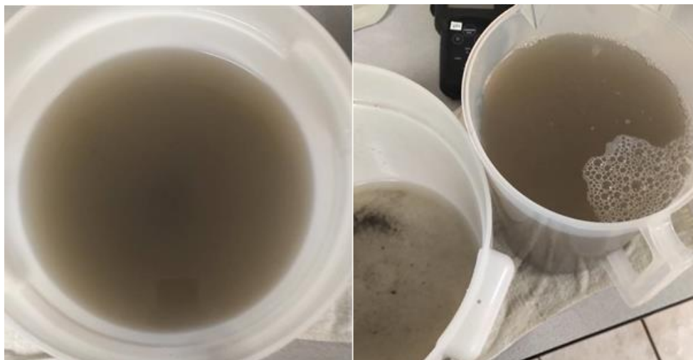
Run-2, trial-1 Day-0 Septic wastewater filtered to 100 µm.
