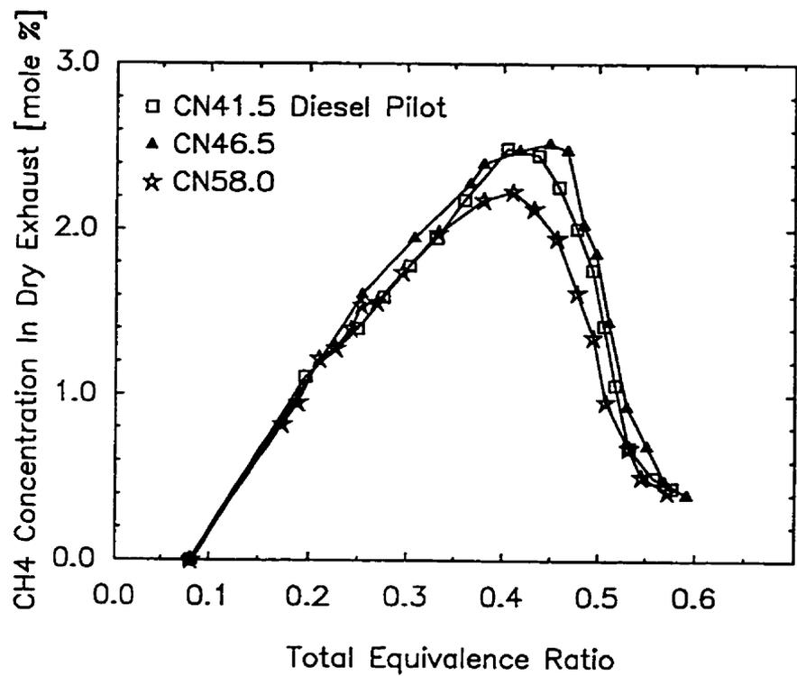
Figure 4.4.7 Variation of Dry Exhaust CH<sub>4</sub> Concentration with Total Equivalence Ratio for Dual Fuel Operation with Methane when Using Different Cetane Number Fuels with a 0.20 kg/h Pilot
