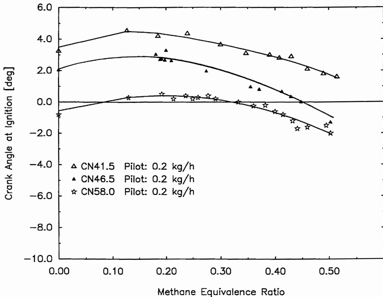
Figure F.1.1 Variations of the Point of Ignition with Gas Equivalence Ratio for Dual Fuel Operation with Methane when Using Different Cetane Number Fuels with a 0.20 kg/h Pilot
