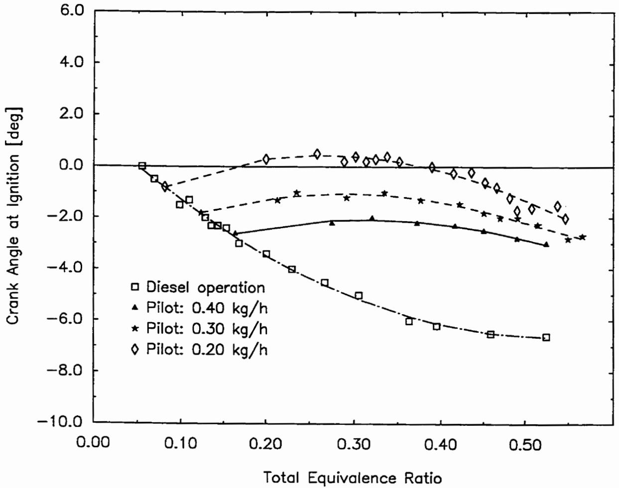
Figure 4.2.9 Variations of the Point of Ignition with Total Equivalence Ratio for Dual Fuel Operation with Methane when Using a 58.0 Cetane Number Fuel with Different Pilot Quantities
