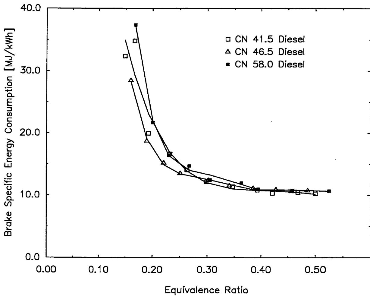
Figure 4.1.2. Variations of Brake Specific Energy Consumption with Equivalence Ratio for Diesel Operation when Using Different Cetane Number Fuels
