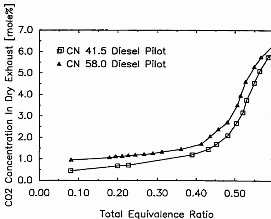
Figure F.1.13 Variation of Dry Exhaust CO<sub>2</sub> Concentration with Total Equivalence Ratio for Dual Fuel Operation with CH<sub>4</sub>-N<sub>2</sub> Mixture (50% by Mass CH<sub>4</sub>) when Using Different Cetane Number Fuels with a 0.20 kg/h Pilot
