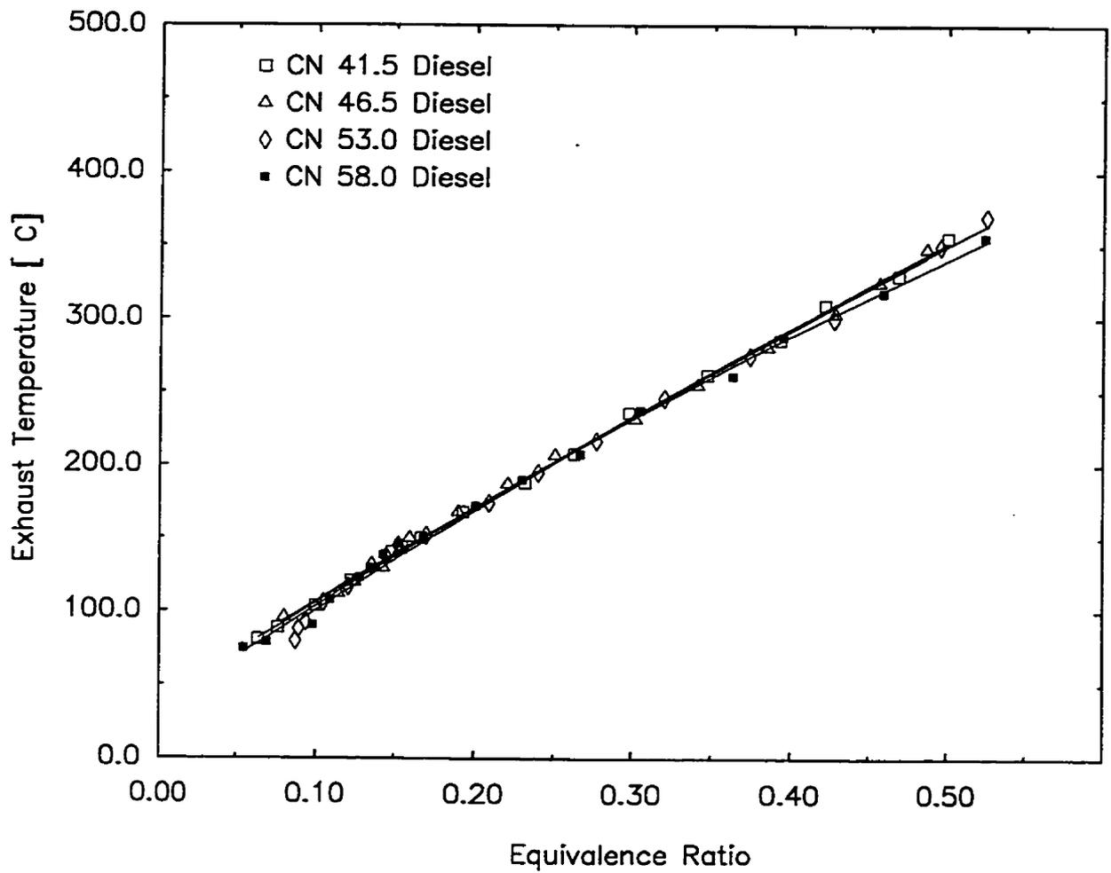
Figure 4.1.3. Variations of Exhaust Temperature with Equivalence Ratio for Diesel Operation when Using Different Cetane Number Fuels
