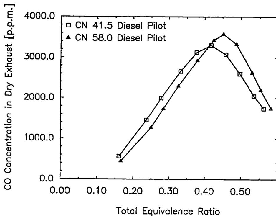
Figure 4.4.13 Variation of Dry Exhaust CO Concentration with Total Equivalence Ratio for Dual Fuel Operation with Methane when Using Different Cetane Number Fuels with a 0.40 kg/h Pilot
