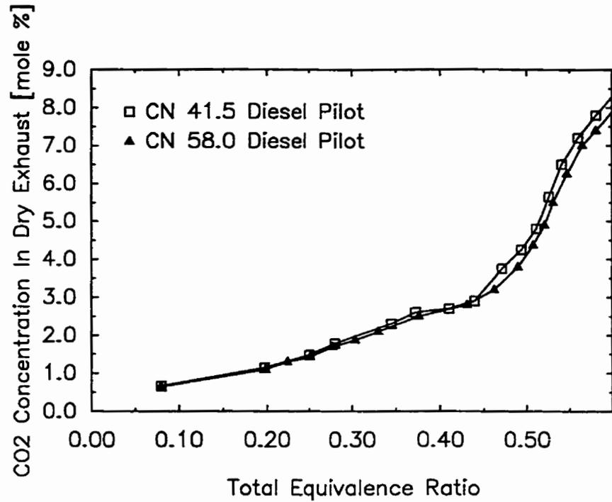
Figure F.1.17 Variation of Dry Exhaust CO<sub>2</sub> Concentration with Total Equivalence Ratio for Dual Fuel Operation with CH<sub>4</sub>-CO<sub>2</sub> Mixture (50% by Mass CH<sub>4</sub>) when Using Different Cetane Number Fuels with a 0.20 kg/h Pilot
