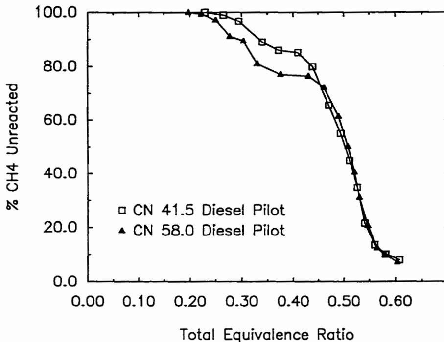
Figure 4.4.19 Variation of the Percent of CH<sub>4</sub> Unreacted with Total Equivalence Ratio for Dual Fuel Operation with a CH<sub>4</sub>-CO<sub>2</sub> Mixture (50% by Mass CH<sub>4</sub>) when Using Different Cetane Number Fuels with a 0.20 kg/h Pilot
