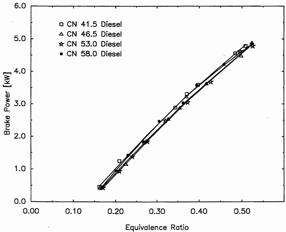
Figure 4.1.1. Variations of Brake Power with Equivalence Ratio for Diesel Operation when Using Different Cetane Number Fuels
