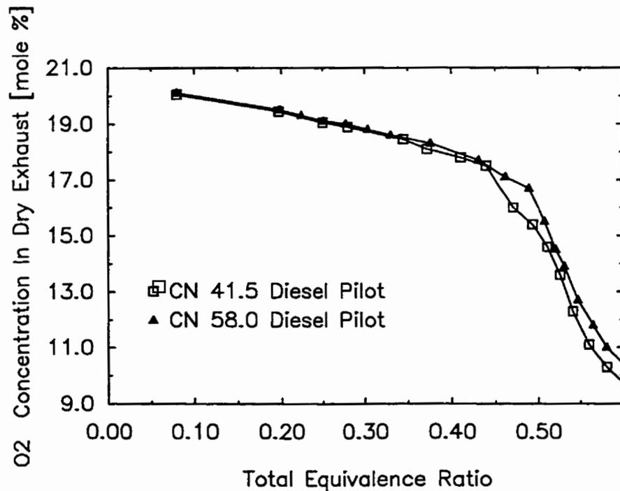
Figure F.1.18 Variation of Dry Exhaust O<sub>2</sub> Concentration with Total Equivalence Ratio for Dual Fuel Operation with CH<sub>4</sub>-CO<sub>2</sub> Mixture (50% by Mass CH<sub>4</sub>) when Using Different Cetane Number Fuels with a 0.20 kg/h Pilot
