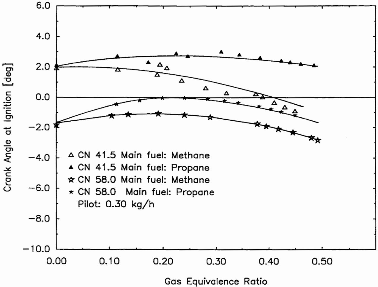
Figure F.1.2 Variations of the Point of Ignition with Gas Equivalence Ratio for Dual Fuel Operation with Propane when Using Different Cetane Number Fuels as Compared to the Corresponding Values Obtained when Operating with Methane.
