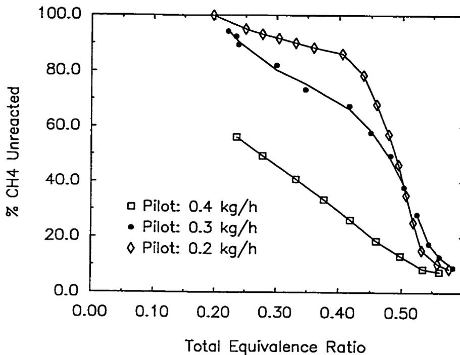
Figure 4.4.3 Variation of the Percent of CH4 Unreacted with Total Equivalence Ratio for Dual Fuel Operation with Methane when Using a 41.5 Cetane Number Fuel with Different Pilot Quantities
