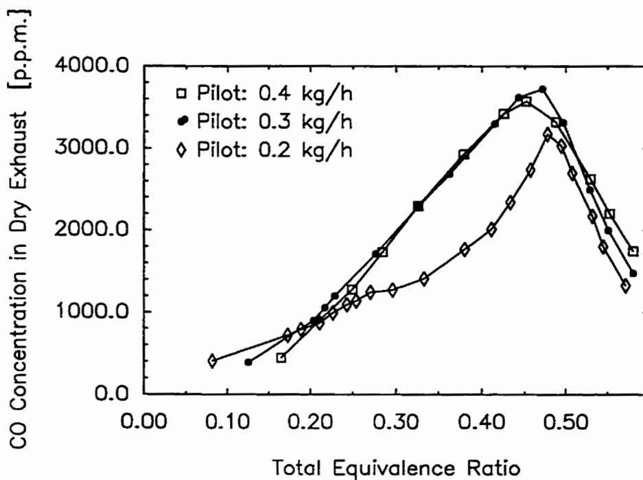
Figure F.1.4 Variations of Dry Exhaust CO Concentration with Total Equivalence Ratio for Dual Fuel Operation with Methane when Using a 58.0 Cetane Number Fuel with Different Pilot Quantities.
