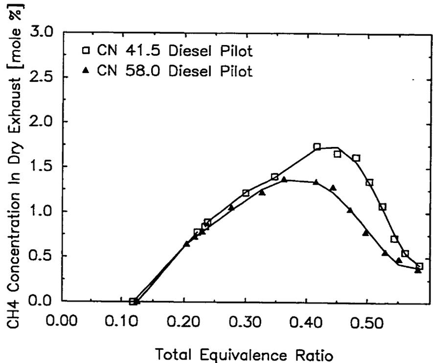
Figure 4.4.8 Variation of Dry Exhaust CH<sub>4</sub> Concentration with Total Equivalence Ratio for Dual Fuel Operation with Methane when Using Different Cetane Number Fuels with a 0.30 kg/h Pilot
