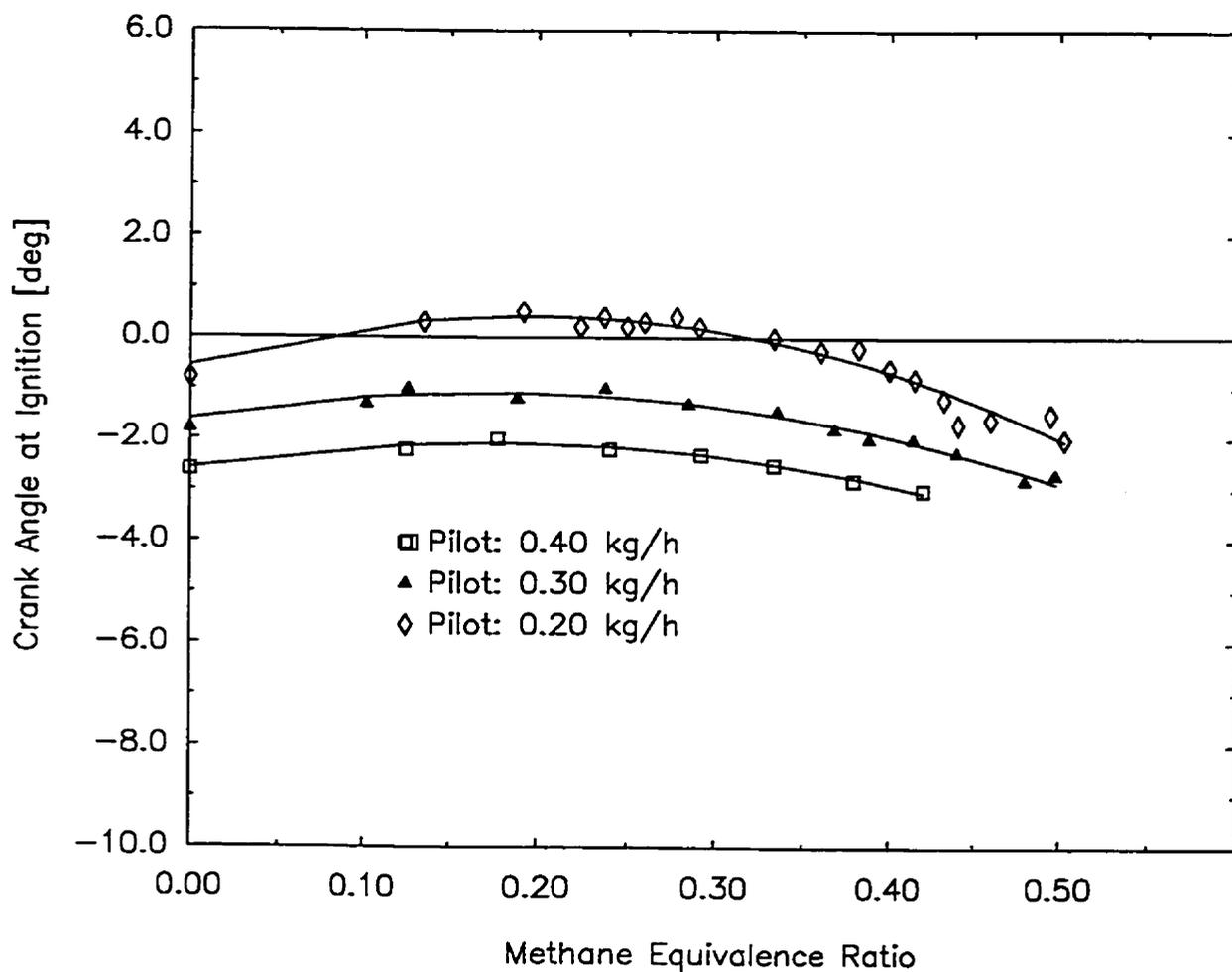
Figure F.1.3 Variations of the Point of Ignition with Gas Equivalence Ratio for Dual Fuel Operation with Methane when Using a 58.0 Cetane Number Fuel with Different Pilot Quantities.
