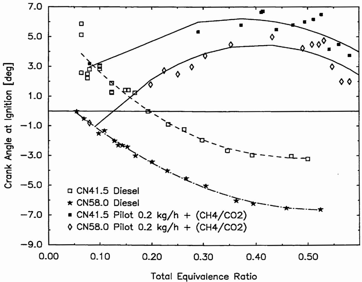
Figure 4.2.8 Variations of the Point of Ignition with Total Equivalence Ratio for Dual Fuel Operation when Using Different Cetane Number Fuels and Different Pilot Quantities with a CH<sub>4</sub>-CO<sub>2</sub> Mixture (50% by mass CH<sub>4</sub>)
