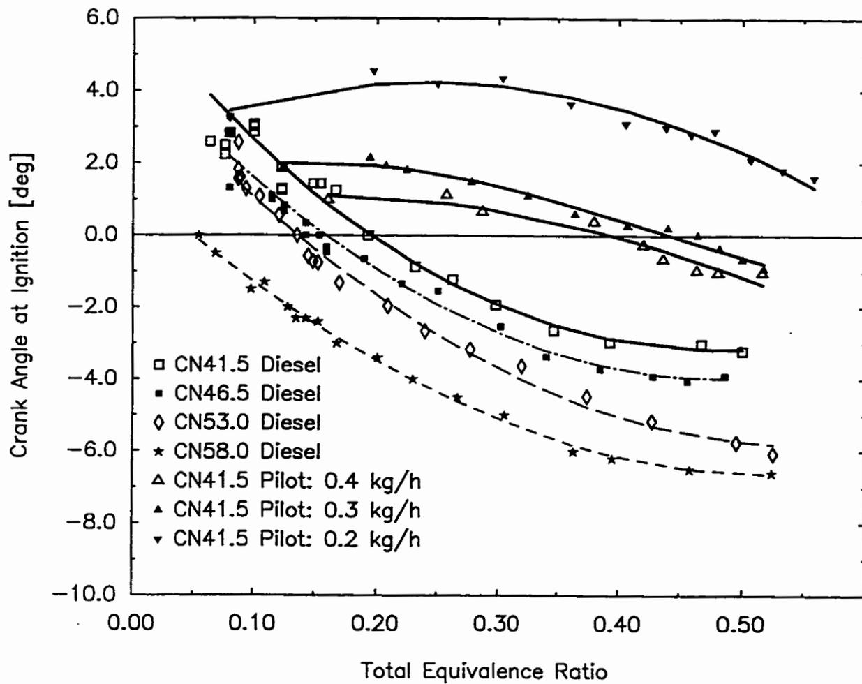
Figure 4.2.2 Variations of the Point of Ignition with Total Equivalence Ratio for Dual Fuel Operation with Methane when Using a 41.5 Cetane Number Fuel with Different Pilot Quantities
