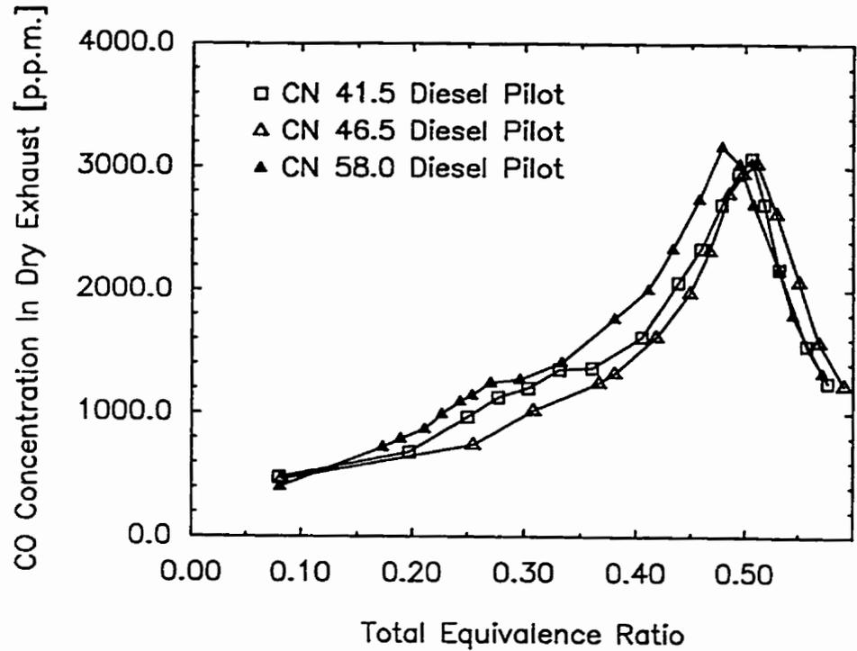
Figure 4.4.11 Variation of Dry Exhaust CO Concentration with Total Equivalence Ratio for Dual Fuel Operation with Methane when Using Different Cetane Number Fuels with a 0.20 kg/h Pilot
