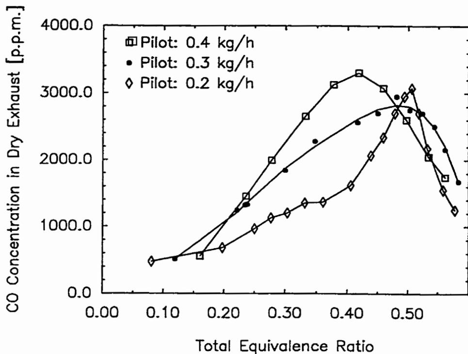
Figure 4.4.1 Variation of Dry Exhaust CO Concentration with Total Equivalence Ratio for Dual Fuel Operation with Methane when Using a 41.5 Cetane Number Fuel with Different Pilot Quantities
