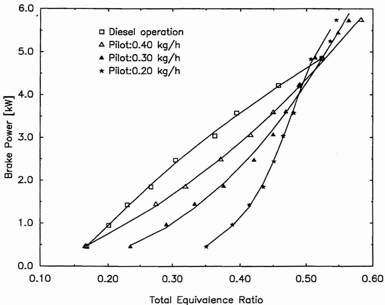
Figure 4.1.4. Variations of Brake Power with Total Equivalence Ratio for Dual Fuel Operation with Methane when Using a 58.0 Cetane Number Diesel Fuel and Different Pilot Quantities. ( $\phi_D=0.166$  for 0.40 kg/h Pilot;  $\phi_D=0.123$  for 0.30 kg/h Pilot;  $\phi_D=0.081$  for 0.20 kg/h Pilot)
