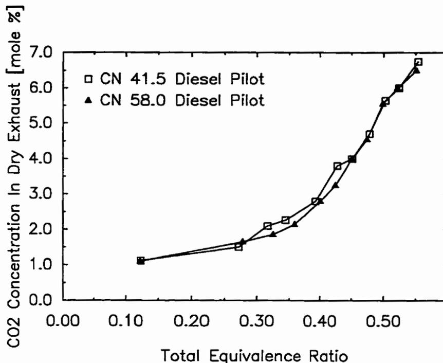
Figure F.1.15 Variation of Dry Exhaust CO<sub>2</sub> Concentration with Total Equivalence Ratio for Dual Fuel Operation with Propane when Using Different Cetane Number Fuels with a 0.30 kg/h Pilot
