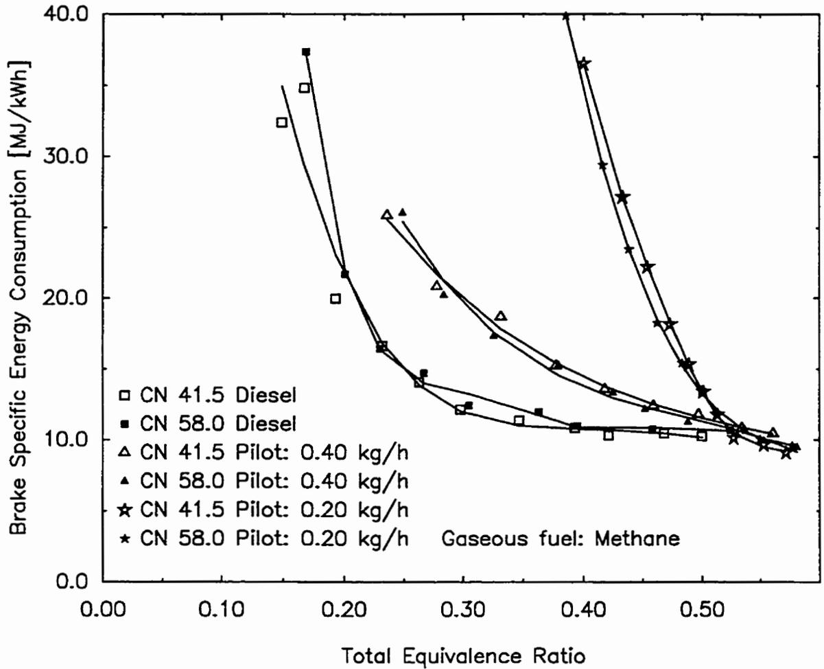
Figure 4.1.5. Variations of Brake Specific Energy Consumption with Total Equivalence Ratio for Dual Fuel Operation with Methane when Using Different Cetane Number Diesel Fuels and Different Pilot Quantities. ( $\phi_D=0.166$  for 0.40 kg/h Pilot;  $\phi_D=0.081$  for 0.20 kg/h Pilot)
