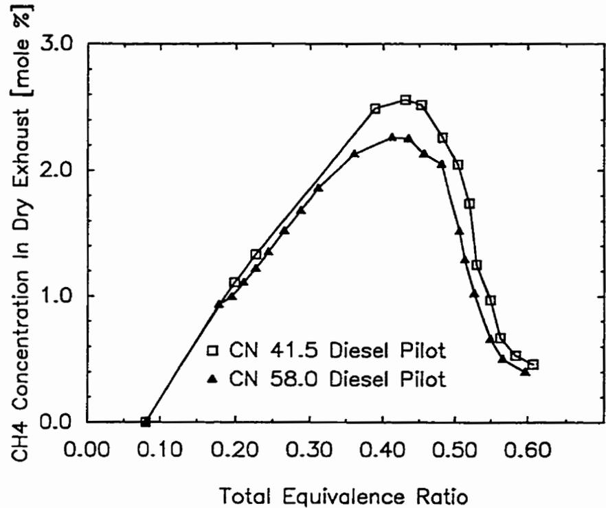
Figure 4.4.15 Variation of Dry Exhaust CH<sub>4</sub> Concentration with Total Equivalence Ratio for Dual Fuel Operation with a CH<sub>4</sub>-N<sub>2</sub> Mixture (50% by Mass CH<sub>4</sub>) when Using Different Cetane Number Fuels with a 0.20 kg/h Pilot
