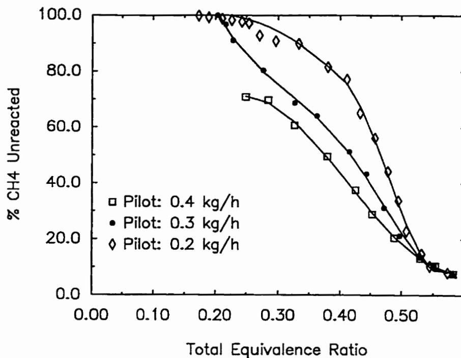
Figure 4.4.5 Variation of the Percent of CH<sub>4</sub> Unreacted with Total Equivalence Ratio for Dual Fuel Operation with Methane when Using a 58.0 Cetane Number Fuel with Different Pilot Quantities
