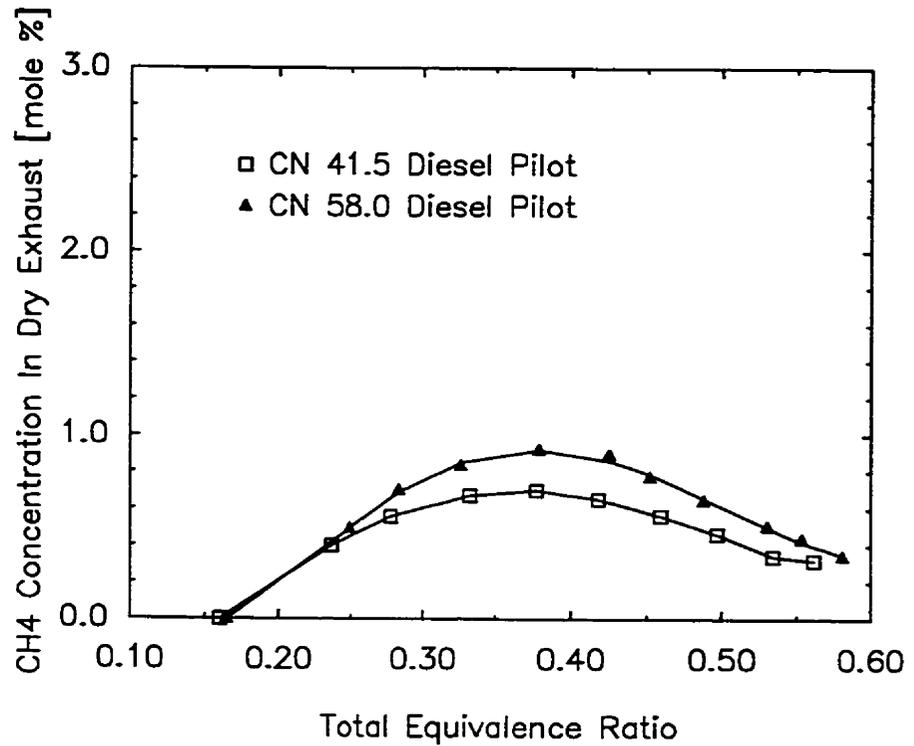
Figure 4.4.9 Variation of Dry Exhaust CH<sub>4</sub> Concentration with Total Equivalence Ratio for Dual Fuel Operation with Methane when Using Different Cetane Number Fuels with a 0.40 kg/h Pilot
