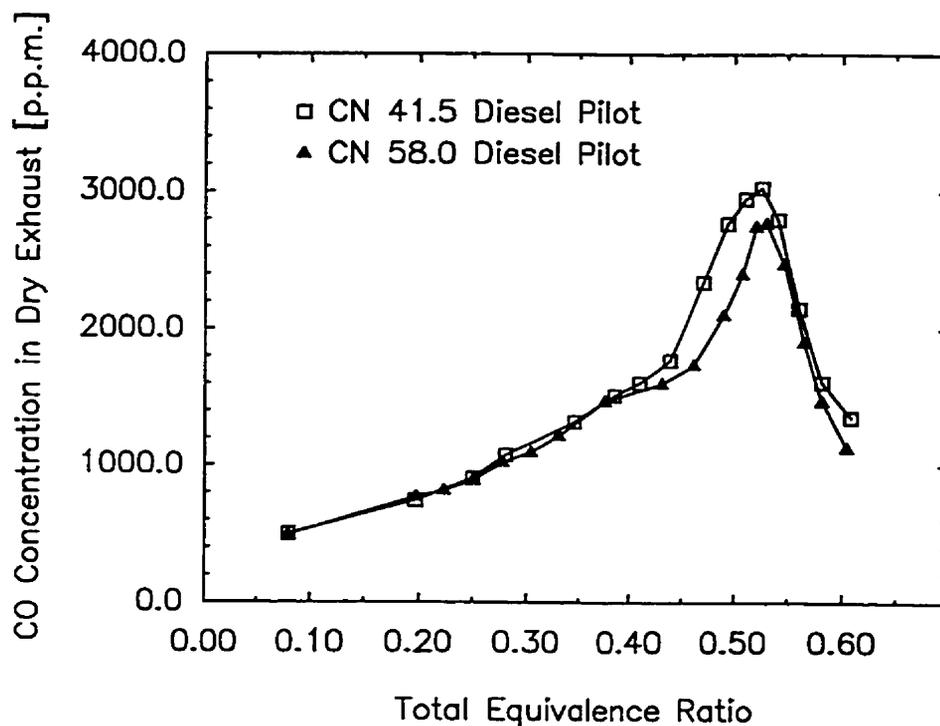
Figure 4.4.17 Variation of Dry Exhaust CO Concentration with Total Equivalence Ratio for Dual Fuel Operation with a CH<sub>4</sub>-CO<sub>2</sub> Mixture (50% by Mass CH<sub>4</sub>) when Using Different Cetane Number Fuels with a 0.20 kg/h Pilot
