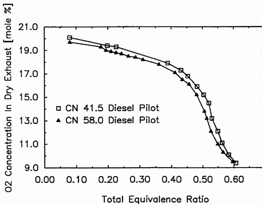
Figure F.1.14 Variation of Dry Exhaust O<sub>2</sub> Concentration with Total Equivalence Ratio for Dual Fuel Operation with CH<sub>4</sub>-N<sub>2</sub> Mixture (50% by Mass CH<sub>4</sub>) when Using Different Cetane Number Fuels with a 0.20 kg/h Pilot
