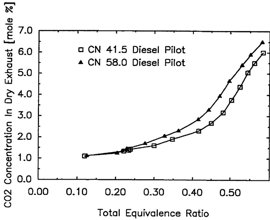
Figure F.1.7 Variation of Dry Exhaust CO<sub>2</sub> Concentration with Total Equivalence Ratio for Dual Fuel Operation with Methane when Using Different Cetane Number Fuels with a 0.30 kg/h Pilot
