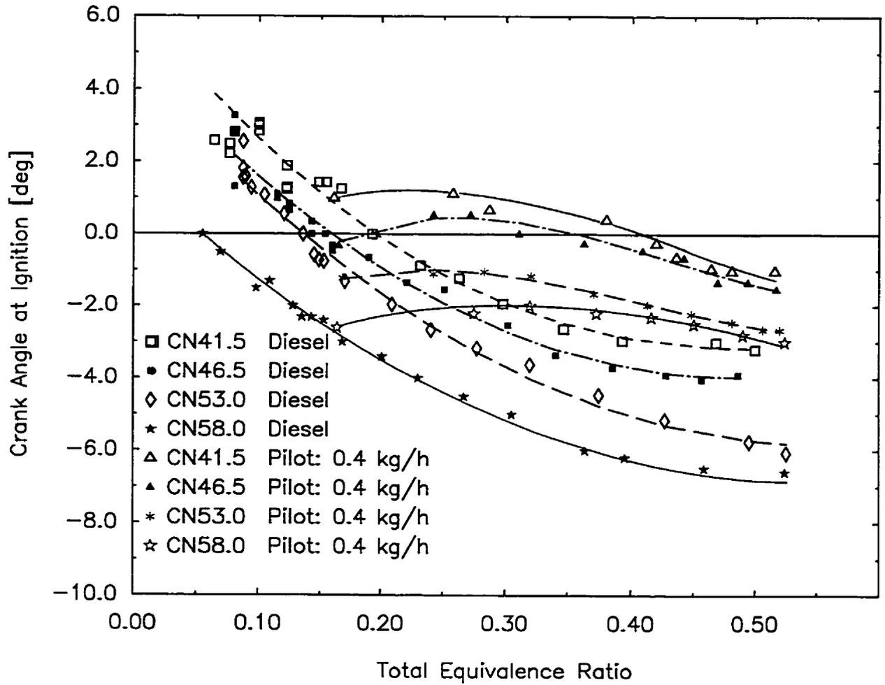
Figure 4.2.3 Variations of the Point of Ignition with Total Equivalence Ratio for Dual Fuel Operation with Methane when Using Different Cetane Number Fuels with a 0.40 kg/h Pilot
