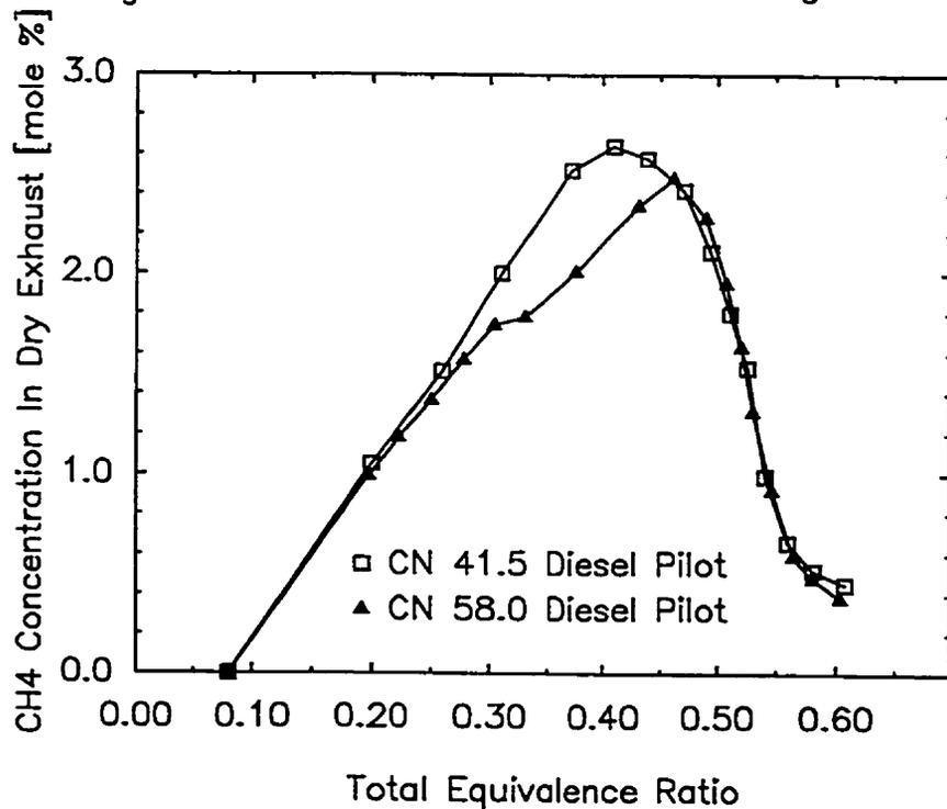
Figure 4.4.18 Variation of Dry Exhaust CH<sub>4</sub> Concentration with Total Equivalence Ratio for Dual Fuel Operation with a CH<sub>4</sub>-CO<sub>2</sub> Mixture (50% by Mass CH<sub>4</sub>) when Using Different Cetane Number Fuels with a 0.20 kg/h Pilot
