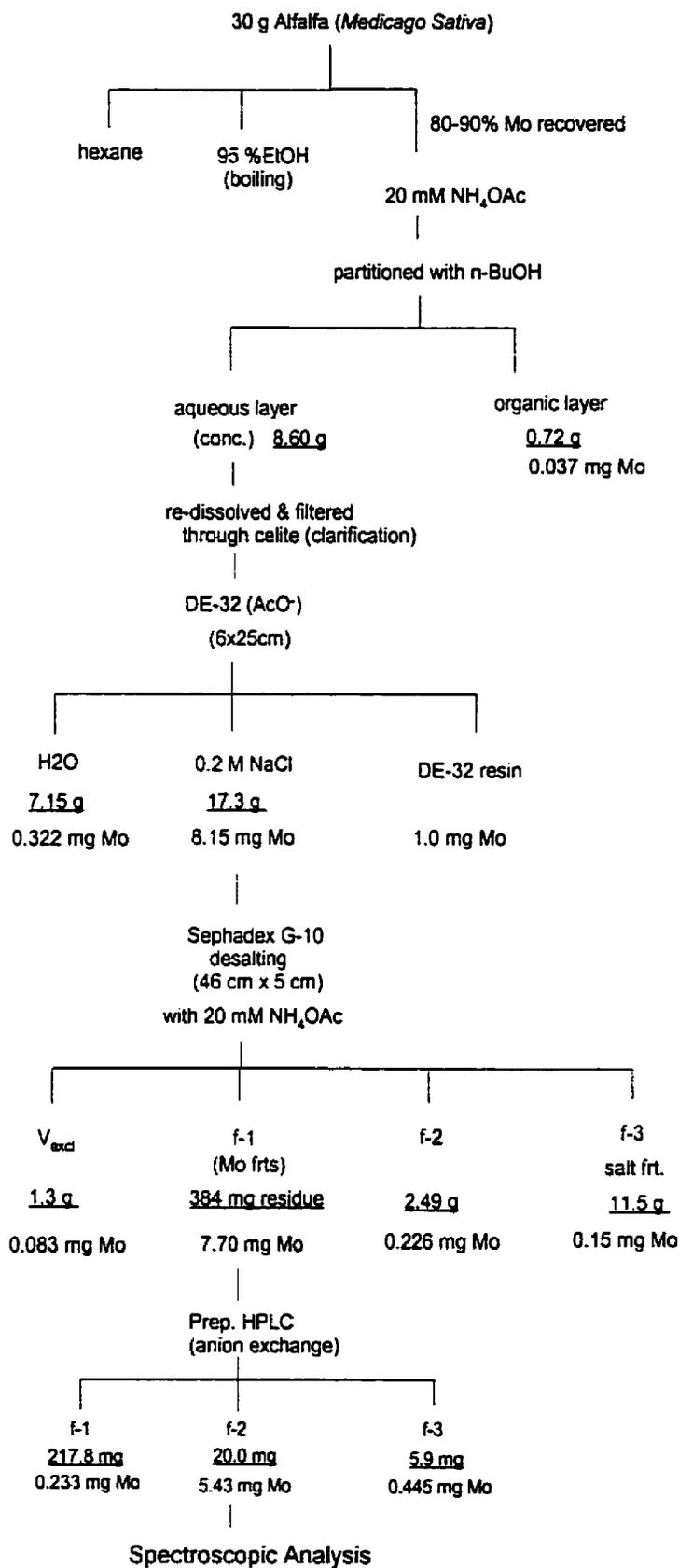
**Figure 3.1** Optimized purification procedure for Mo from alfalfa
