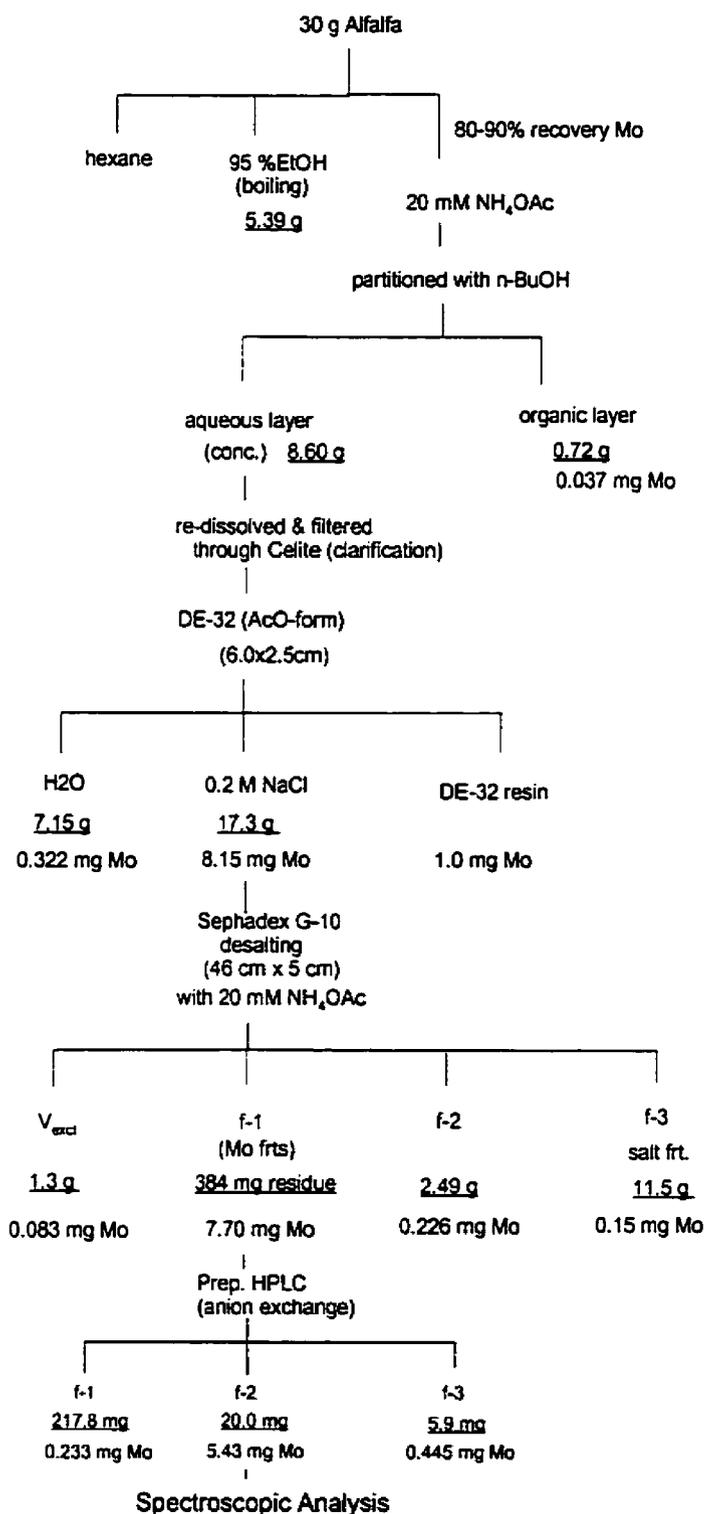
Figure 2.8 Modified purification procedure for Mo in alfalfa
