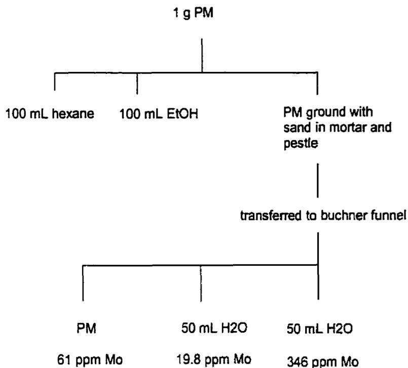
**Figure 2.1** Modified extraction protocol for Mo in alfalfa
