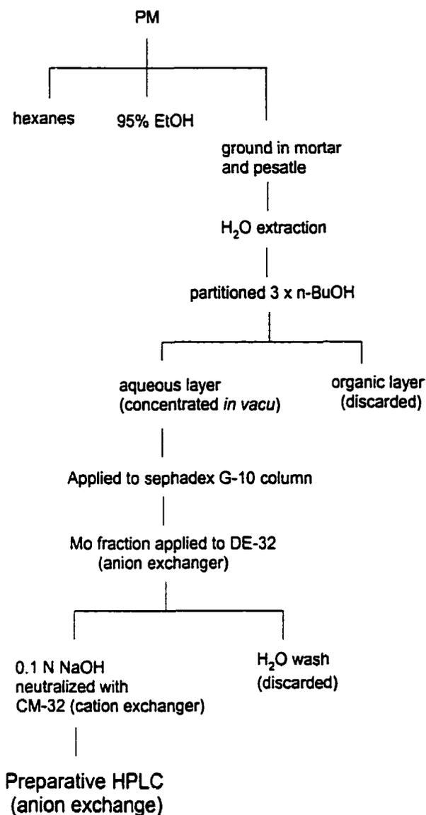
**Figure 2.6** Initial purification sequence for Mo from alfalfa
