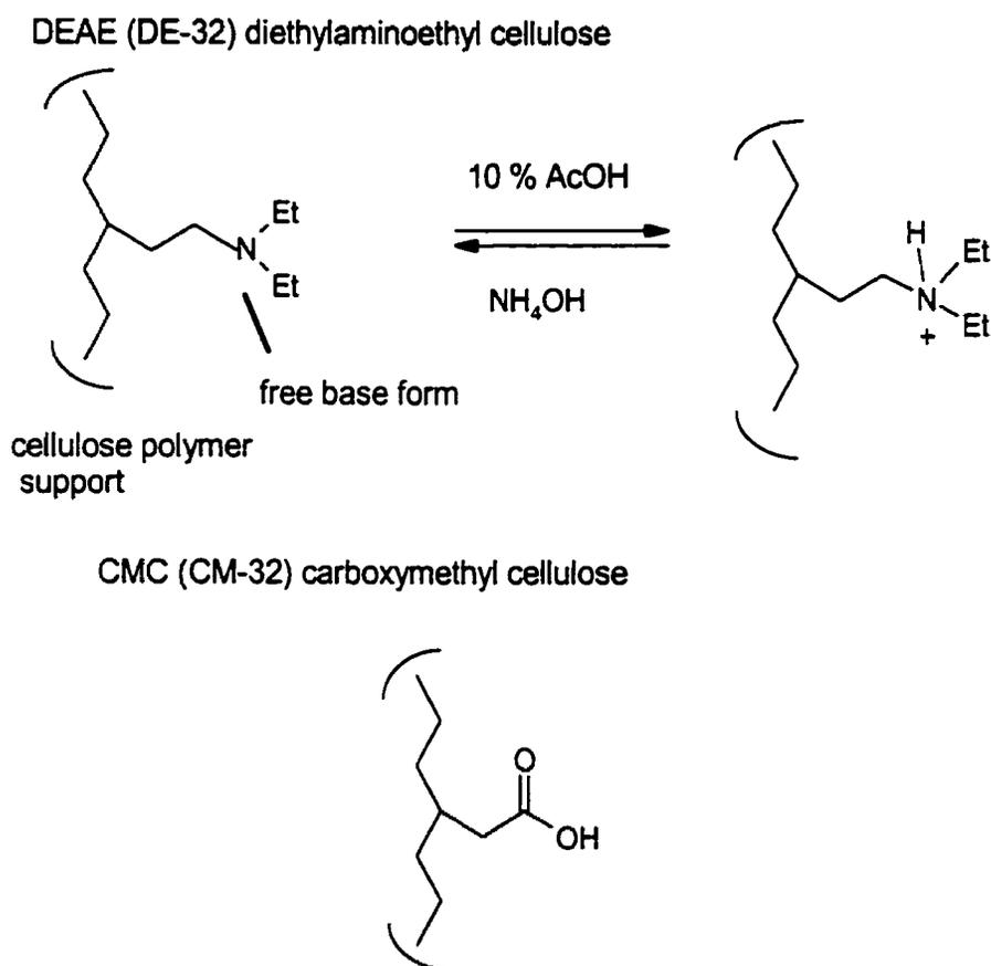
**Figure 2.3** Functional sites of ion exchange resins used
