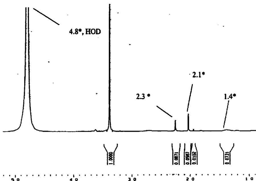
**Figure 2.11** Quantitative  $^1\text{H}$  NMR of purified Mo species, chemical shifts given in ppm (\*), integration values shown above ppm scale
