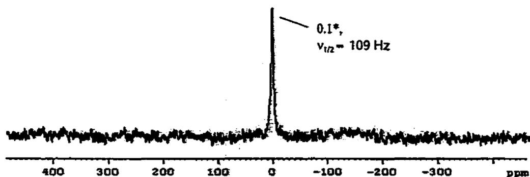
**Figure 2.10**  $^{95}\text{Mo}$  NMR spectrum of the purified Mo species, chemical shift in ppm(\*)
