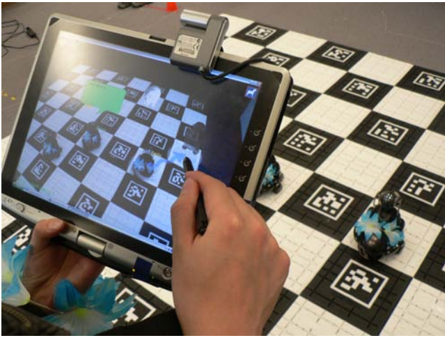
Figure 2: Human player interacting with robot teammates using a handheld mixed reality interface
