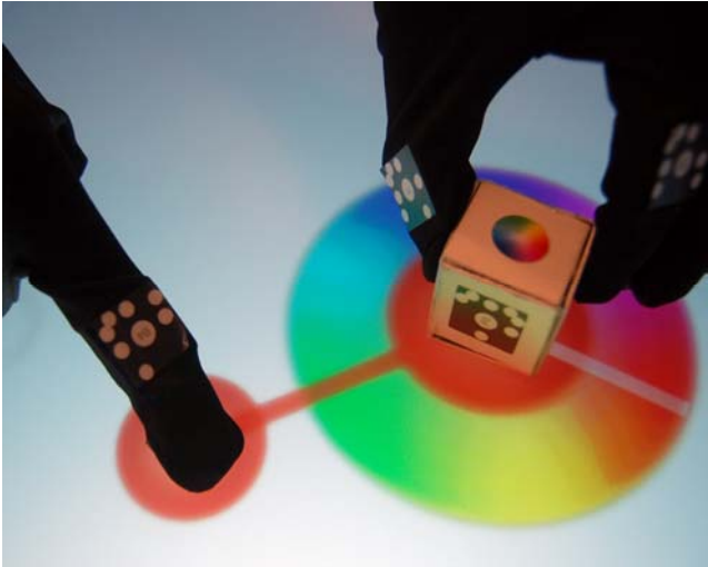
Figure 6. Calibrating a finger's color with a tangible object.
