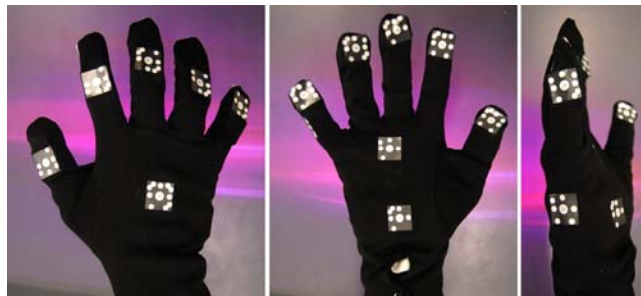
Figure 1. The fiduciary-tagged glove (top, bottom, side)
