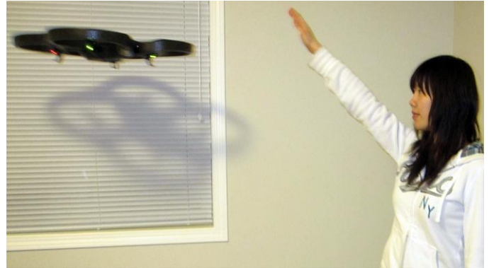
Figure 1. Using a gesture to tell the A.R. Drone to fly higher.
