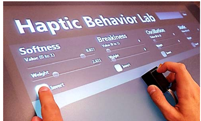
Figure 1. Behavior Lab lets developers explore, combine and feel diverse haptic behaviors before writing code.
