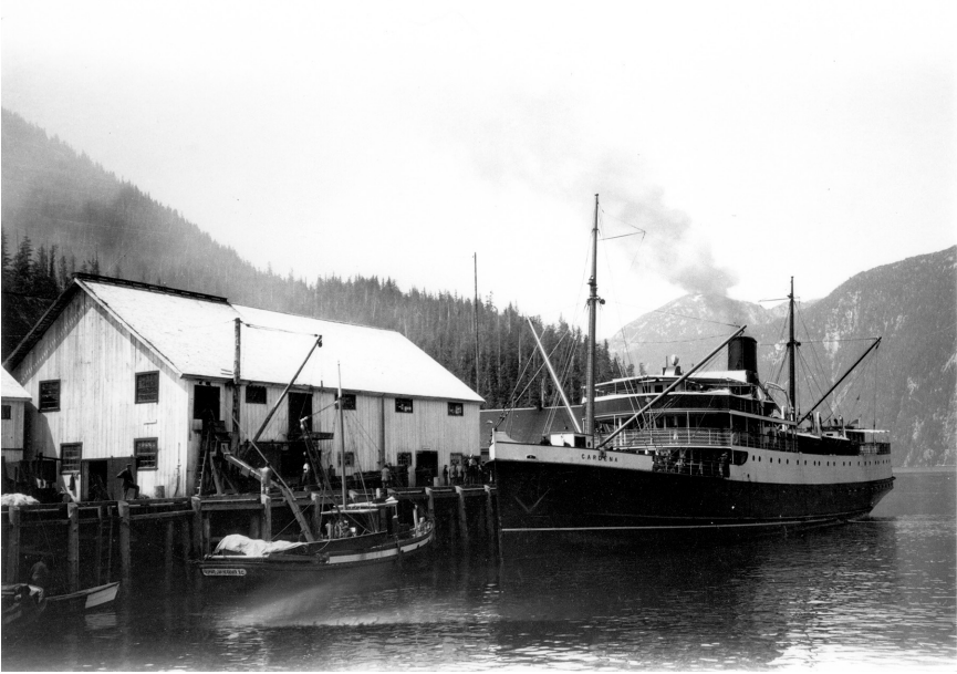
FIGURE 8.3. The S.S. Cardena , seen here at the Butedale salmon cannery (c. 1935), had a 350-ton cargo capacity, had refrigeration for thirty tons of boxed fish, and could carry eleven thousand cases of canned salmon. It was also licensed to carry 250 passengers. Courtesy of City of Vancouver Archives.
