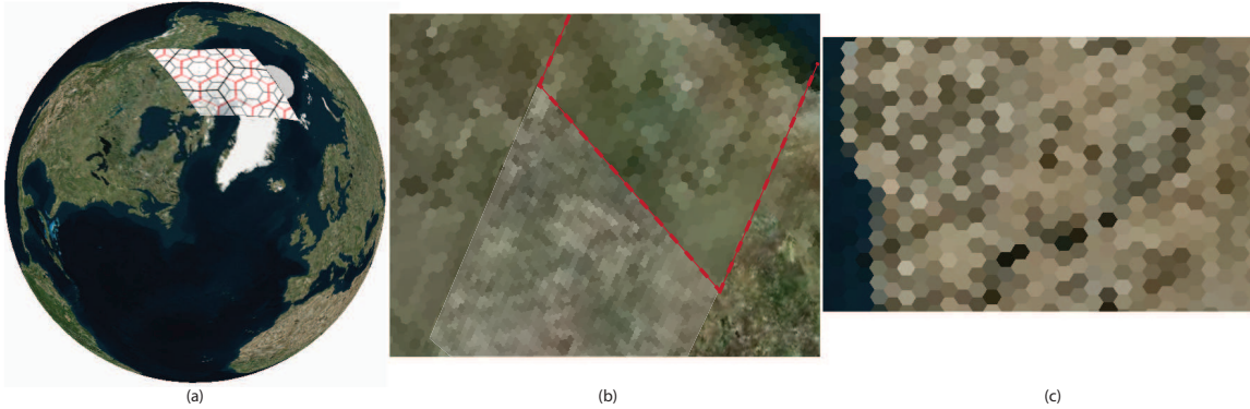
Figure 4: (a) A textured globe using diamonds. One of the diamonds has been textured differently to show the formation of diamonds. (b) Two textured diamonds beside each other. Red lines highlight the boundary of the two diamonds. (c) A close up look of the hexagonal sampling of textures.
