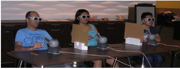
Figure 5: Corresponding placement between three Omni devices and three participants in the collaborative VE of the experiment.
