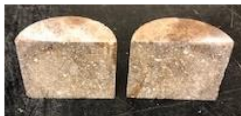
Top (A) – Core Plug #7. Located between TC 6 and 7. Second (B) – Core Plug #9. Located between TC 9 and 10. Third (C) – Core Plug #11. Located between TC 19 and 20. Bottom (D) – Core Plug #16. Located between TC 28 and 29. Photo 7. Core Plugs after Combustion Test Two, Prior to Extraction.
