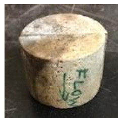
Top (A) – Core Plug #7. Located between TC 6 and 7. Second (B) – Core Plug #9. Located between TC 9 and 10. Third (C) – Core Plug #11. Located between TC 19 and 20. Bottom (D) – Core Plug #16. Located between TC 28 and 29. Photo 7. Core Plugs after Combustion Test Two, Prior to Extraction.
