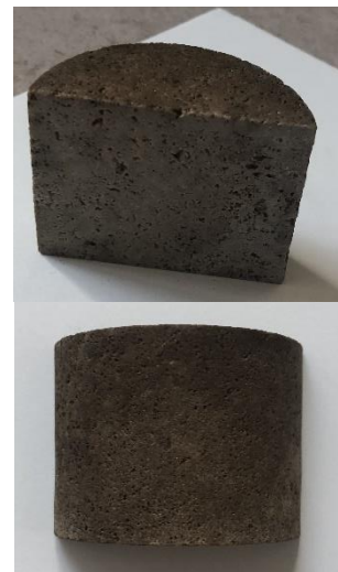
Left – Core Plug #1. Located between TC 6 and 7. Middle – Core Plug #6. Located at TC 22, which was drilled in the center to introduce the TC. Right – Core Plug #7a. Located between TC 29 and 30.
