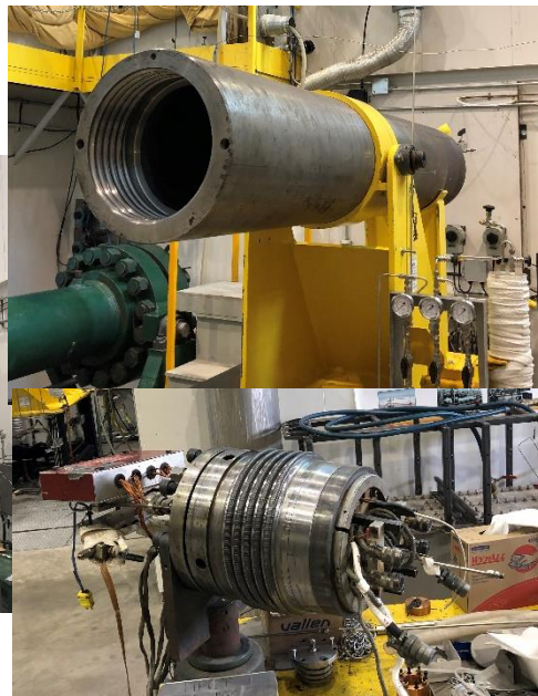
Photo 2. High Pressure Combustion Tube's jacket with production system in the background (left photo) and jacket cap with flanges (right bottom).
