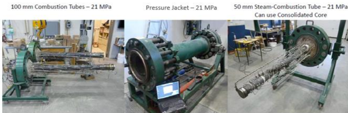
Figure 2.11 Combustion Tube for 21 MPa Tests (Mehta et. al 2018)
