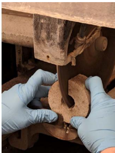
Photo 6. Core Plug #4 After Test One. Being Cut Dry Prior Extraction
