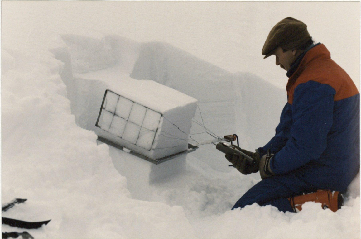
Figure 3.2: Tensile Test on an 18^\circ Slope
