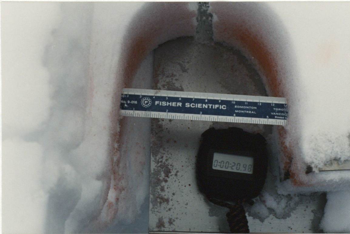
Figure 5.7: Displacement of Snow Block and Fracture Surfaces
