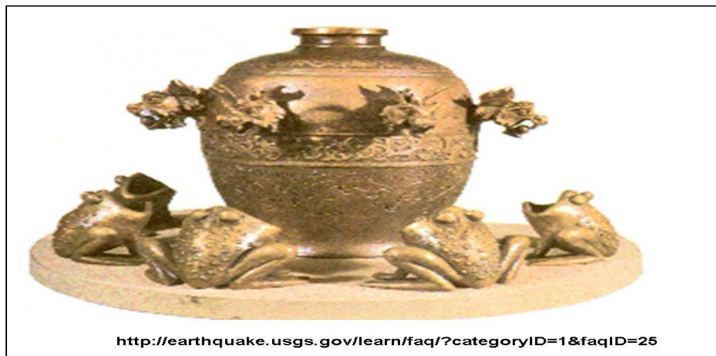
Figure 1.1: The earliest known mechanical seismoscope, built by a Chinese astronomer in 132 A.D.
