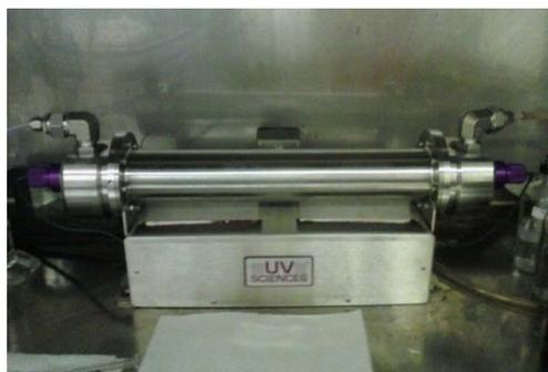
Figure 3.1. Photoreactor
