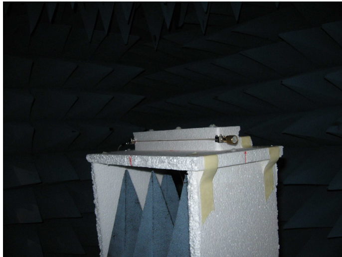
Figure 5.9: The non-inverting element antenna mounted for E-plane measurement in the anechoic chamber
