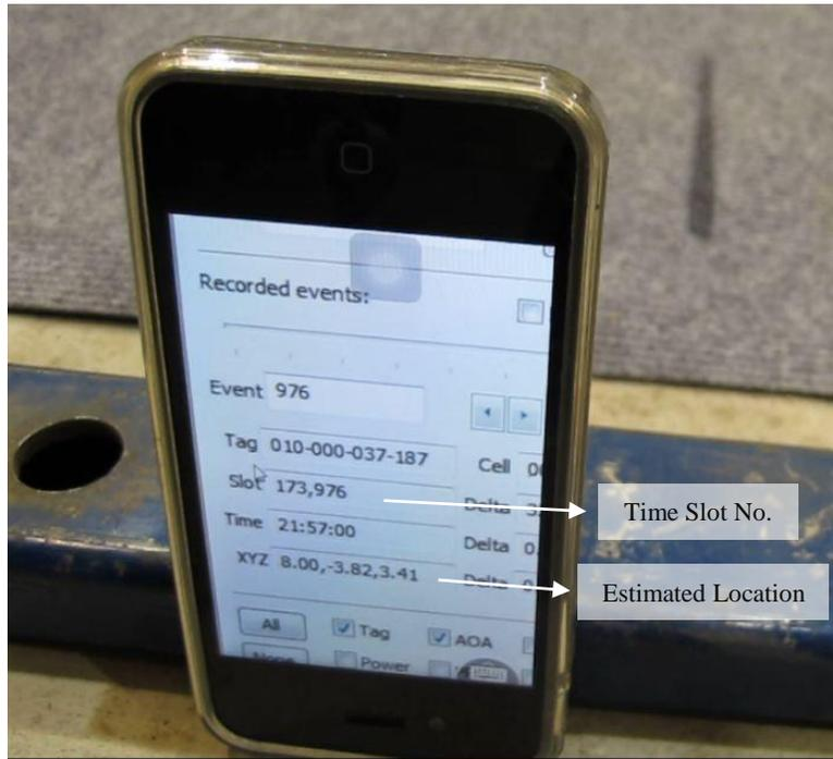
Figure 3.8 Mobile device (cell phone) showing the UWB hub display
