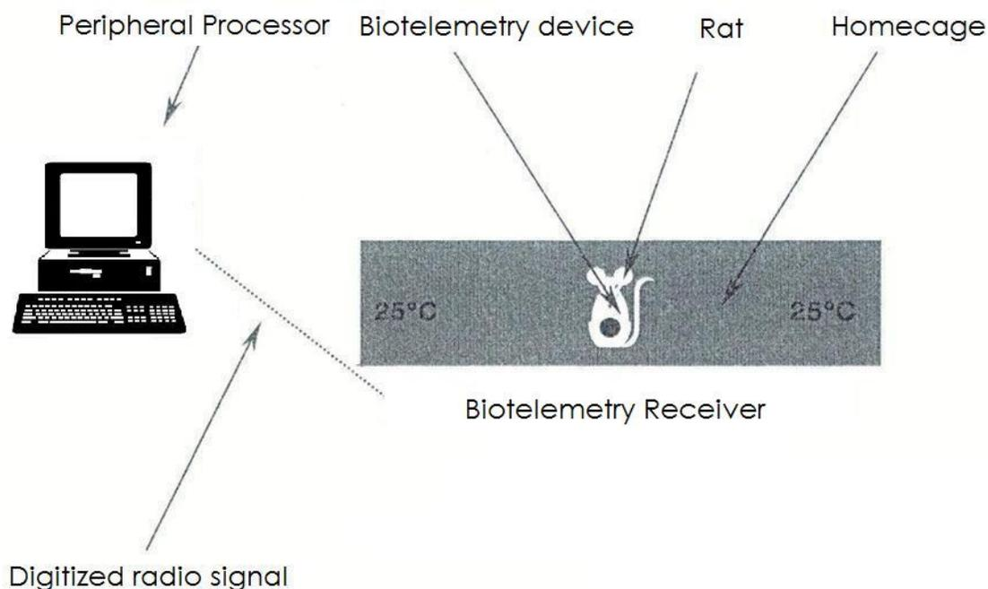
**Figure 2-1: Diagram showing the experimental set-up for core temperature transmission and recording from chronically instrumented rat inside its cage. Adapted from Fofie (59).**
