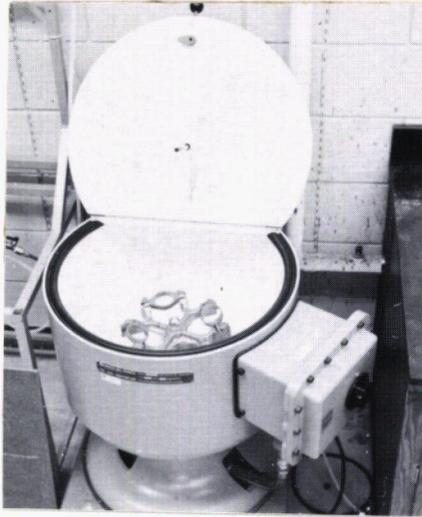
Figure 11: Photograph of Centrifuging Test Apparatus (IEC Model K)
