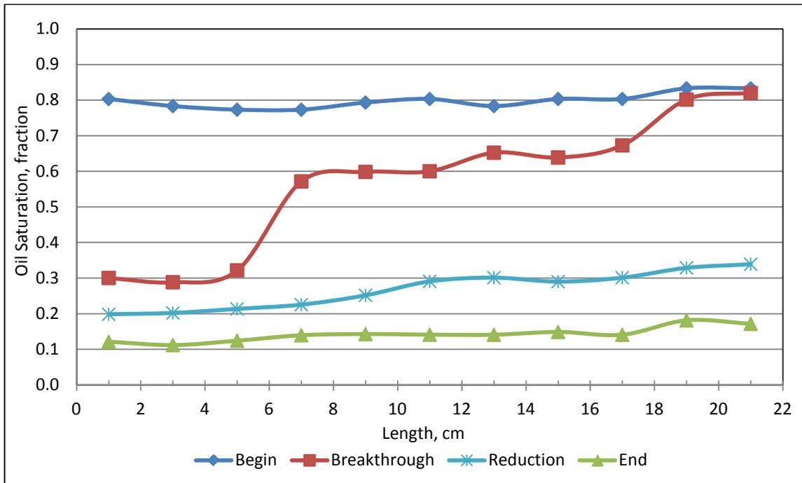
**Figure 4.19: Oil saturation profiles during waterflooding for A5-1000-10**
