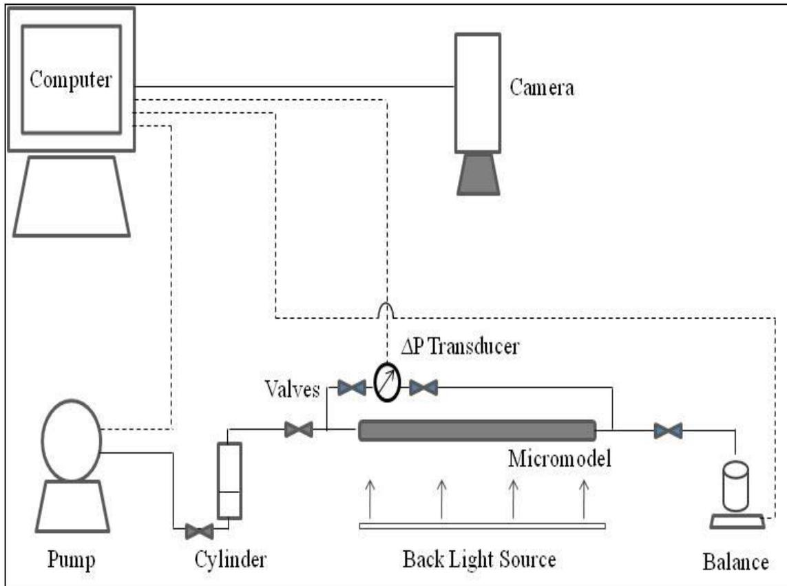
**Figure 3.5: Schematic of the experiment (forced imbibition)**
