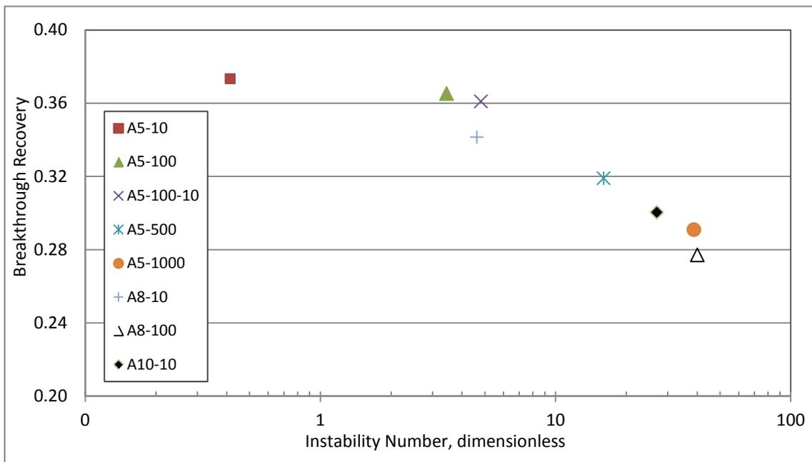
**Figure 5.1: Breakthrough recoveries as a function of instability number**
