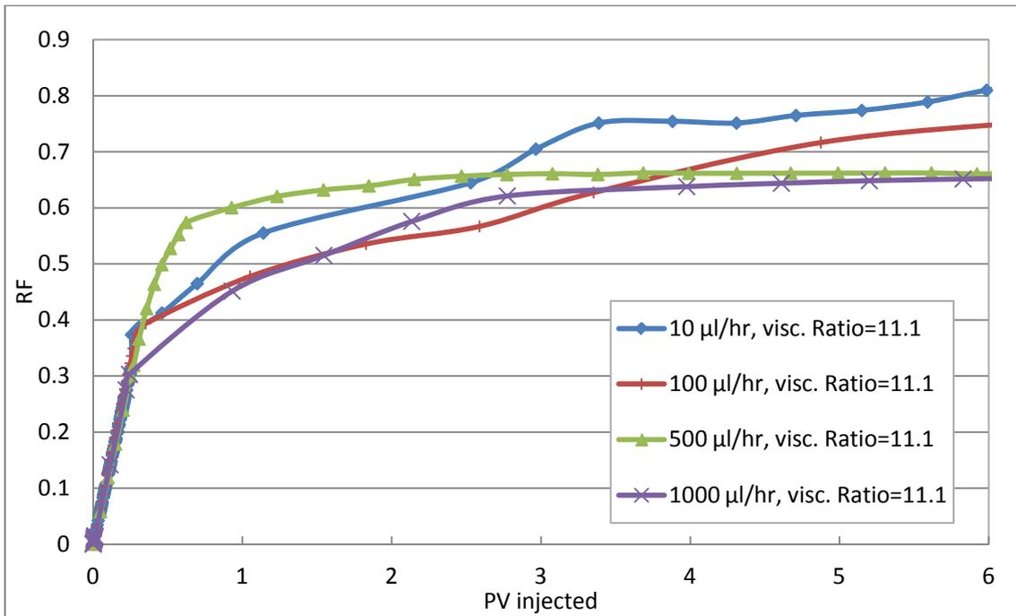
Figure 4.37: Recovery factors at different water injection rate
