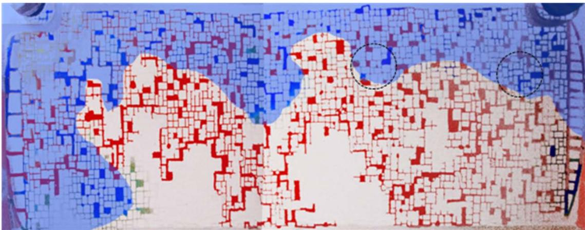
\*In this figure, the micromodel was first saturated with colourless distilled water. The water which was used for displacing oil was dyed blue. The green area ahead of water front was where dye diffused. The inlet is located at left side.
