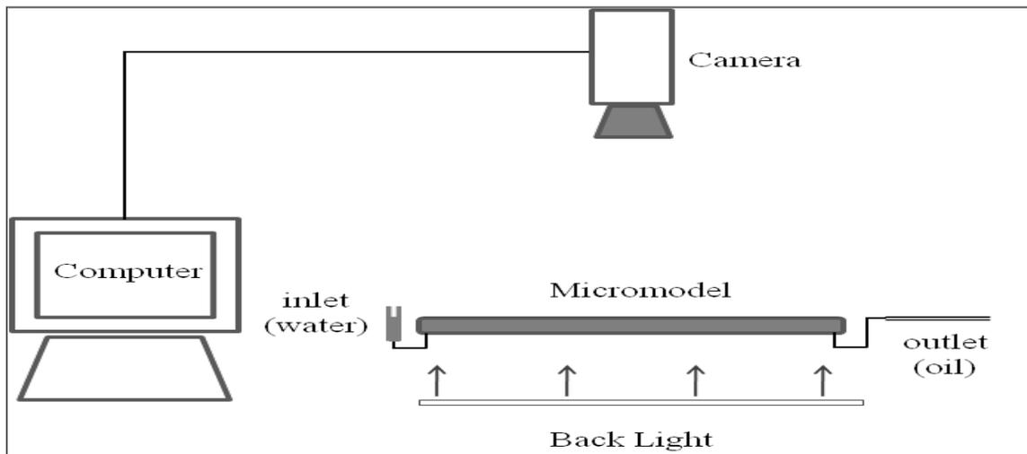
**Figure 3.8: Schematic of the experiment (spontaneous imbibition)**
