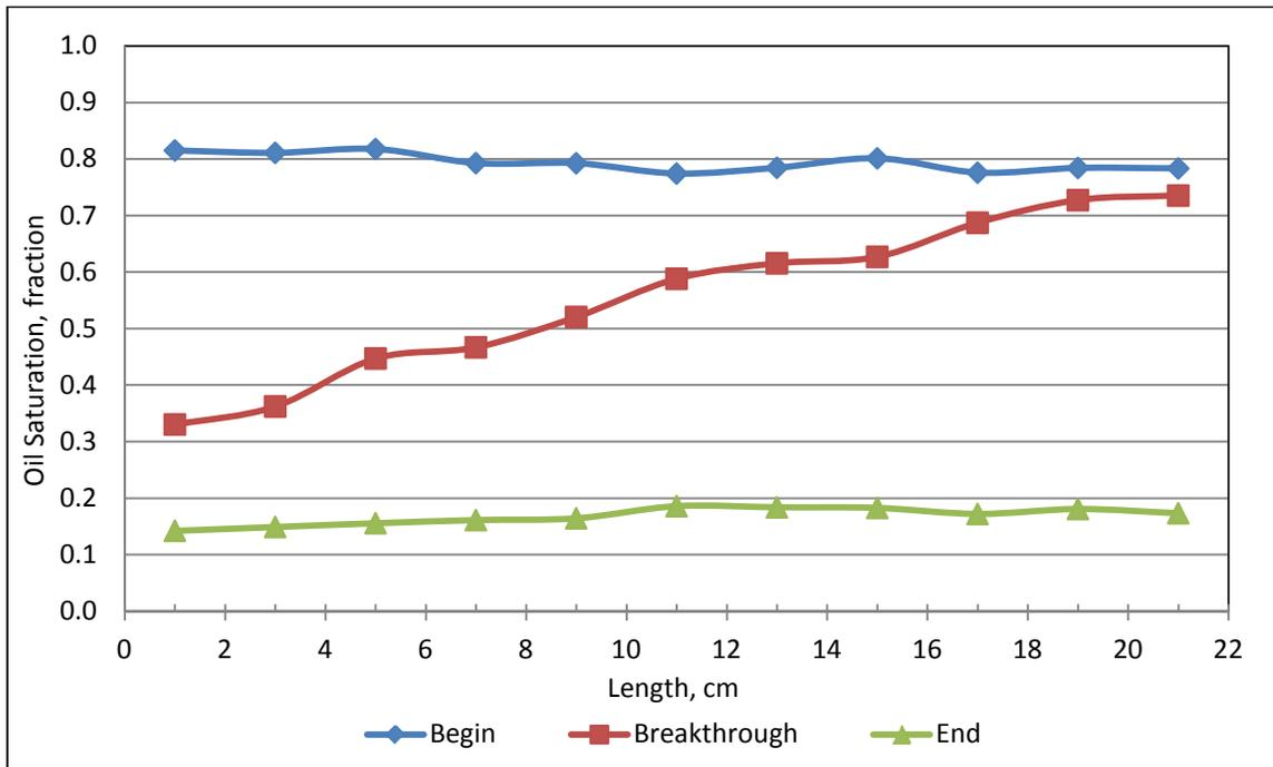
**Figure 4.31: Oil saturation profiles during waterflooding for A10-10**
