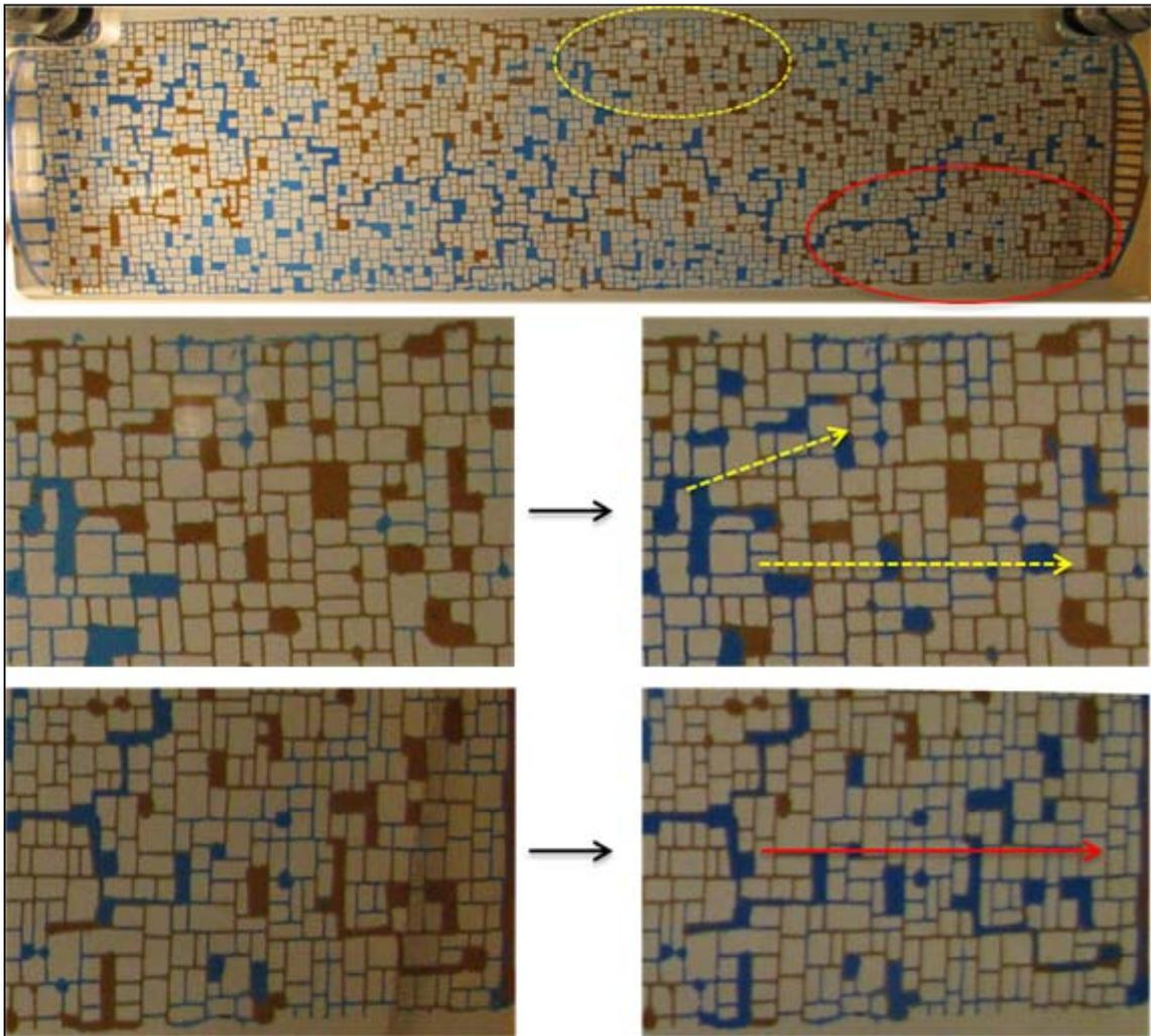
**Figure 4.43: Direction of imbibition after water breakthrough for A5-500**
