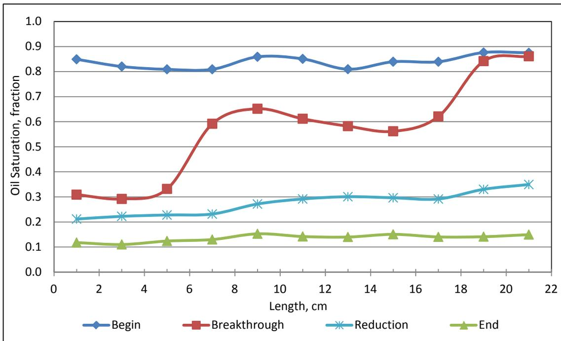
Figure 4.15: Oil saturation profiles during waterflooding for A5-500-10
