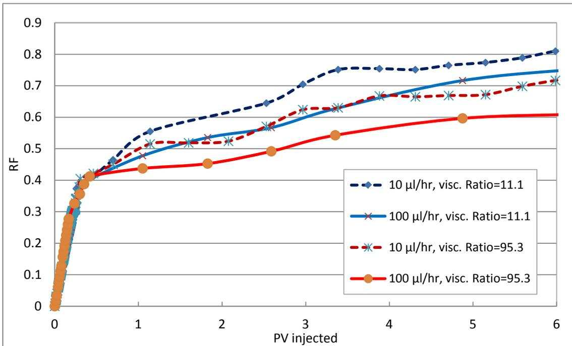
Figure 4.38: Recovery factors of low injection rate cases
