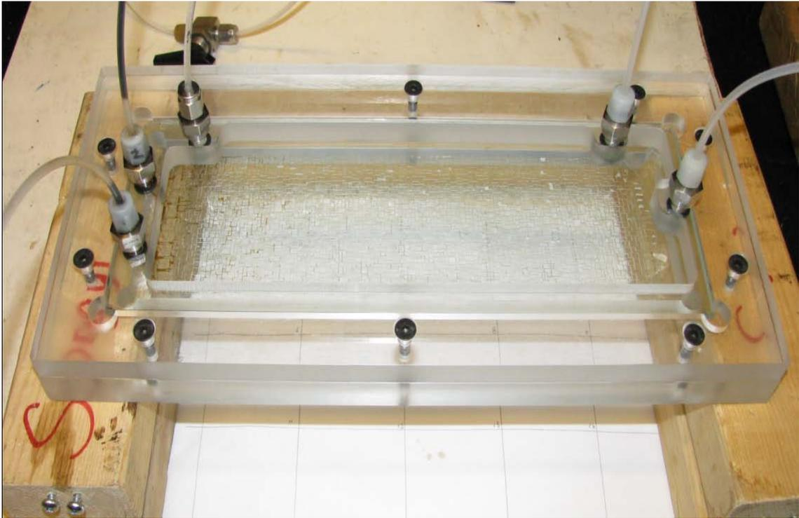
**Figure 3.6: Micromodel assembly (forced imbibition)**
