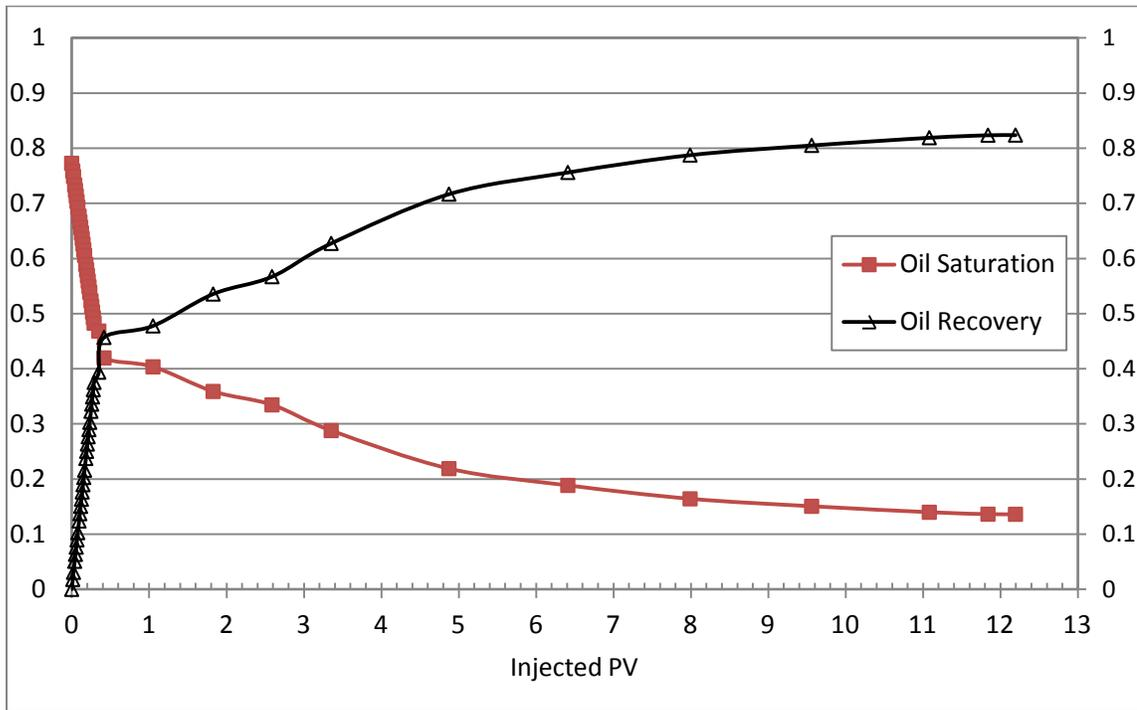
Figure 4.7: Recovery vs. PVs of water injected for A5-100
