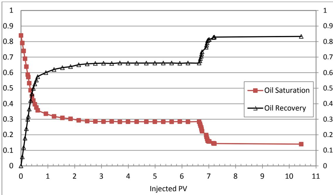
Figure 4.14: Recovery vs. PVs of water injected for A5-500-10
