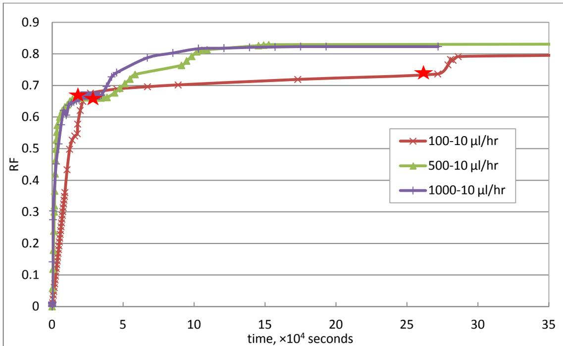
**Figure 4.40: Production responses after switching to low injection rate**
