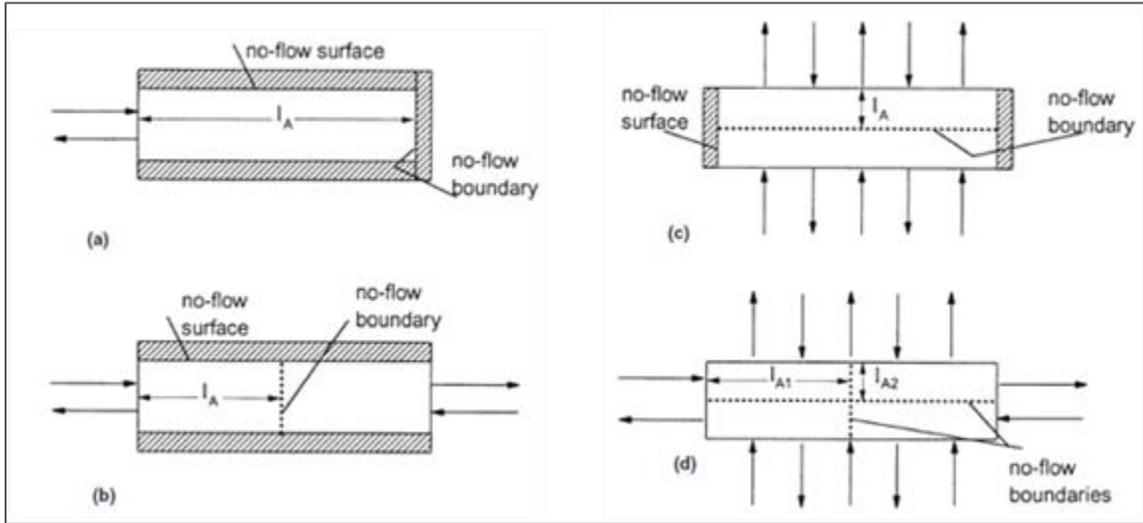
(a) OEO-one end open, 1D linear counter-current imbibition. (b) TEO-two end open, 1D linear counter-current imbibition. (c) TEC-two end closed, radial counter-current imbibition. (d) AFO-all faces open, 3D counter-current imbibition (Zhang et al., 1996; Ma et al., 1997).
