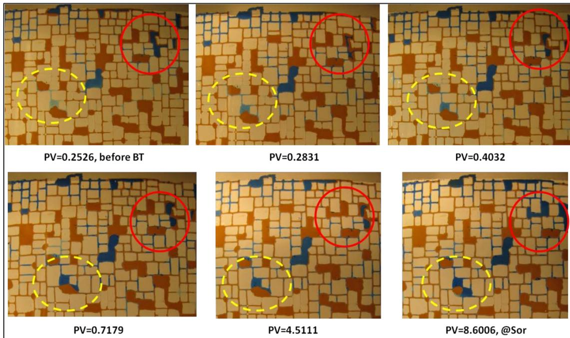
**Figure 4.44: Schematic of film thickening, snap-off and oil refilling**
