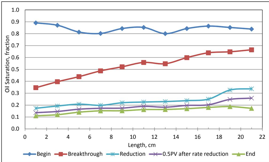
**Figure 4.12: Oil saturation profiles during waterflooding for A5-100-10**
