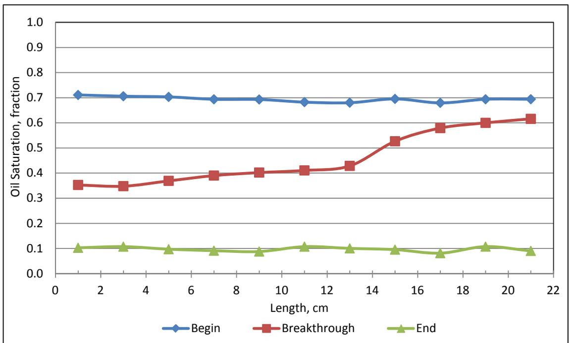
Figure 4.23: Oil saturation profiles during waterflooding for A8-10
