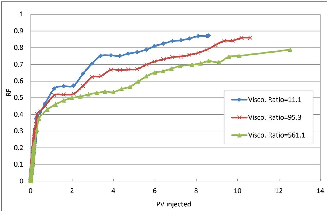
**Figure 4.35: Recovery factor vs. PVs injected**
