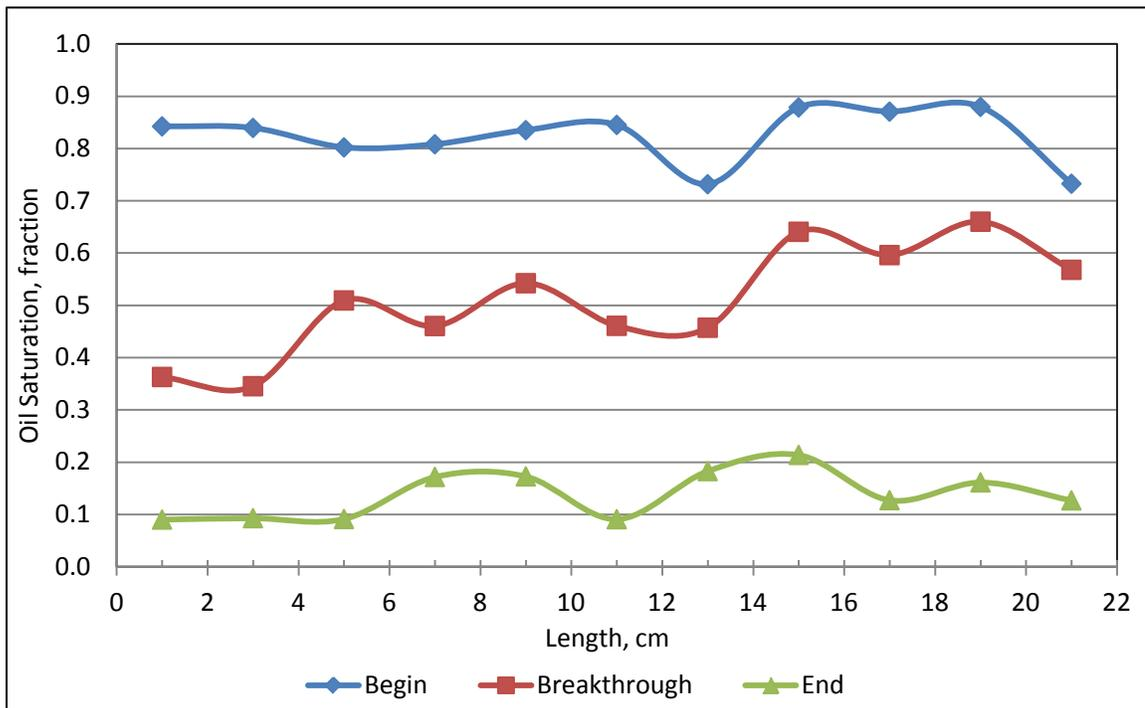
**Figure 4.3: Oil saturation profiles during waterflooding for A5-10**
