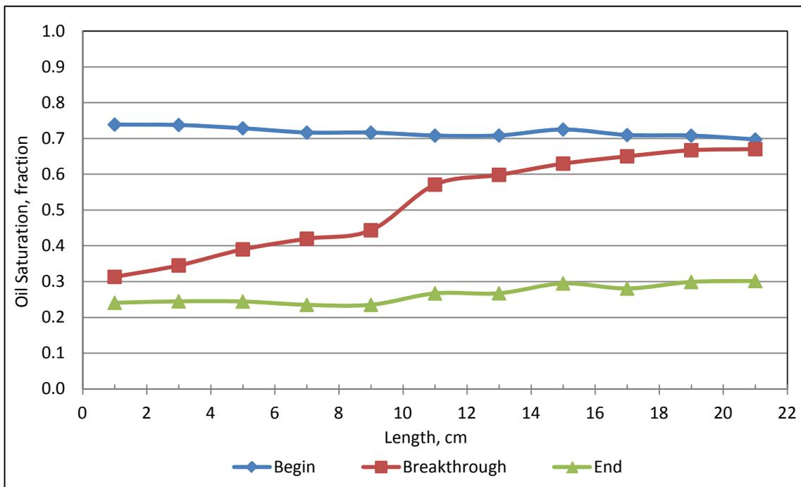
Figure 4.27: Oil saturation profiles during waterflooding for A8-100
