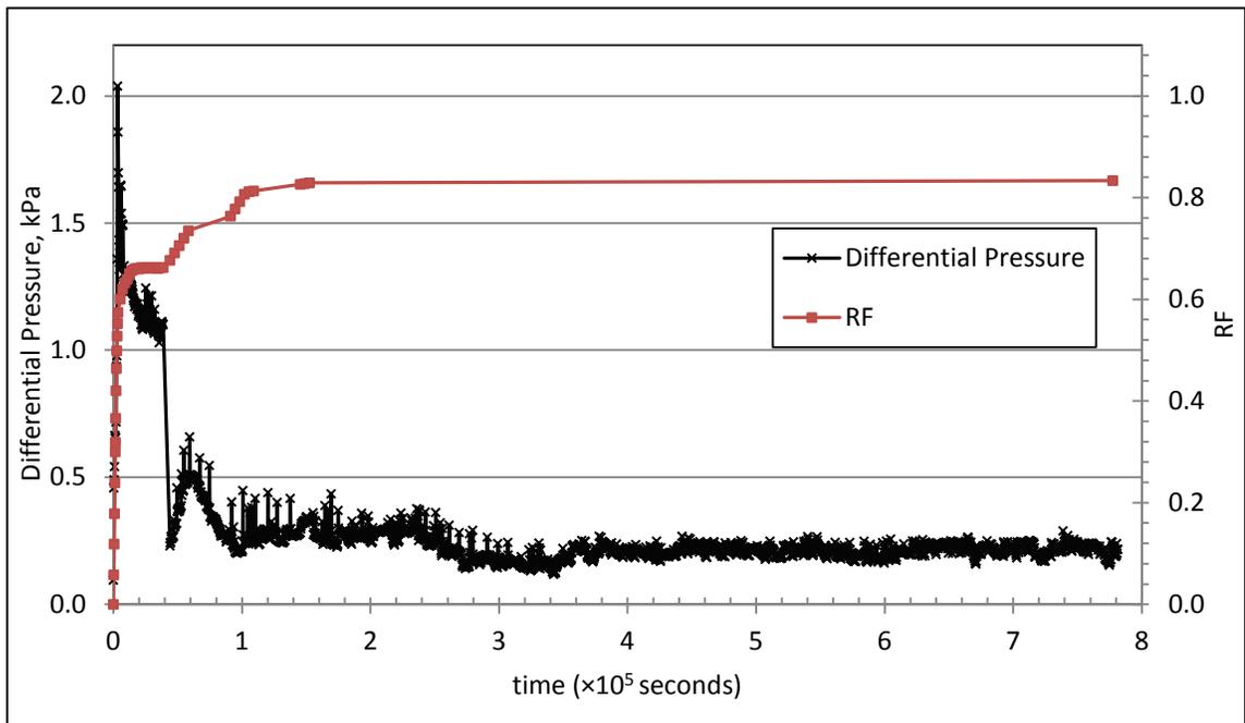
**Figure 4.48: Comparison of oil production and differential pressure (A5-500)**
