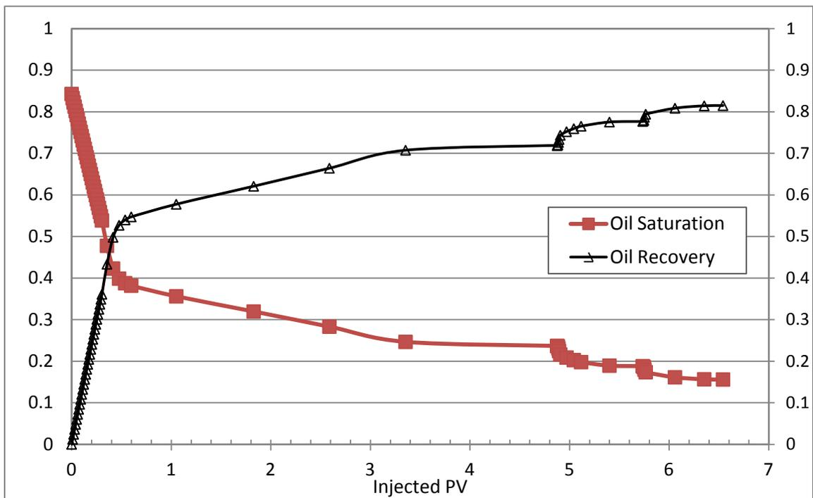
Figure 4.11: Recovery vs. PVs of water injected for A5-100-10
