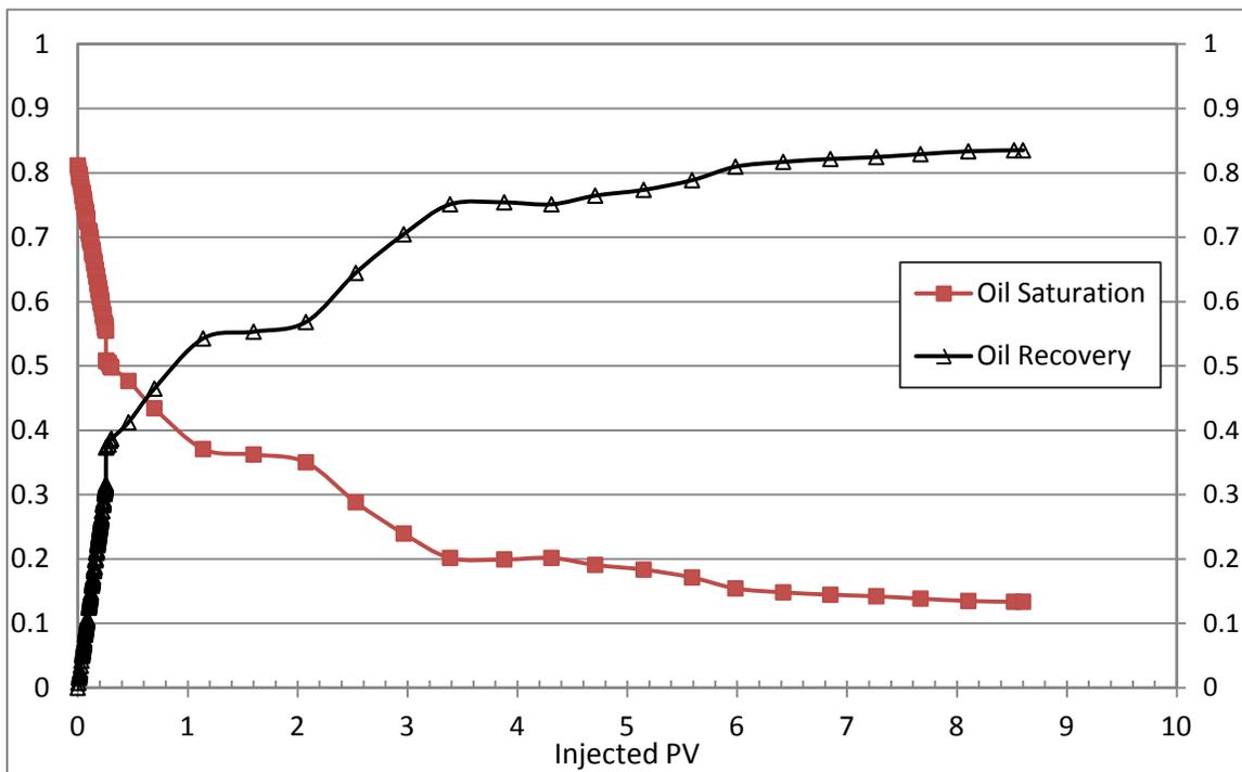
**Figure 4.2: Recovery vs. PVs of water injected for A5-10**
