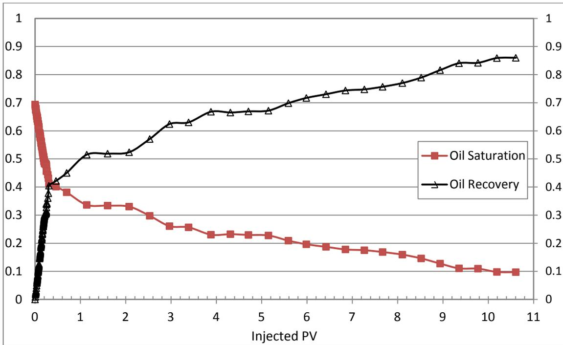
Figure 4.22: Recovery vs. PVs of water injected for A8-10
