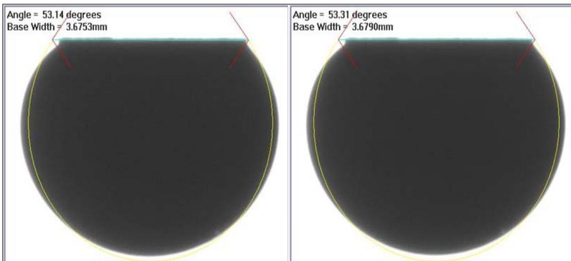
**Figure I.1: Oil drop images for contact angle measurement**
