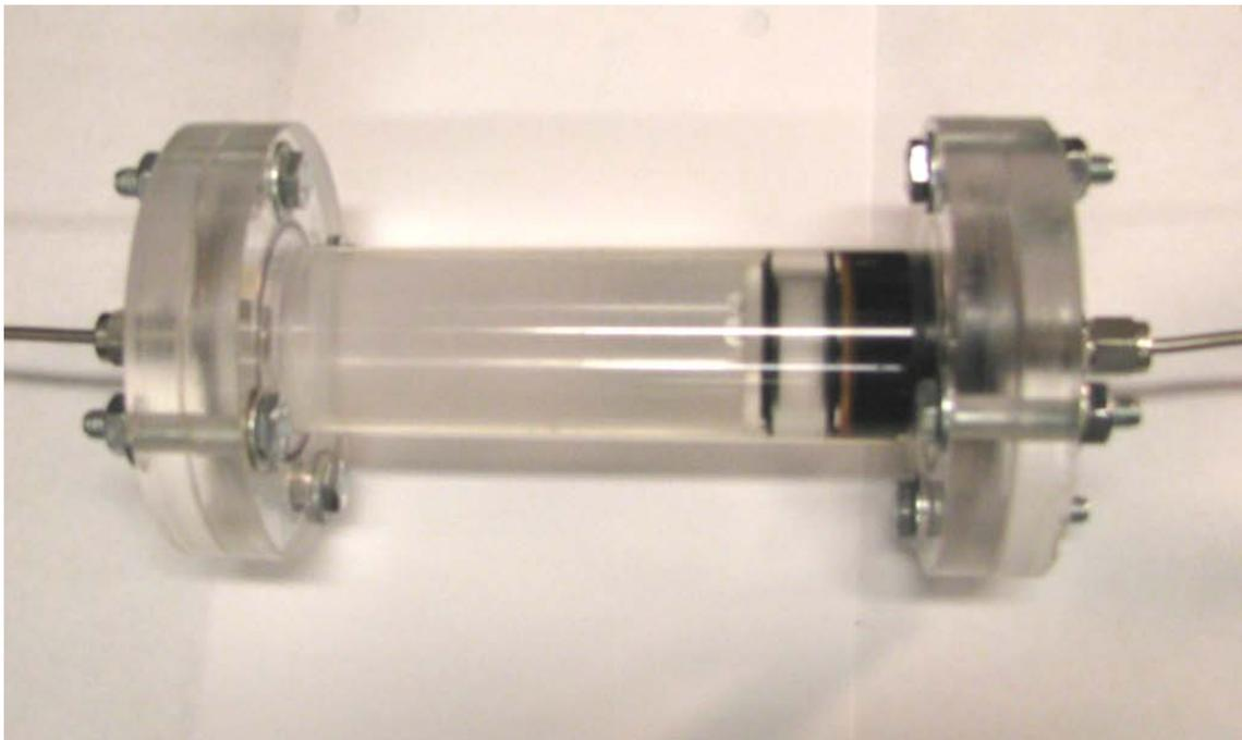
**Figure 3.7: Small volume piston cylinder**
