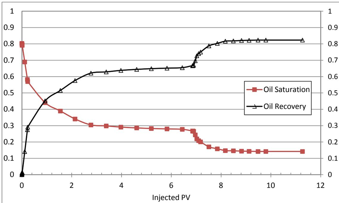
Figure 4.18: Recovery vs. PVs of water injected for A5-1000-10
