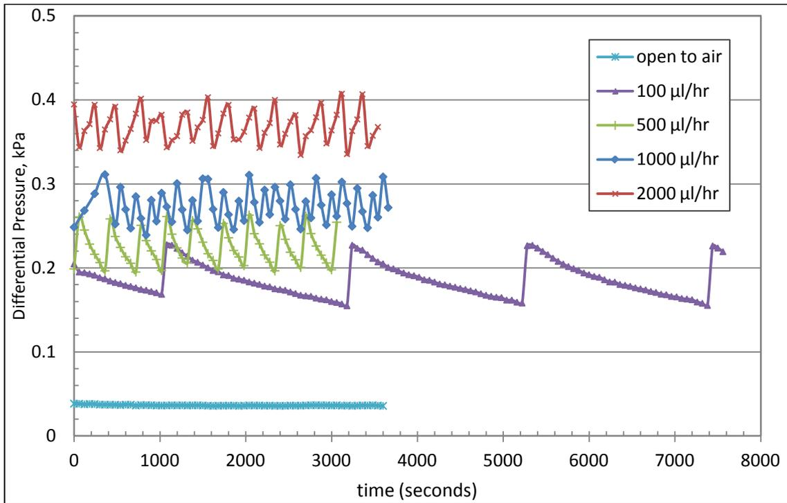
**Figure III.2: Differential pressure curves of water drop experiment**
