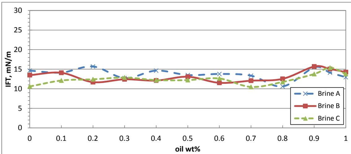
**Figure 3.1: IFT of oil – water system using spinning drop method**
