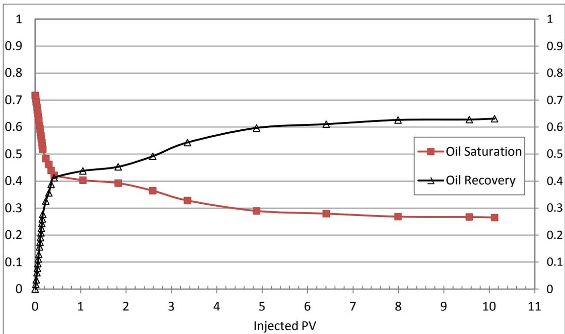
**Figure 4.26: Recovery vs. PVs of water injected for A8-100**
