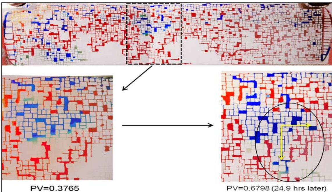
**Figure 4.42: Direction of imbibition after water breakthrough for A8-10**
