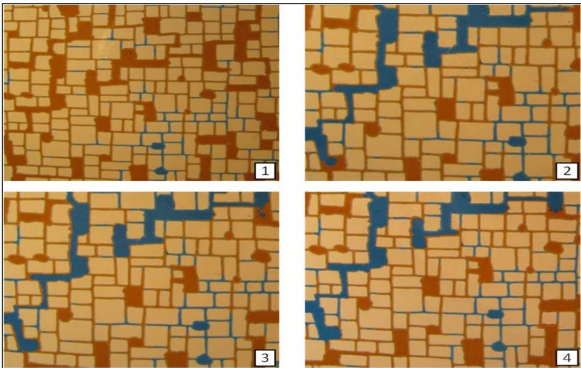
**Figure 4.45: Schematic of viscous instability (A5-1000)**
