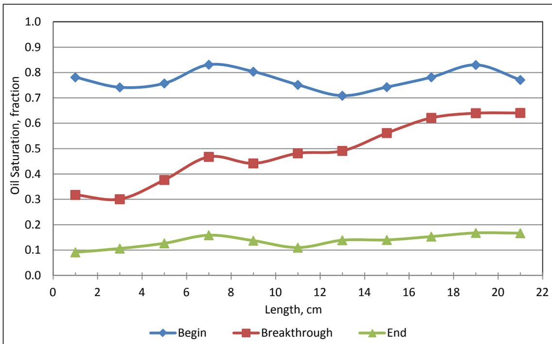
Figure 4.8: Oil saturation profiles during waterflooding for A5-100
