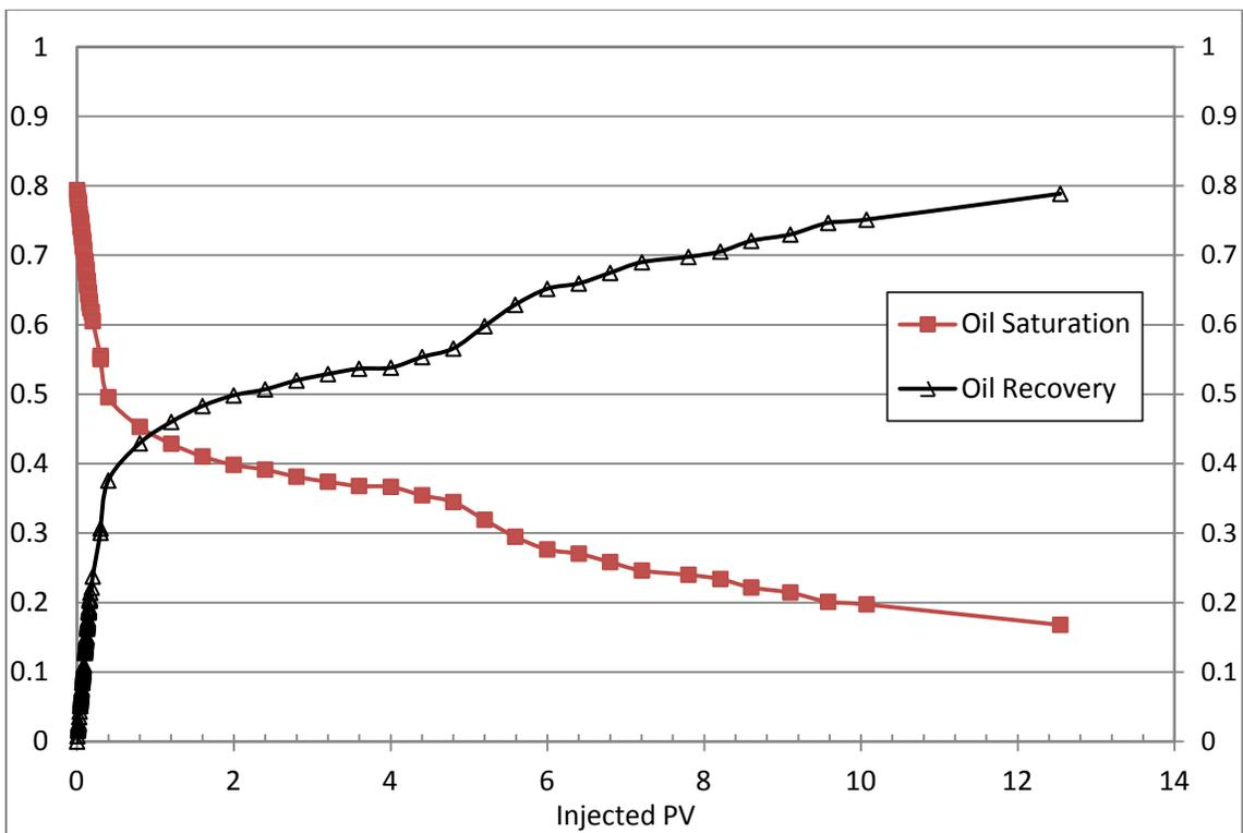
Figure 4.30: Recovery vs. PVs of water injected for A10-10
