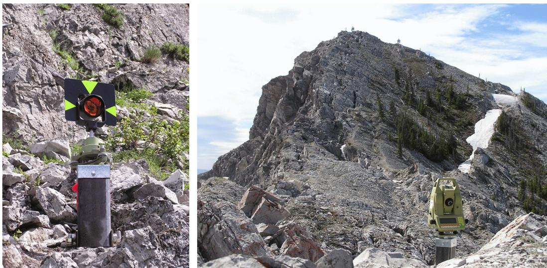
Figure 5.4: Prism on monitoring pillar (left) and LEICA TCA 2003 pointing at South Peak (right)
