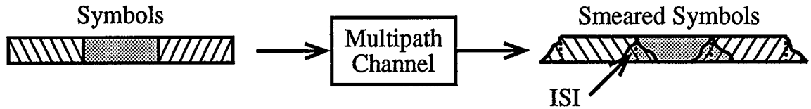
Figure 2.5 ISI of multiple symbols passing through a multipath channel.
