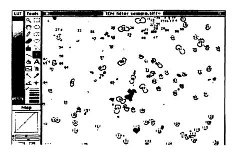
Figure 11-- Result of Analyze Particles command. Pores are outlined and numbered.
