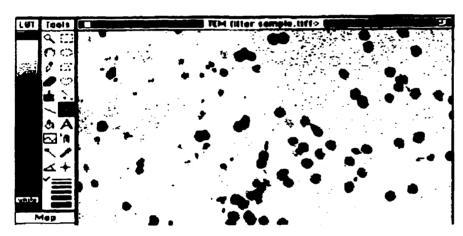
Figure 9-- Filter image with pores selected using thresholding (see text).
