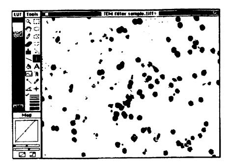
Figure 10-- Pores in smoothed TEM Filter image selected by thresholding.
