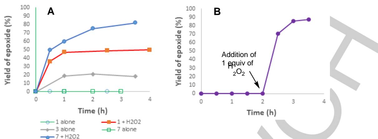
**Figure 4.** A) Yields of cyclooctene epoxide were obtained by GC analysis with an internal standard. Reactions were performed in dichloromethane with equimolar amounts of cyclooctene, the selenium compound and, where indicated, hydrogen peroxide. B) Epoxidation was conducted similarly with selenonic acid **4** alone, followed by addition of one equiv of hydrogen peroxide after 2 h. Rate constants are provided in the Supporting Information.
