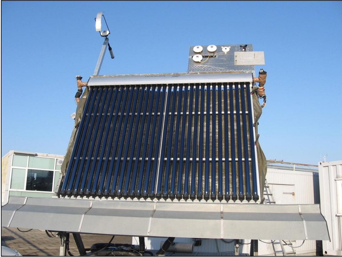
Figure 2.4: Instrumentation of HP ETC TZ58-1800-30R on Test Day ((Jiangsu Sunrain Solar Energy, n.d.)
