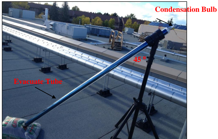
Figure 3.14: Experimental Setup to Determine Heat Capacity of Evacuated Tube. Photographed by Athaudage Dona, (2013)
