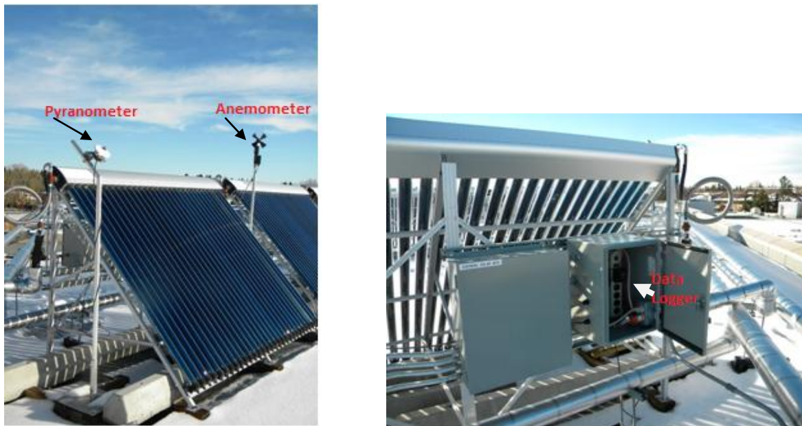
Figure 3.6: a) Front View West Side Collector (Left) b) Back View of West Side Collector(Right). Photographed by Athaudage Dona ,(2012).
