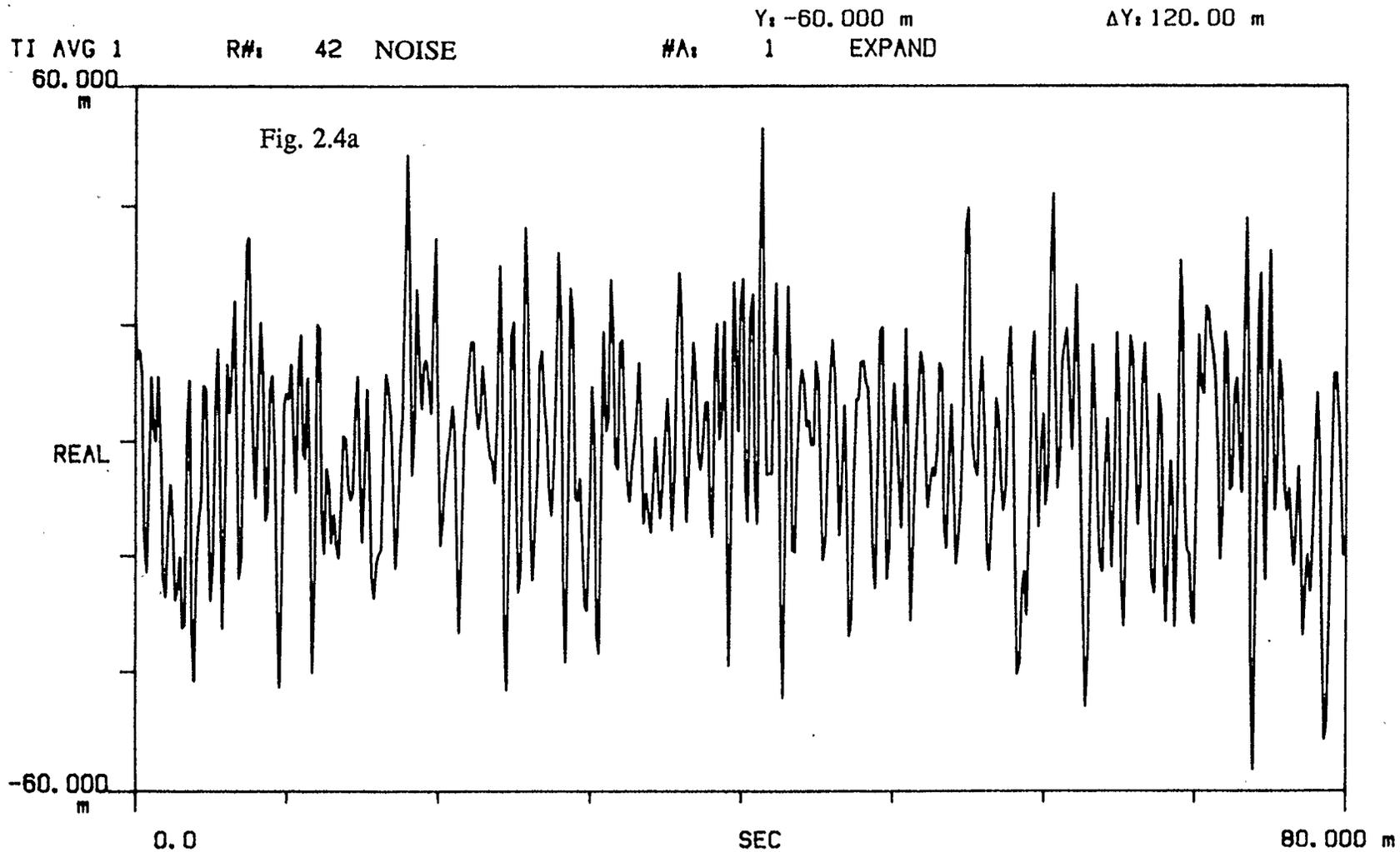
Fig. 2.4 A simulation of an optimal filter for a first order Butterworth signal  $n = 1$ , with a  $SNR = d = 10$ , and an  $ESR = \sigma_e / \sigma_s = 0.4254$ . (a) The noise  $n(t)$ . (b) The input signal  $s(t)$ , and the filter output  $y(t)$ .
