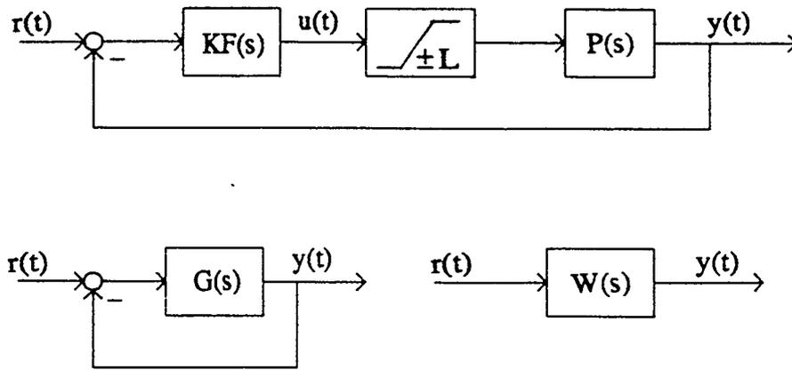
Fig. 3.1 The realistic series compensation problem considered.  $P(s)$  has  $PZE \geq 3$ , and saturation constraint nonlinearity ( $\pm L$ ) at its input.
