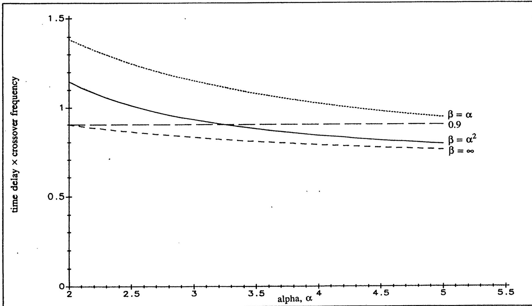
Fig. 3.8 MACSYMA results for time delay as a function of alpha for  $2 \leq \alpha \leq 5$ .
