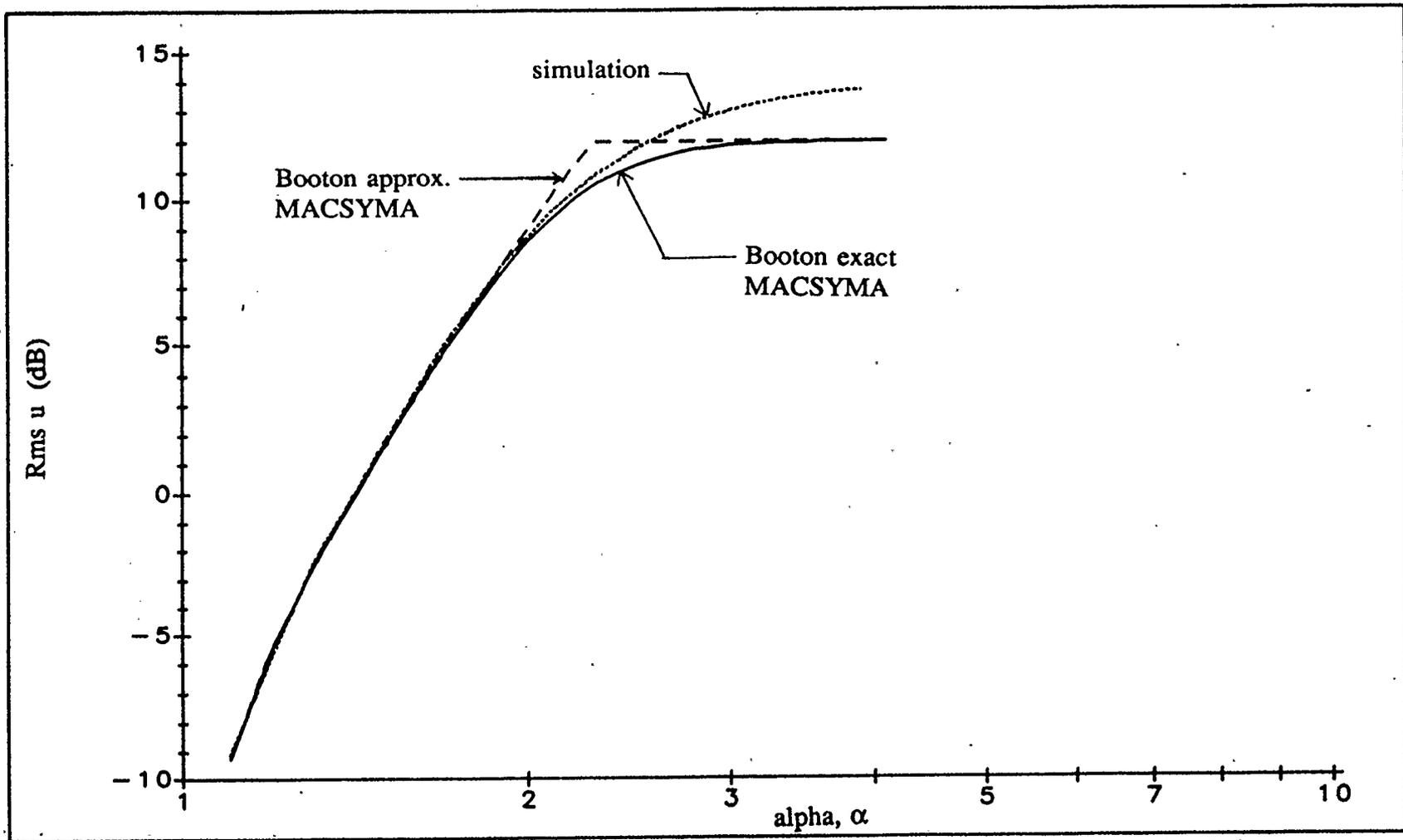
Fig. 4.5 Rms control effort of the LQ regulator with the saturation nonlinearity for a stochastic input.
