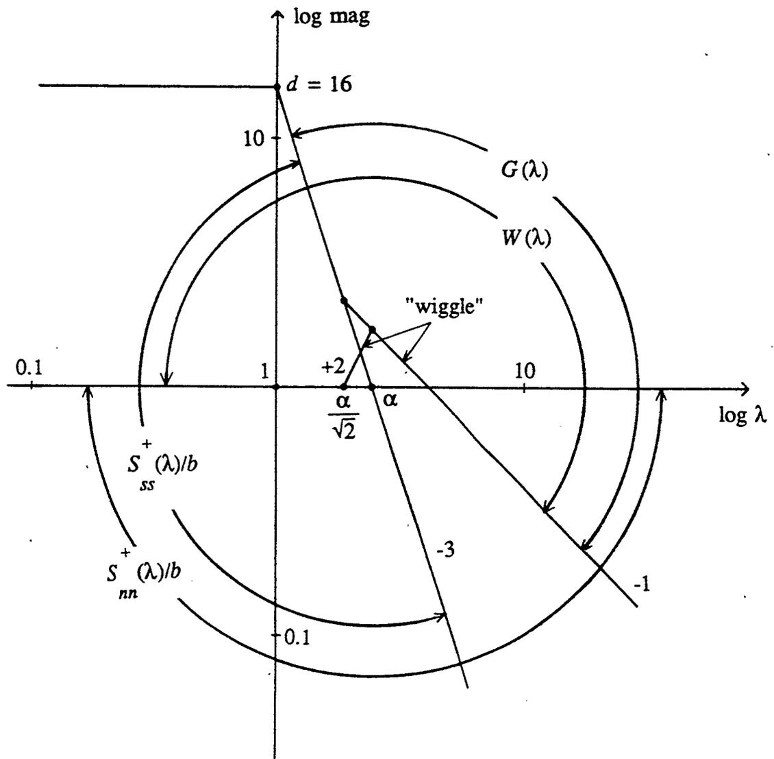
Fig. 2.2 Bode plots for an optimal filter, with  $n = 3$  and  $d = 16$ . The factored given data are normalized by the white noise  $b$ , and the optimal filters are  $W(\lambda)$  and  $G(\lambda)$ . Notice the simple graphical relationship between the given data and the optimal filters  $W(\lambda)$  and  $G(\lambda)$ .
