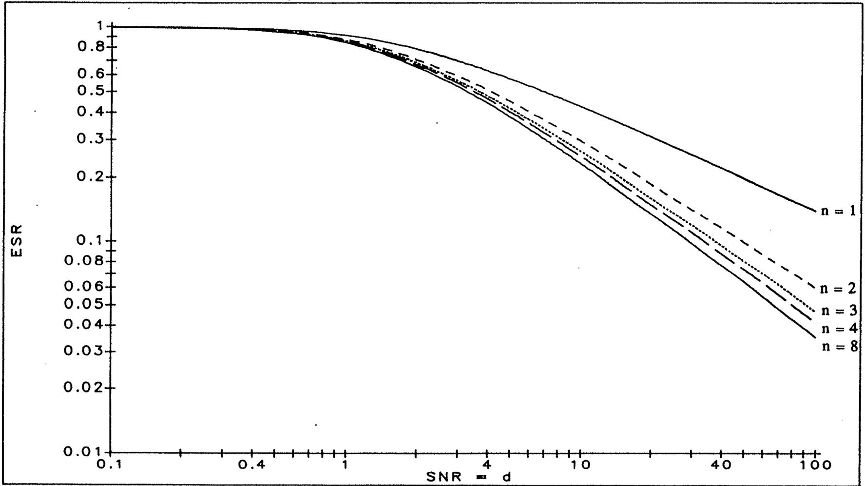
Fig. 2.3 The optimal filters performance. ESR versus SNR for  $n = 1, 2, 3, 4,$  and  $8.$
