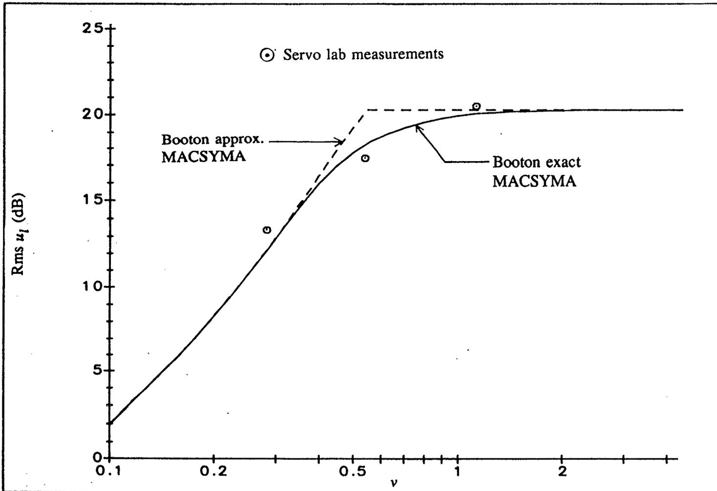
Fig. 3.17 Continuation of Fig. 3.16. Rms value of the limited input to the fixed plant  $\sigma_u$  versus normalized frequency  $\nu$ .
