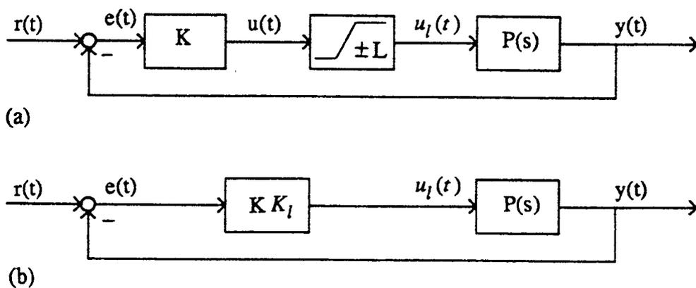
Fig. 3.14 Booton's analysis for a control system with a random input. (a) Actual nonlinear system. (b) Linearized model.
