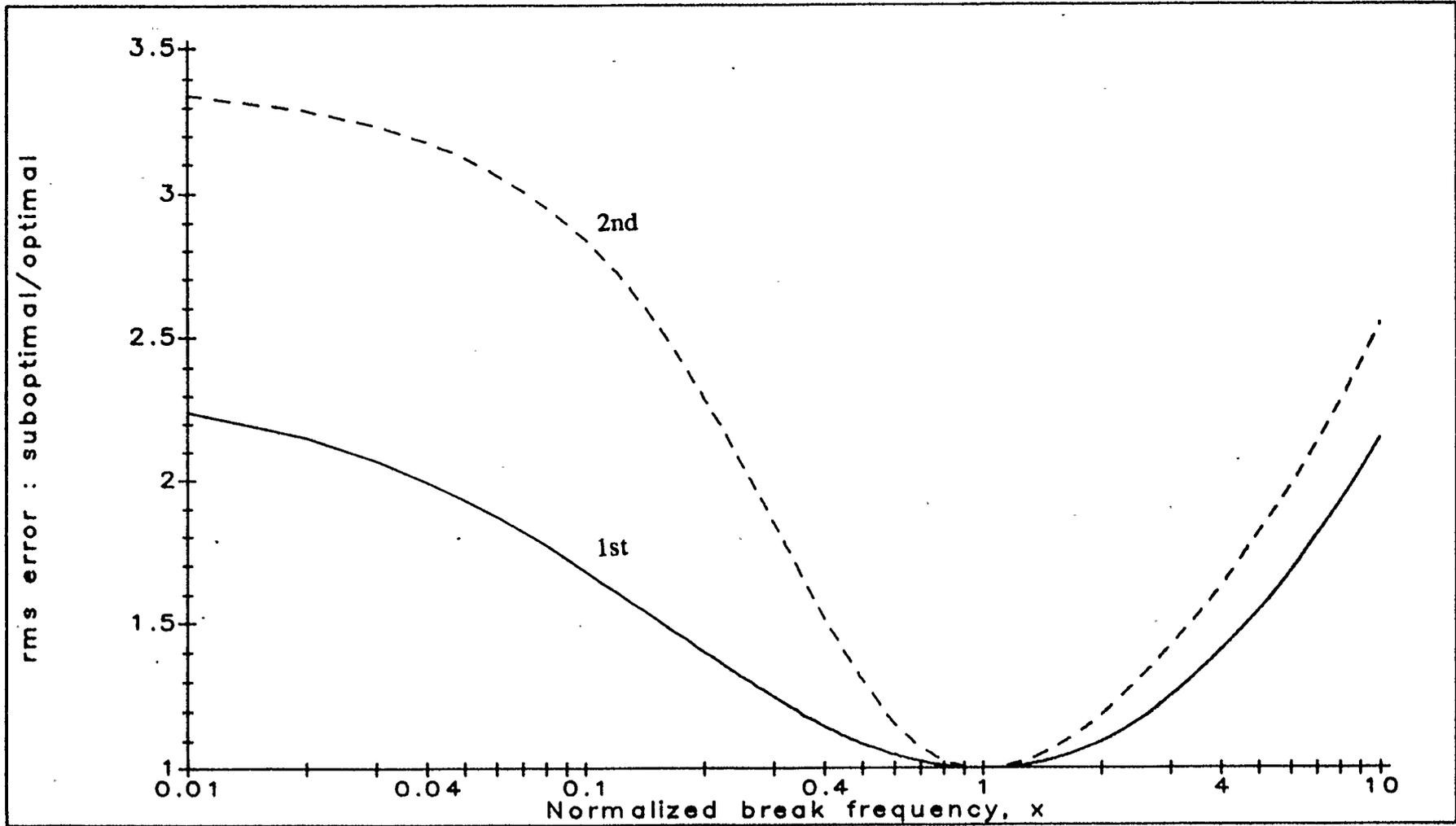
Fig. 2.9 Increase in rms error for the suboptimal filter  $G_2(\lambda)$ .
