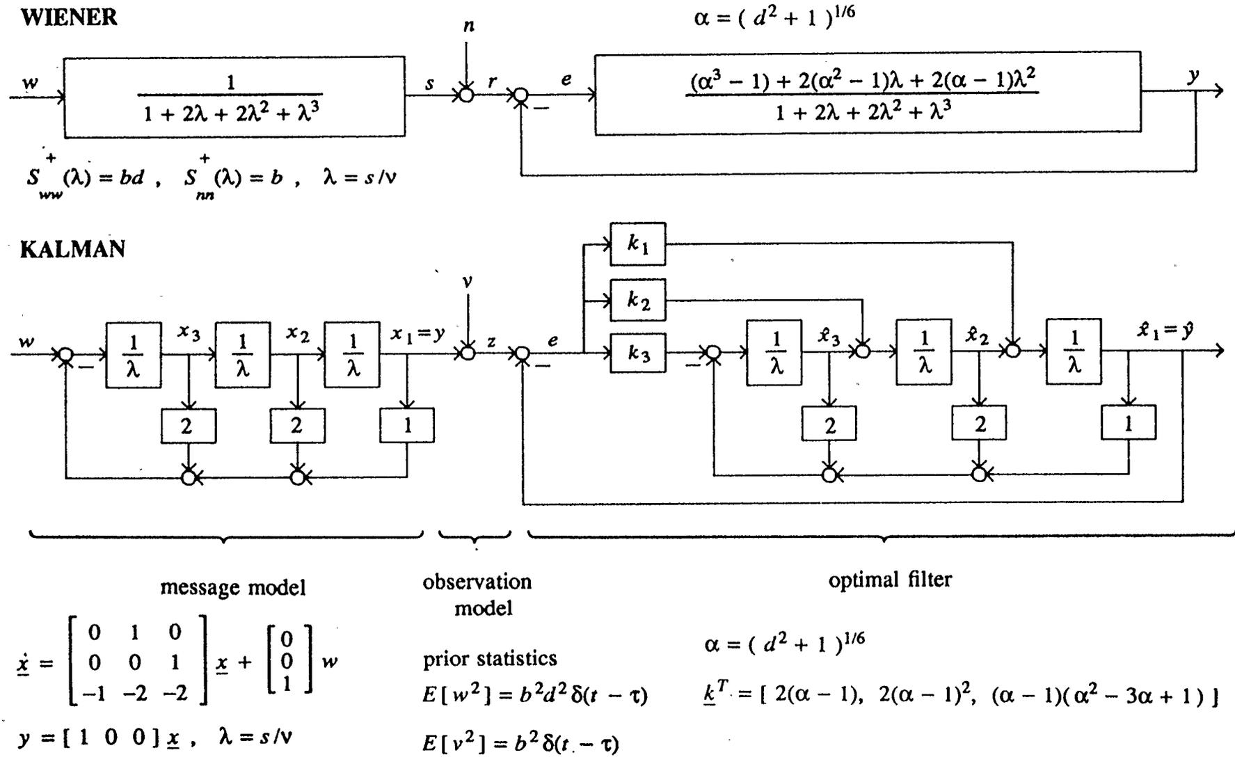
Fig. 2.6 Comparison of Wiener and Kalman filters, for third order Butterworth signals (n=3), in terms of normalized frequency  $\lambda$  ( $\lambda = s/v$ ).
