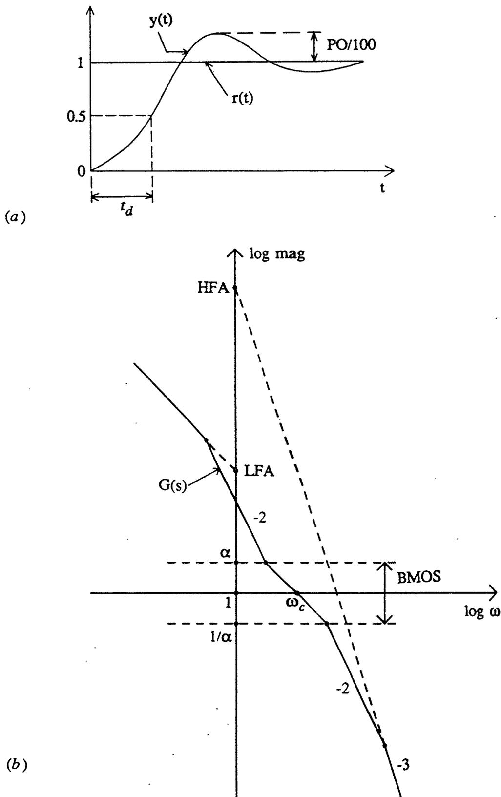
Fig. 3.3 (a) Basic specifications (specs). Time domain specs. PO = percent overshoot, a quality of response spec.  $t_d$  = time delay, a speed of response spec. (b) Frequency domain specs. LFA = low frequency asymptote;  $\omega_c$  = crossover frequency; BMOS = the horizontal symmetrical ( $\alpha$ ,  $1/\alpha$ ) band of a -1 slope at mag. = 1; and HFA = high frequency asymptote.
