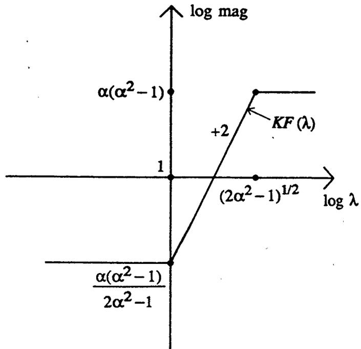
Fig. 4.6 Bode plot of the series compensation  $KF(\lambda)$ , considering the saturation nonlinearity and which uses the ABPR.
