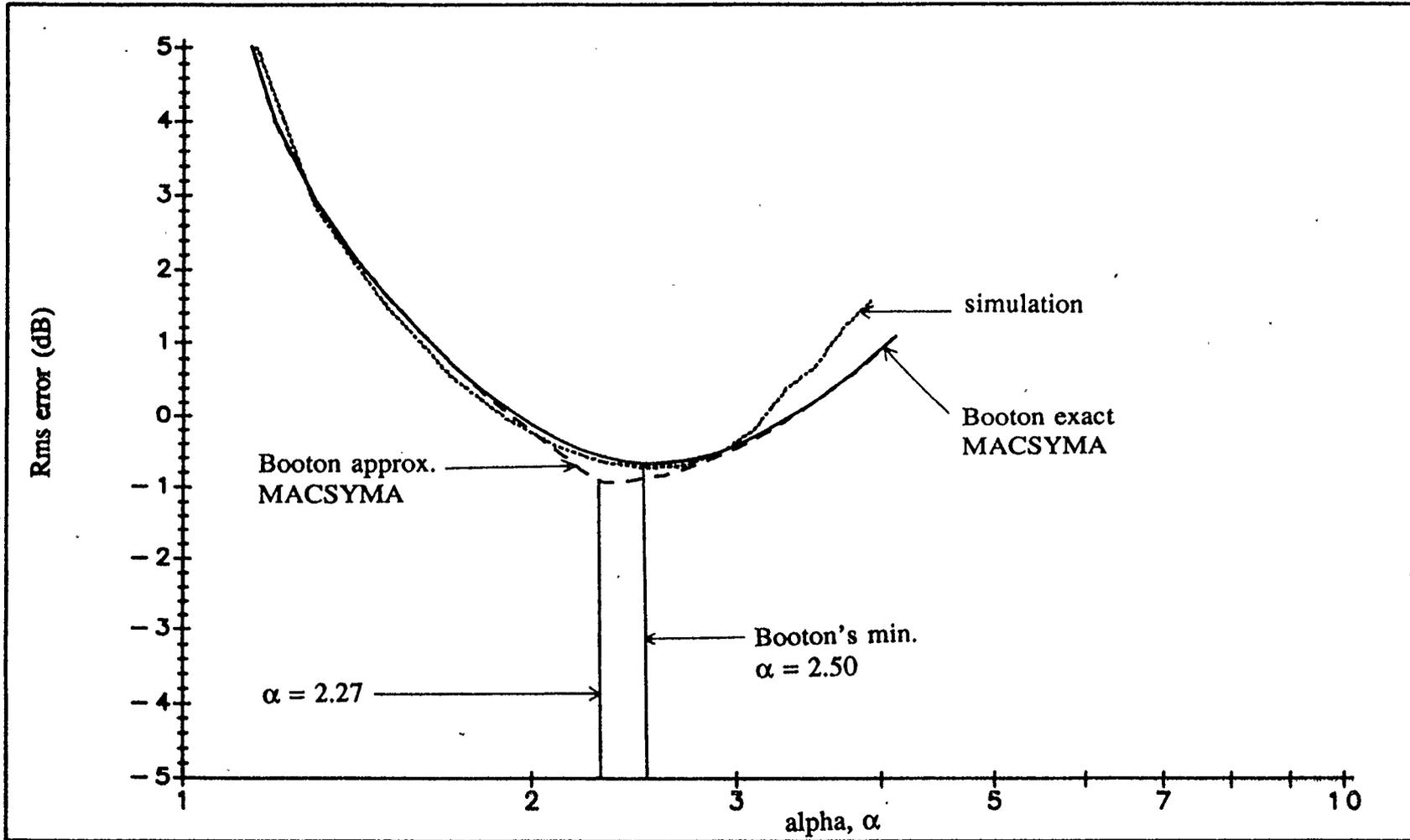
Fig. 4.4 Rms error of the LQ regulator with the saturation nonlinearity for a stochastic input.
