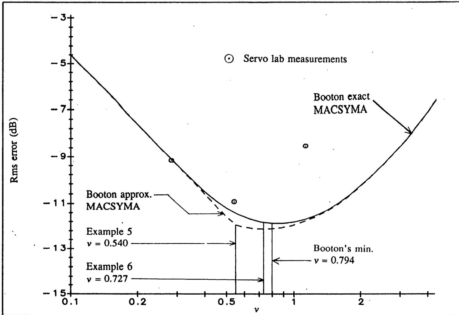
Fig. 3.16 Simulation results for Examples 5 and 6. Rms error versus the normalized frequency  $\nu$  where  $c = \nu\omega$ .
