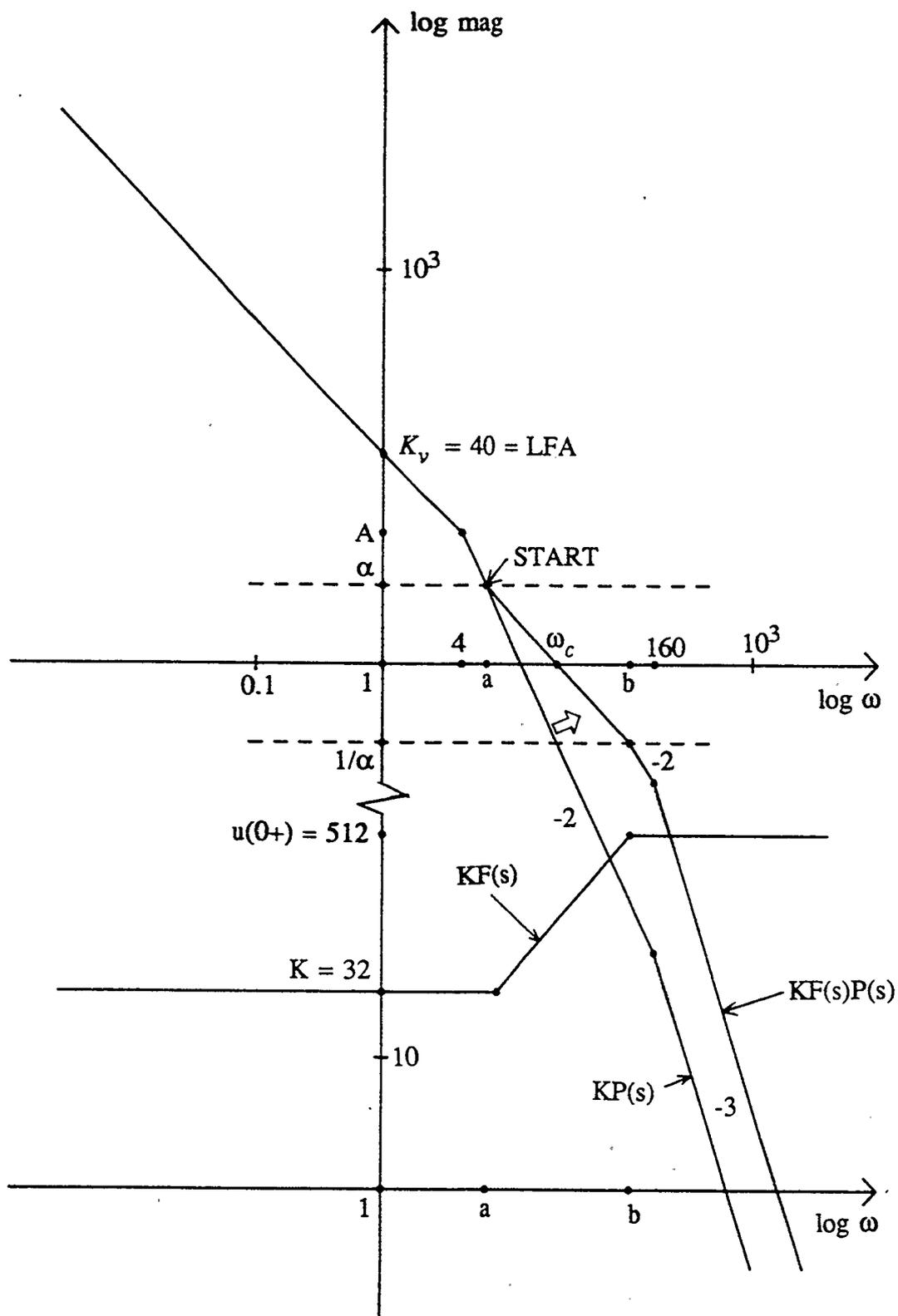
Fig. 3.11 Example 2, design procedure for a lead network.
