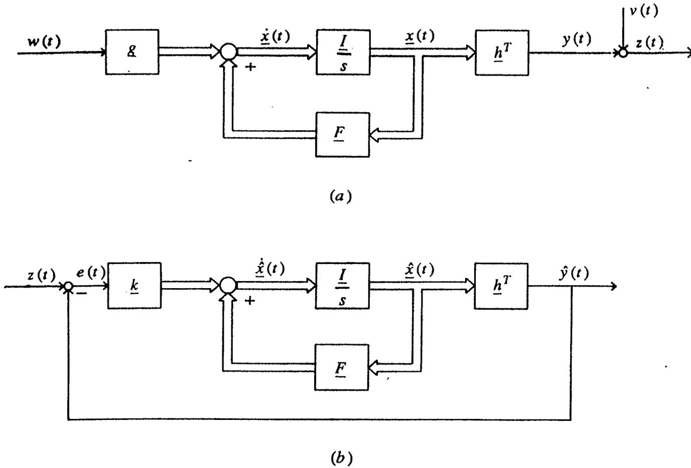
Fig. 2.5 The Kalman filter problem. (a) The message and observation model. (b) The optimal filter.
