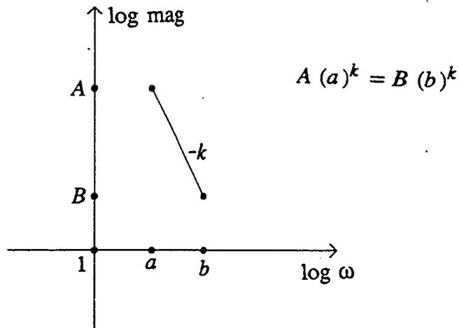
Fig. 3.2 The algebraic Bode plot relationship (ABPR) between any two points  $(a, A)$  and  $(b, B)$  which are connected by a slope of  $-k$ .
