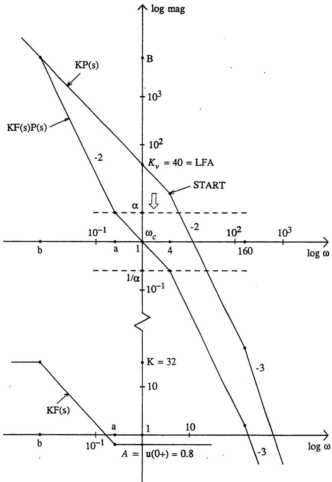
Fig. 3.9 Example 1, design procedure for a lag network.
