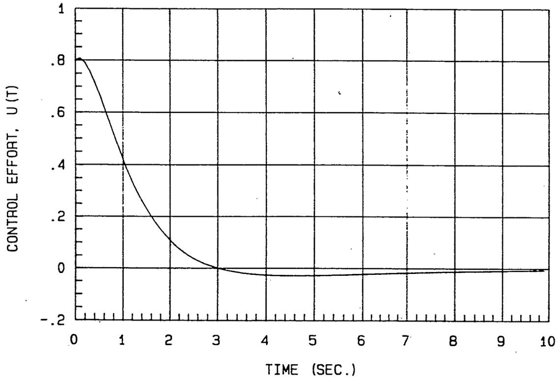
Fig. 3.10. Example 1, computer simulation of step response and control effort.
