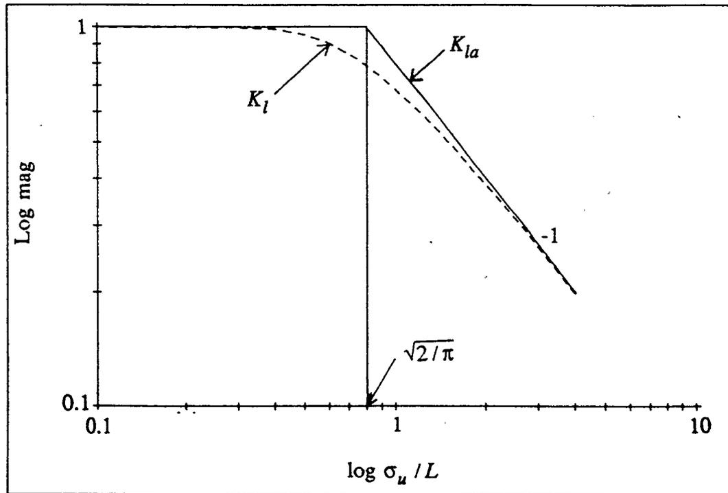
Fig. 3.15 Booton's equivalent gain  $K_l$ , and an approximation to it  $K_{la}$ .
