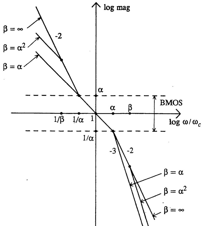
Fig. 3.6 The compensated systems which are used to relate time domain specs on  $y(t)$ , to frequency domain specs on  $G(s)$ .
