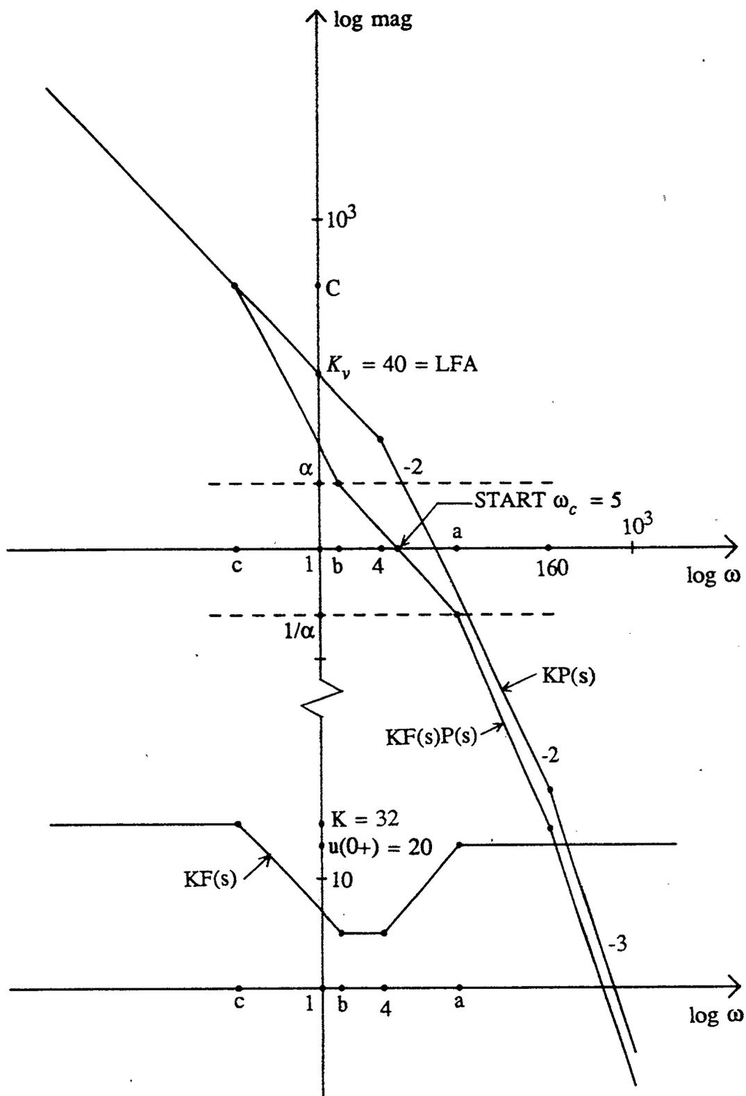
Fig. 3.12 Example 3, design procedure for a lag-lead network.
