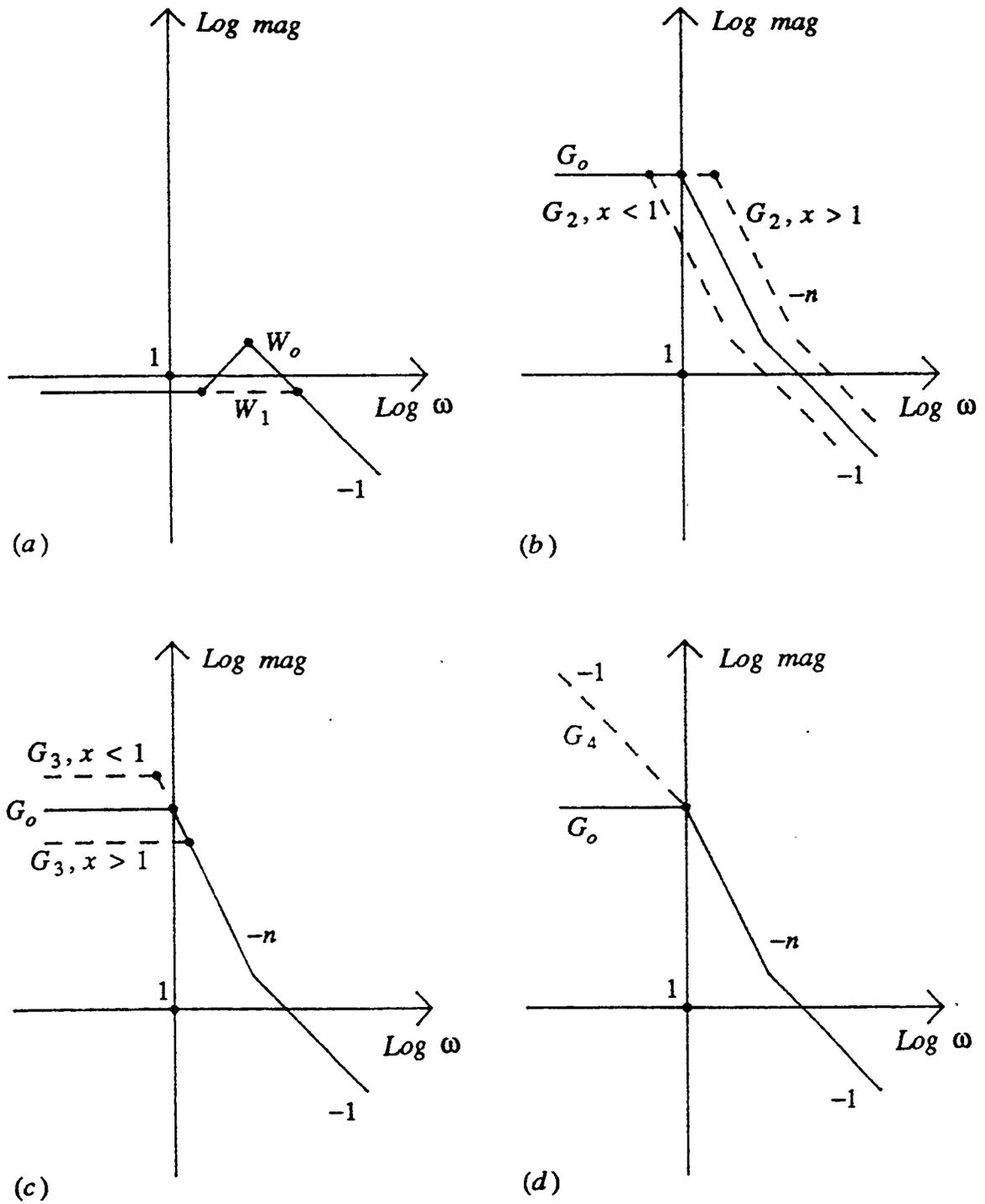
Fig. 2.7 Bode plots for suboptimal filters. (a) Suboptimal filter  $W_1$ . (b) Suboptimal open-loop filter  $G_2$ . (c) Suboptimal open-loop filter  $G_3$ . (d) Suboptimal open-loop filter  $G_4$ .
