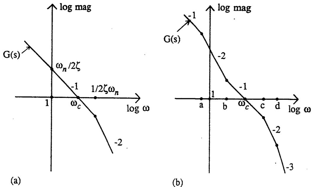
Fig. 3.4 Systems used to relate time domain specs on  $y(t)$  to frequency domain specs on  $G(s)$ . (a) Traditional. (b) This Chapter.
