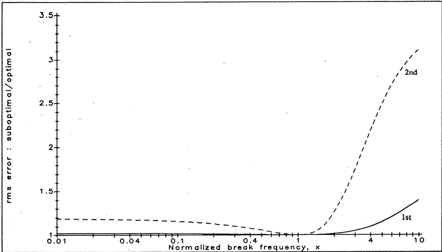
Fig. 2.10 Increase in rms error for the suboptimal filter  $G_3(\lambda)$ .
