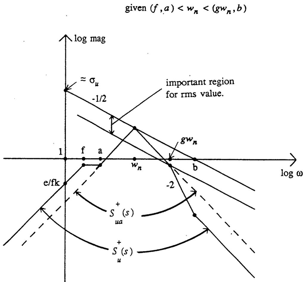
Fig. 3.18 Example 6, design procedure for the approximate evaluation of the mean-square value,  $\sigma_u^2$ .
