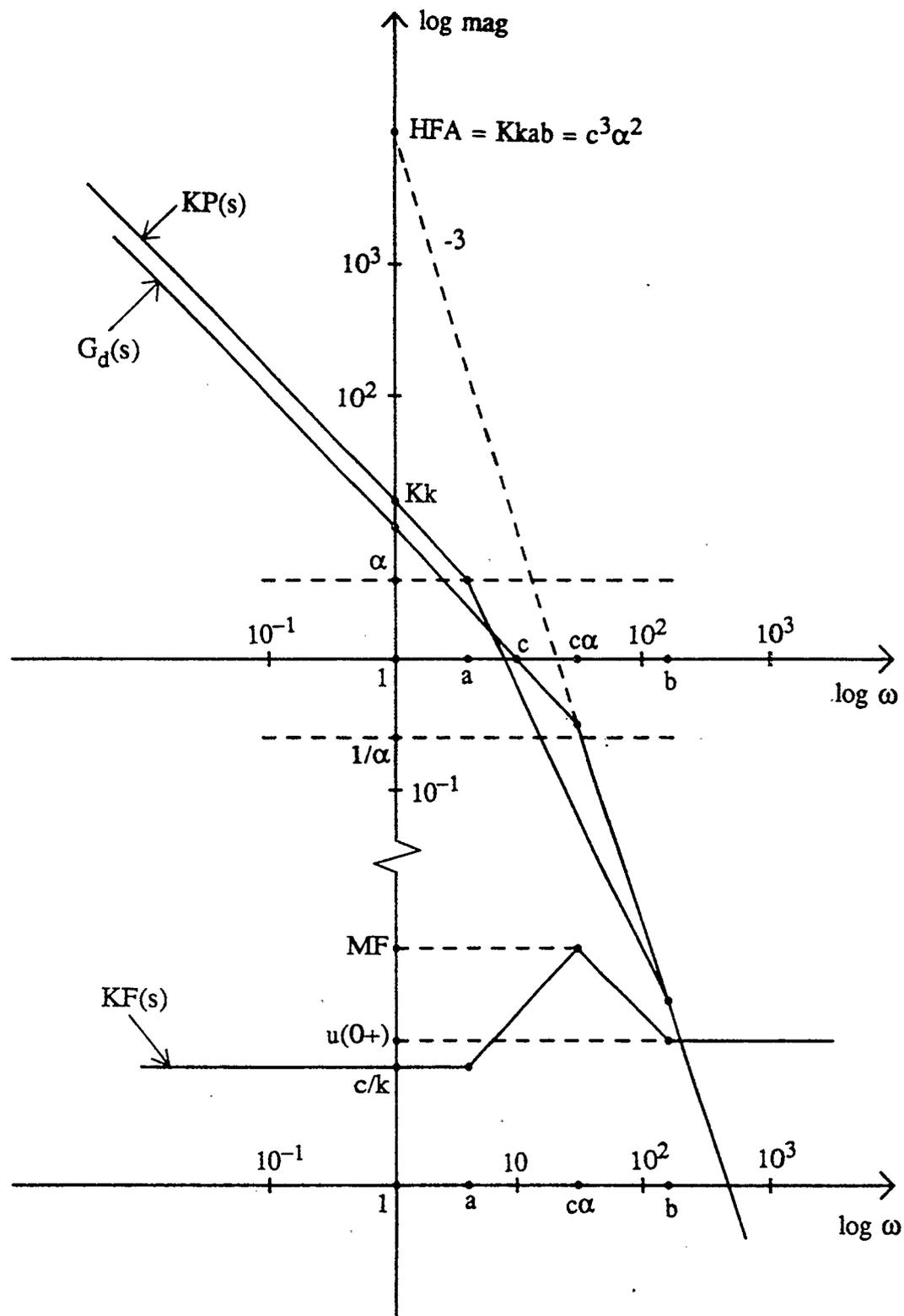
Fig. 3.13 Example 4, design procedure for a saturation constraint for a unit step.
