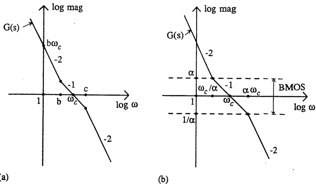
Fig. 3.5 The maximize phase margin problem. (a) The problem. (b) The solution.
